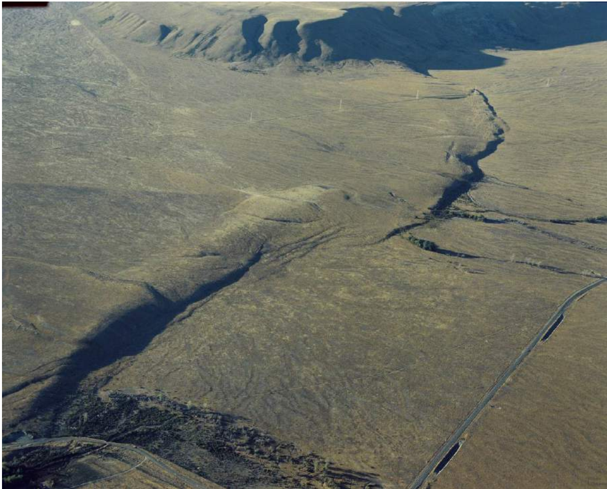
Figure 1.3 A northward oblique aerial view of the Ostler Fault Zone, about 12 km southwest of Twizel. The fault zone runs from lower left to upper right, and has offset and buckled a ~22,000 year old glacial meltwater outwash plain, with well-preserved relict braided channels, that was sourced from the Lake Ohau area. Lake Ohau Road is at lower left, and State Highway 8 is in lower right. At the lower left, the fault scarp (in shadow) is sharply defined. Heading towards the photo centre, the fault scarp evolves into a broad fold which peters out near the photo centre. At that point, another fault strand and associated fold has emerged 200 m or so in front of it (right) and, in somewhat serrated form, curves broadly to the left towards the shadow of a high uplifted terrace (Table Hill), and then curves along the foot of the hill (in shadow) to the upper right corner. Right of centre and right of the fault scarp, the three darker lines are the channels of spring-fed streams that emanate from the foot of the fault scarp. This view shows an array of 'definite' faults and folds which all form part of a single entity, the Ostler Fault Zone. In the generalised dataset accompanying this report, the Ostler Fault Zone at this location is represented by a single mapped fault line, and the folds and numerous small subsidiary fault strands are not differentiated in this regional-scale dataset. In contrast to the strike-slip faults shown in Figure 1.2 , the Ostler Fault Zone is a dip-slip fault with a reverse sense of movement (see Figure 3.1 for diagrammatic representations of these two different styles of fault movement). Photo: D.L. Homer, GNS Science CN576/B; taken 1995.
