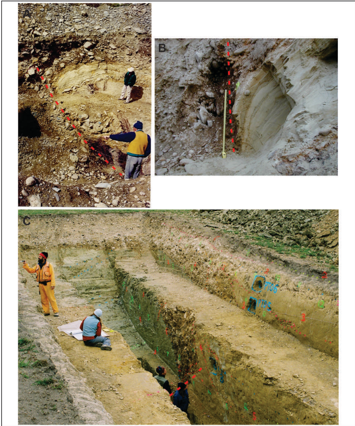
Figure 3.2 Illustrations of faults exposed in investigation trenches. Dashed red lines indicate the position of the fault in each photo. A & B: The Waitangi Fault (feature 12f – see Appendix 2) exposed in 1999 in a trench 700 m downstream of Aviemore Dam. A: the fault runs upper left to lower right and a bed of yellow sand has been pushed up and buckled over against river gravel to the left. B: detail of the fault contact after further excavation and cleaning. The yellow tape measure (extended 1 m) provides scale. Layering in the sand has been dragged down nearly vertical against the fault, while elongate river stones immediately left of the sand bed have been dragged up into vertical alignments. C: A trench excavated across the Kirkliston Fault Zone (feature 13 - see Appendix 2) in 2007, 14 km northeast of Kurow. The fault contact is beside the two people deep in the trench. Greenish-grey claystone overlain by yellow-brown stream gravel (left of centre) has been thrust up and buckled over against yellow-brown silt (loess) to the right. Detailed examination and mapping of the materials showed evidence for at least two separate rupture events. The blue-painted squares mark samples that were collected for luminescence dating to obtain age control on the rupture events. The dating showed that the most recent rupture most likely occurred between 12,900 and 22,000 years ago, and the recurrence interval for surface rupture is between 23,000 and 39,000 years. Photos A & B: D.J.A. Barrell; Photo C: S.A.L. Read.
