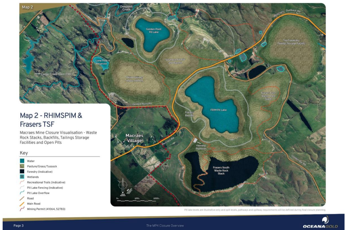
Figure 3.14: Golden Point Pit, SP11 TSF, Innes Mills Pit and FTSF at closure.
