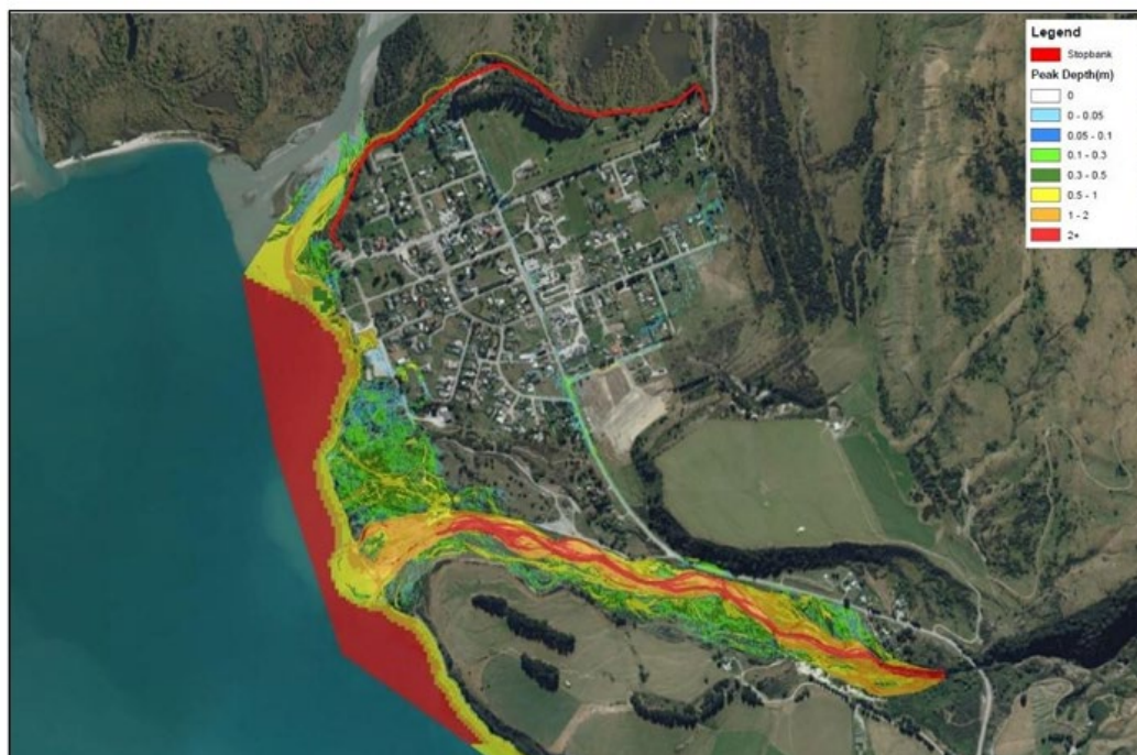
Figure 9.8 Model results showing floodwater depths for a Buckler Burn flooding scenario with a 300 m 3 /s peak flow. In this scenario minor floodwaters flow into the township area, mainly flowing northwards along Oban Street and around the eastern margin of the township.
