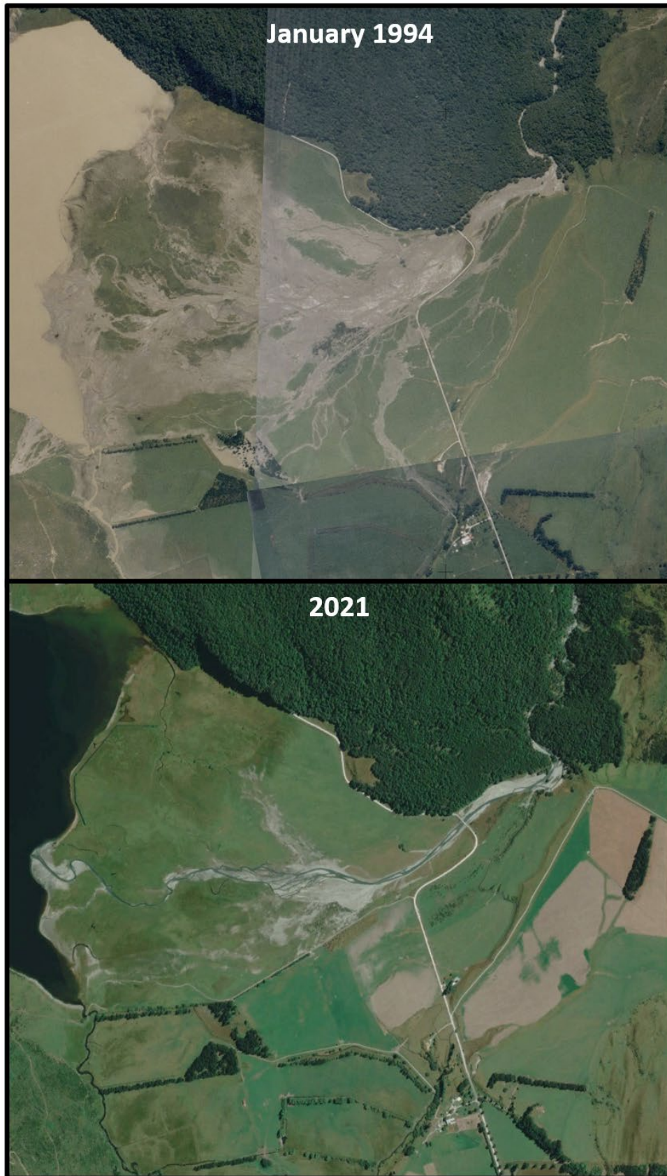
Figure 5.10 Comparison of the Earnslaw Burn alluvial fan in flood (1994) and non-flood conditions (2021), illustrating the potential for widespread flooding and debris impacts across alluvial fan surfaces.
