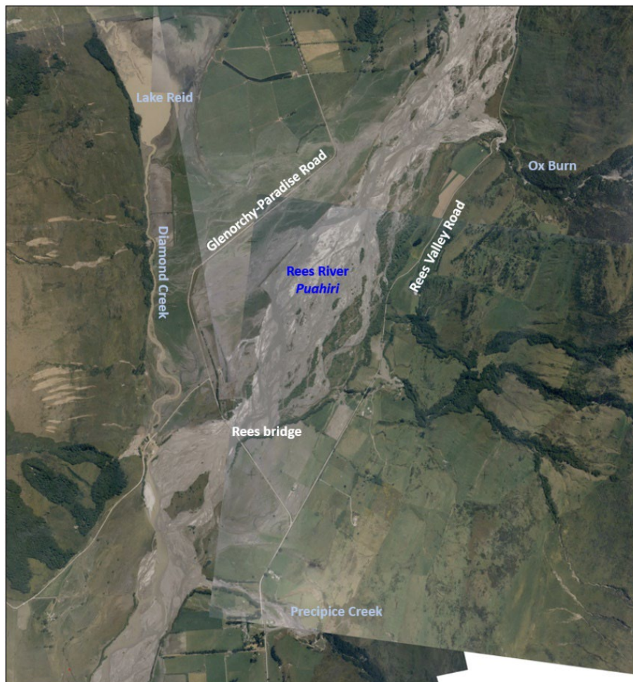
Figure 5.19 January 1994 - disruption to road access and damage to infrastructure and land, caused by flooding of Rees floodplain, and alluvial fan activity at the Precipice Creek and Ox Burn alluvial fans.
