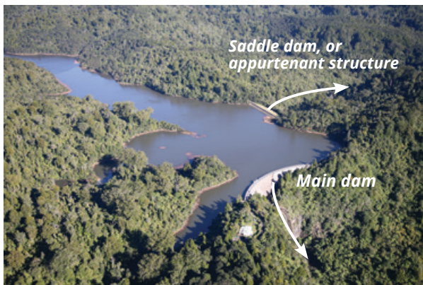
Figure 4.1: example of main and subsidiary dams with different features and dam-break flow paths (provided by Watercare Services).
