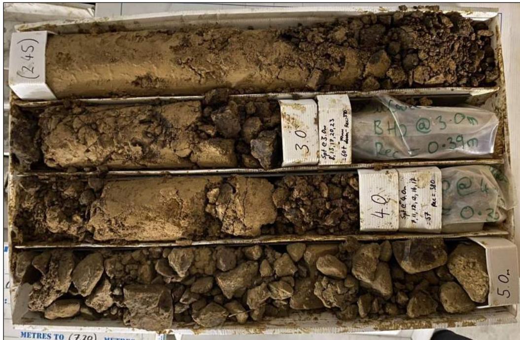
Photo BH10.2 BH10 Box 2: 2.5m to 5.0m
