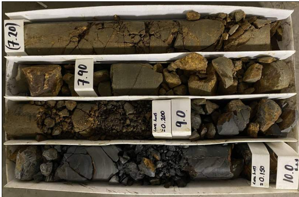
Photo BH10.4 BH10 Box 4: 7.2m to 10.0m
