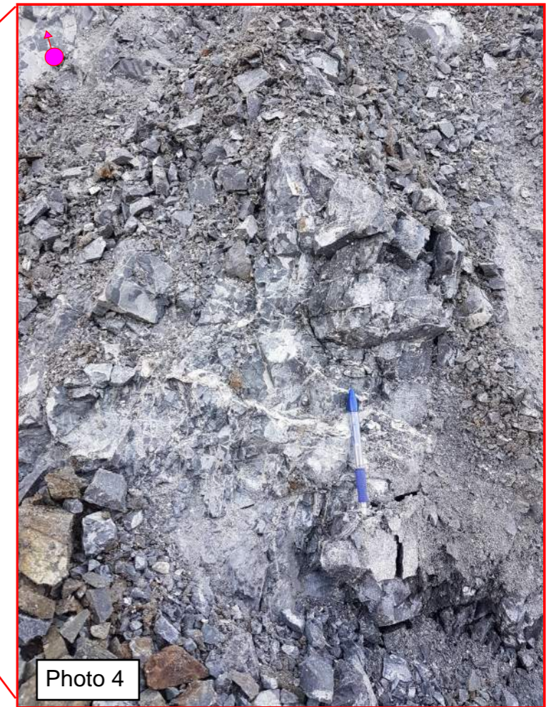
Photo 4 (above): Cataclasite shear zone observed, approximate dip angle is 45 to the west
