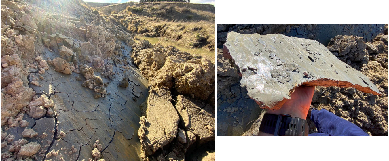
Photo 1: Example of the FF surface condition as exposed in the upper Frasers West headscarp. The sliding surface is described as slickensided and undulous, comprising high plasticity moist firm clay. Note: The exposed orientation does not reflect the regional geometry due to interactions with the Macraes Fault Zone.
