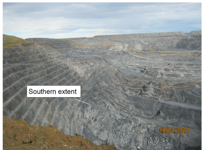
Inset 3: Approximate extents of the April 2014 20 Mm 3 west wall failure.
