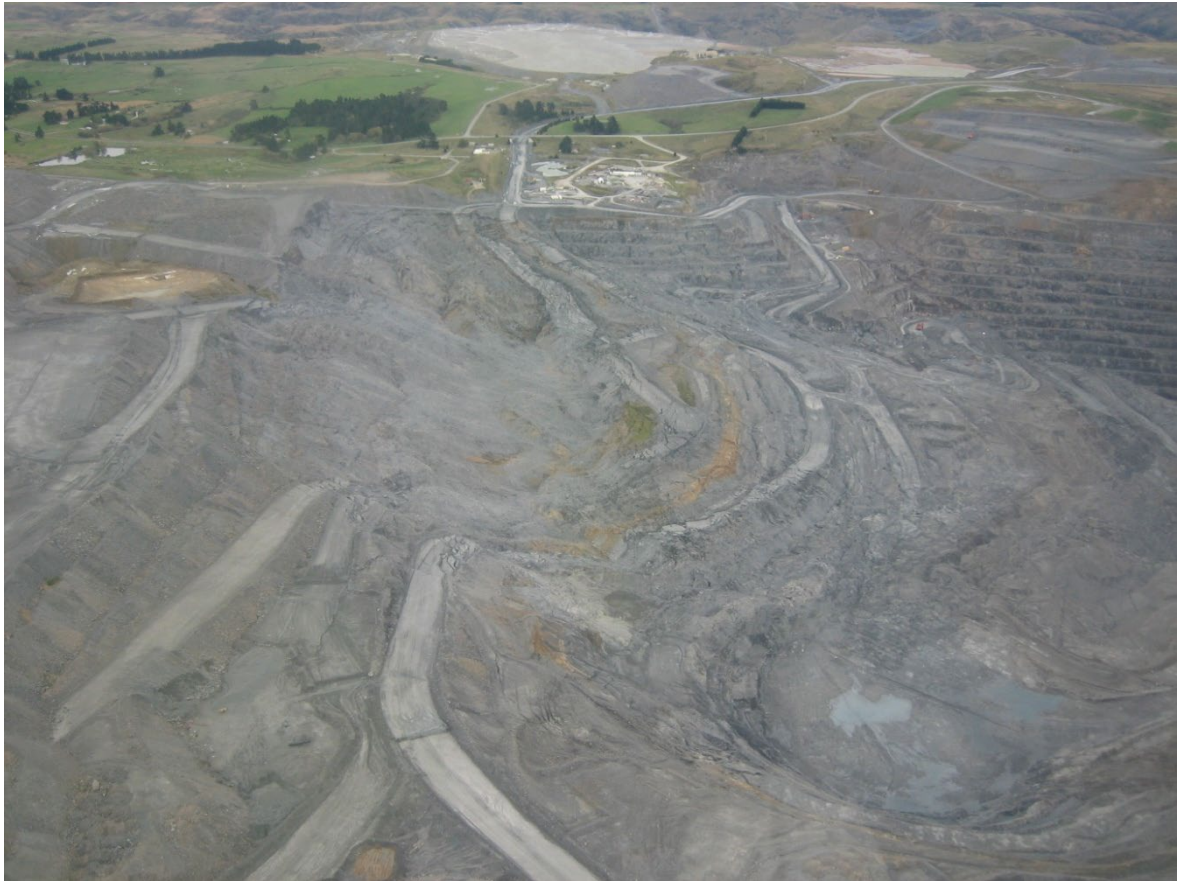
Photo 6: Aerial view of the west wall taken from the south looking roughly along strike towards the north. The distance the west wall has moved can be gauged by the offset seen in the haul roads. The smooth plane in mid-photo is the FF.
