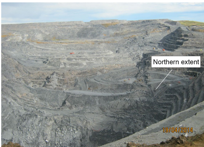
Photo 5: Northern and southern extent of failure.
