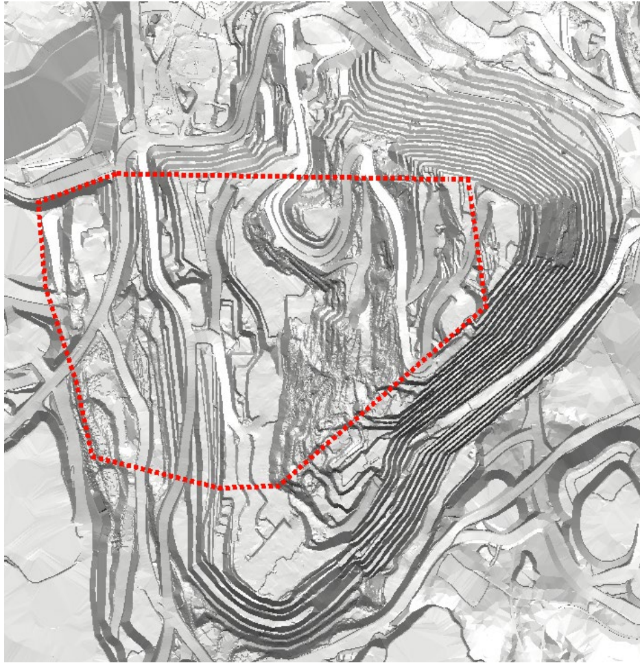
Inset 3: Approximate extents of the April 2014 20 Mm 3 west wall failure.
