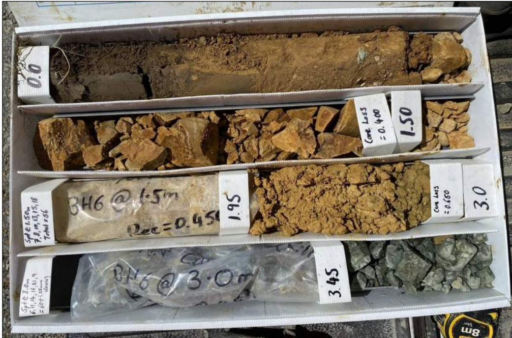
Photo BH6.1 BH6 Box 1: 0.0m to 4.5m
