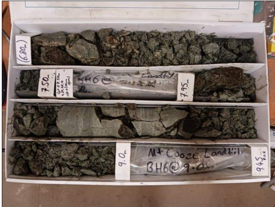
Photo BH6.3 BH6 Box 3: 6.8m to 9.45m
