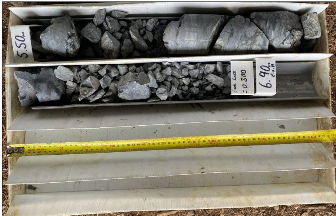
Photo BH9.2 BH9 Box 2: 5.5m to 6.9m
