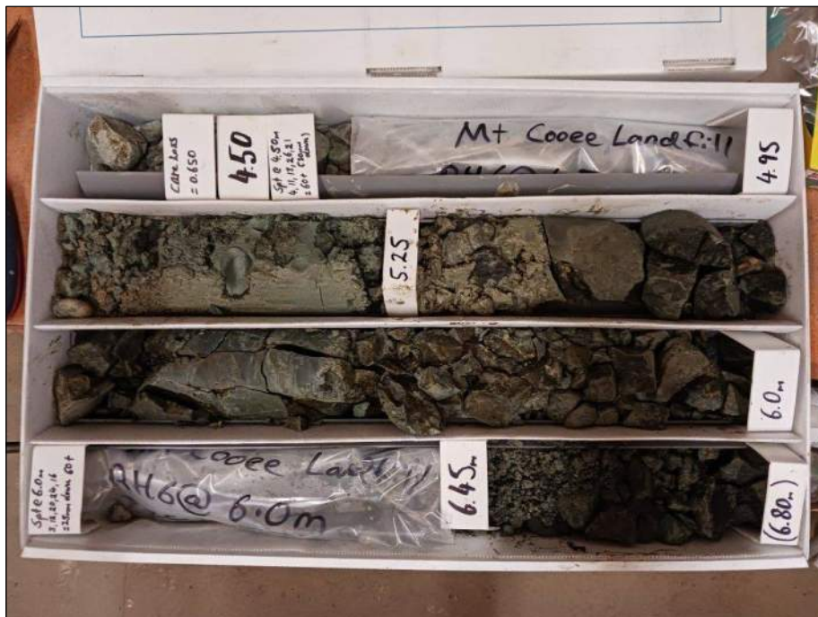
Photo BH6.2 BH6 Box 2: 4.5m to 6.8m
