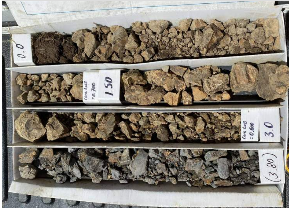
Photo BH4.1 BH4 Box 1: 0.0m to 3.8m
