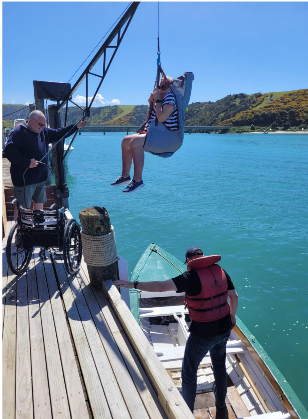
Original crane has been repurposed to provide safe, all tide access to boats
