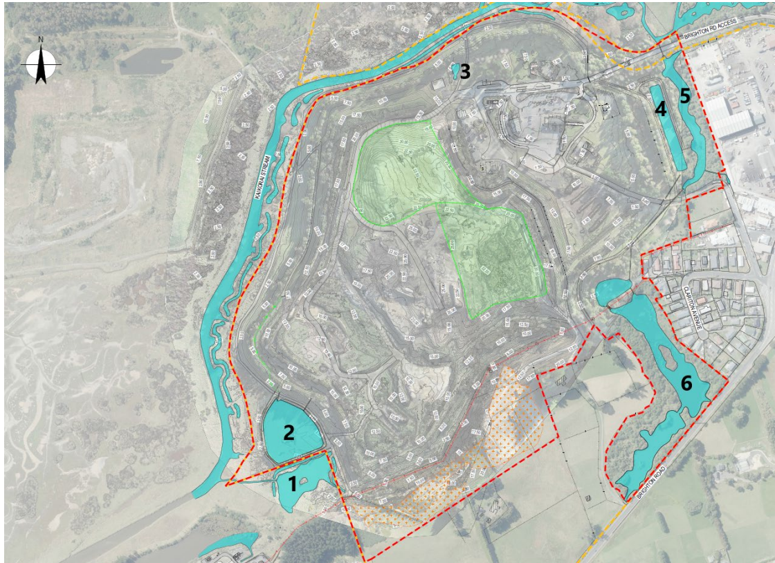
Figure 15 Artificial surface waterbodies on site. 1 & 2 western sedimentation pond including overflow; 3 northern leachate pond; 4 eastern sedimentation pond; 5 eastern constructed wetland; 6 southeastern constructed wetlands. The borrow area sedimentation pond is not shown in this view. Source: RM23.185 Design Report, with modifications (numbering) by the report writer.
