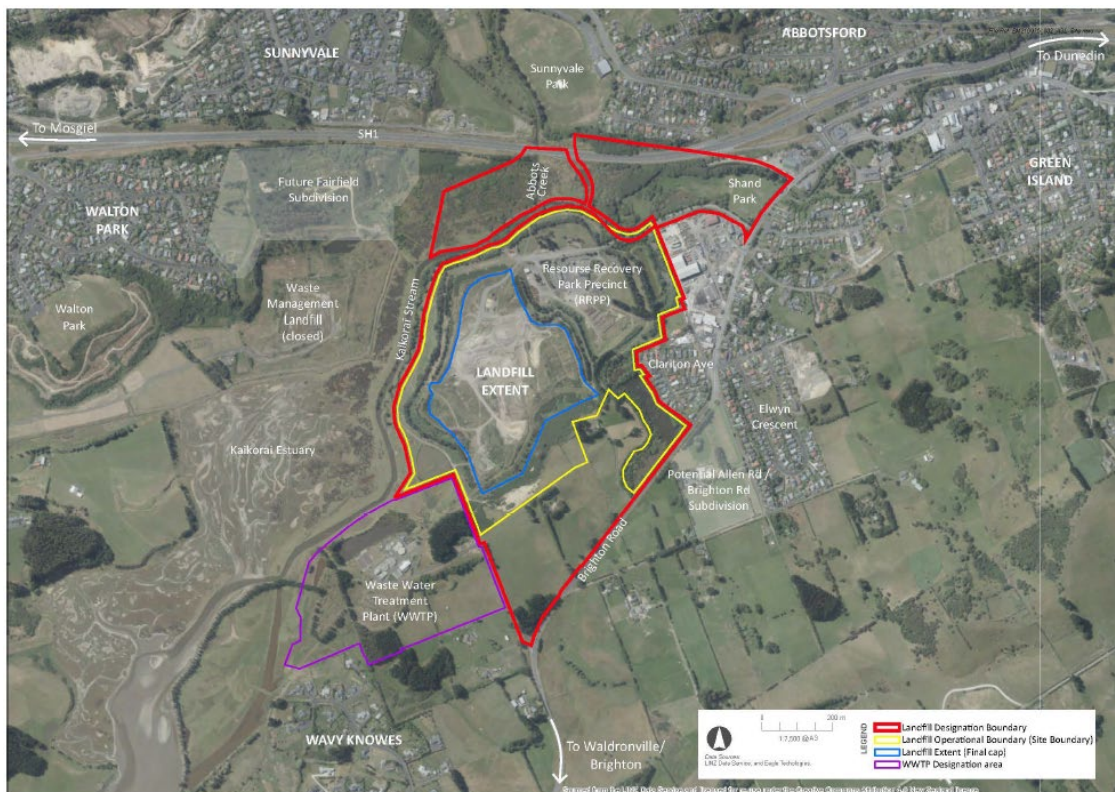
Figure 12 Landfill designation boundary (red line), operational boundary i.e. area historically used for waste placement (yellow line), landfill extent i.e. area of landfill still in operation (blue line), and GIWWTP designation area (purple line). Source: RM23.185 application.
