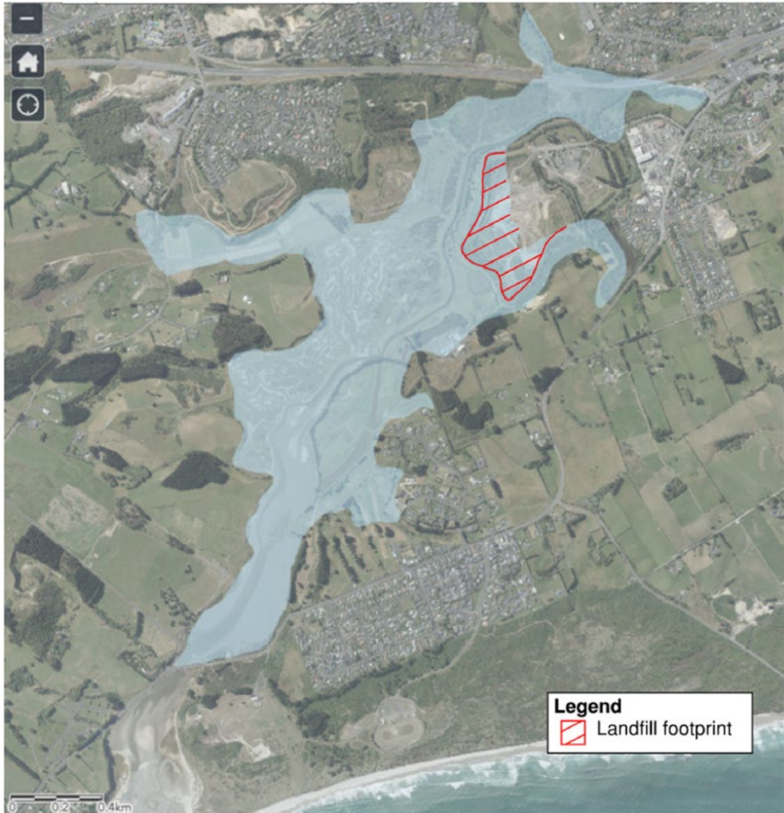
Figure 13 Fluvial flood risk area. Source: RM23.185 Design Report.
