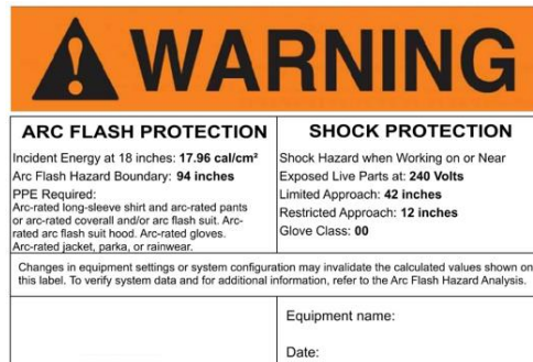
Figure B17-1 High Voltage Warning Label Illustration
