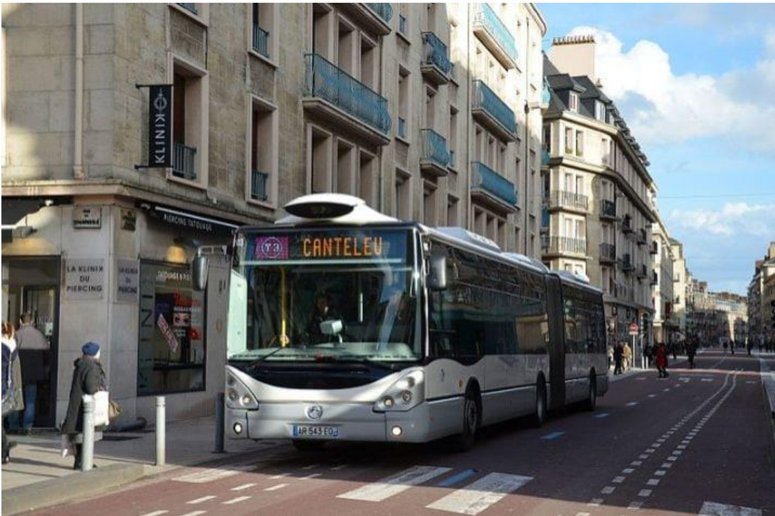
Figure 52: Rouen bus rapid transit system which is optically guided at bus stops (Source: Mobilys)
