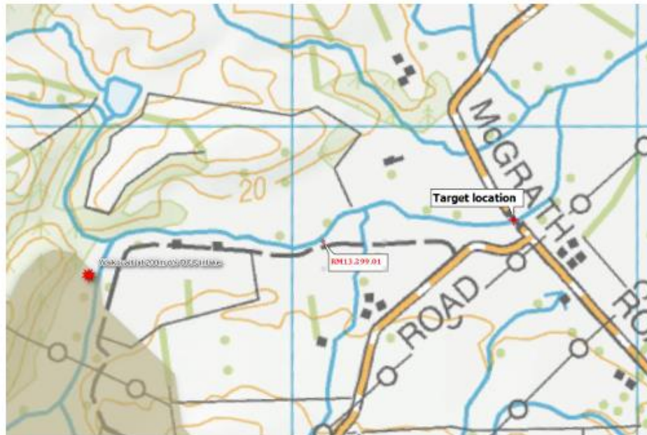
Figure 3. The target location relative to the flow recorder at DCC intake
