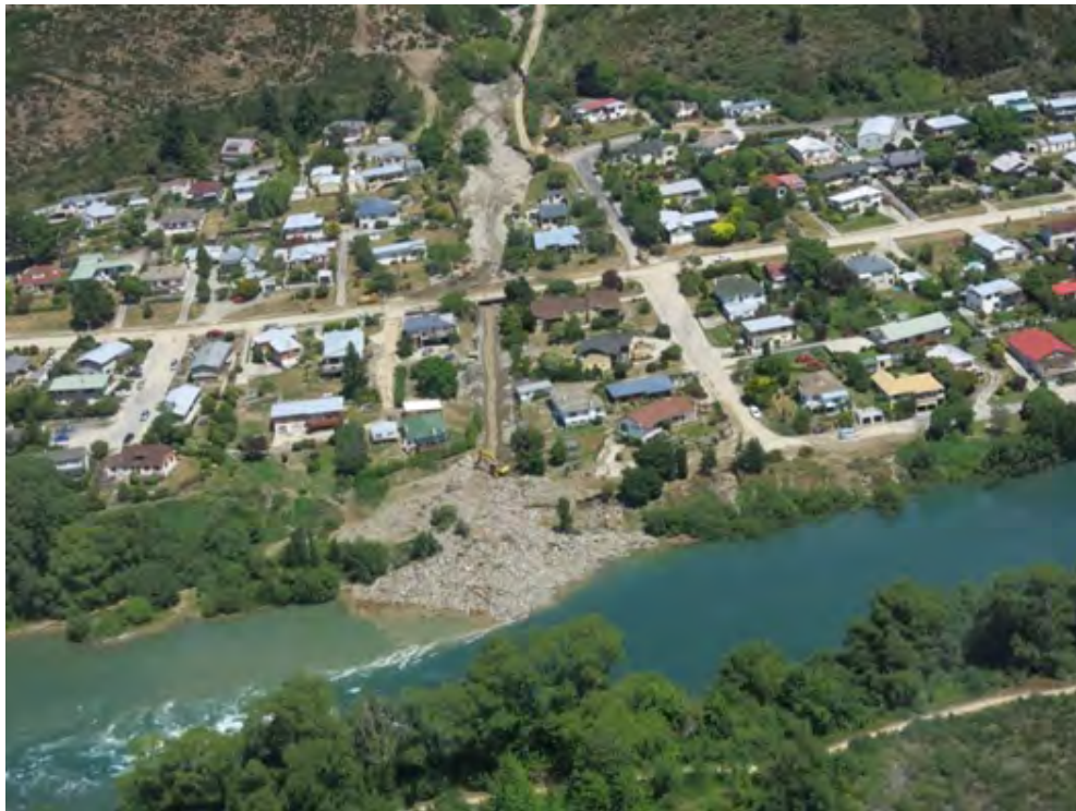
Figure 8: Impacts of the November 2017 debris flow event at Reservoir Creek, showing the extensive deposition of sediment debris at the confluence with the Clutha River.
