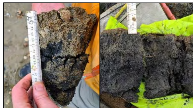
Deep aRPD at Site B1 in November 2022 (left), compared with the shallower appearance in December 2023 (right).
