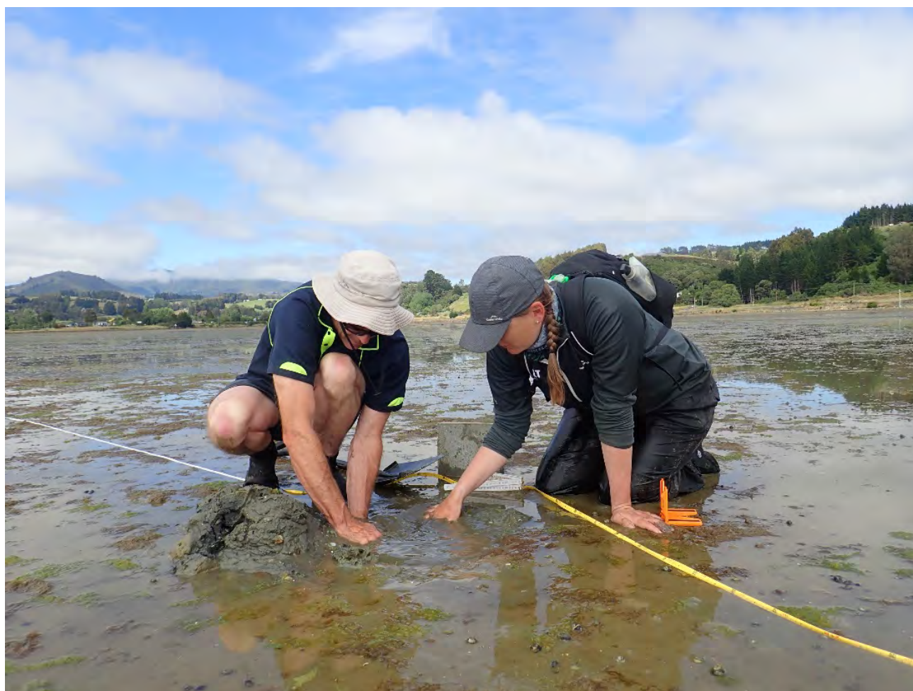
Figure 3: Sediment Plate installation in Blueskin Bay during fine scale monitoring
