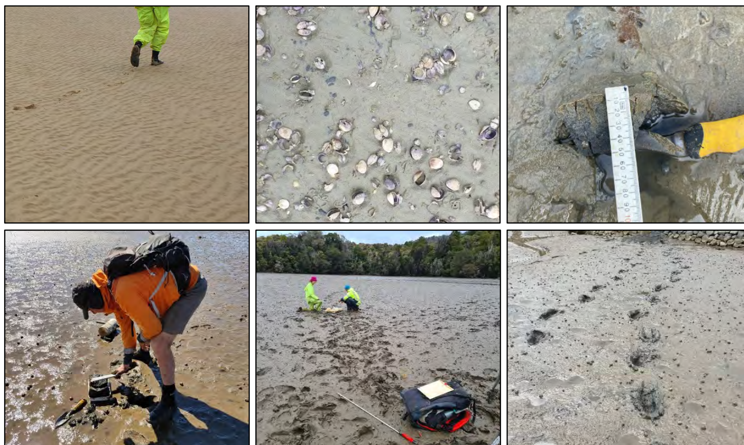
Examples of substrate types: Top row (L to R); mobile sand (mS; 0-10%), firm shell/sand (fShS; 0-10%), firm sand (fS; 0-10%).
