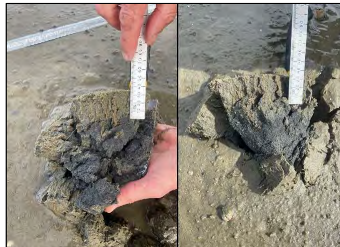
Deep sediment oxygenation (aRPD transition from brown to dark grey sediment) at Site A (left) and Site B (right) in December 2023.
