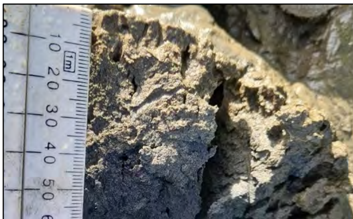
Sediment aRPD at Site B, rated as 'Good' (aRPD ~40mm).
