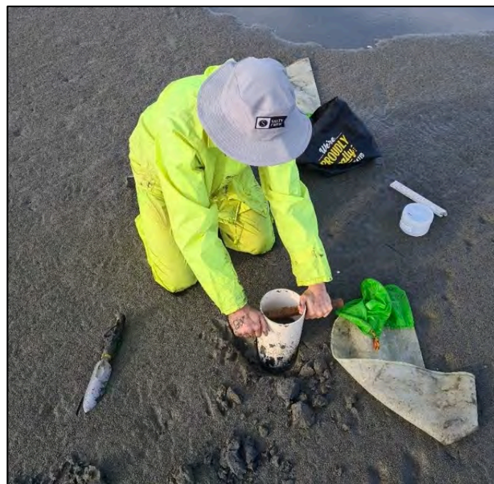
Sediment core sampling for macrofauna at Site 4 in the lower Catlins Lake.
