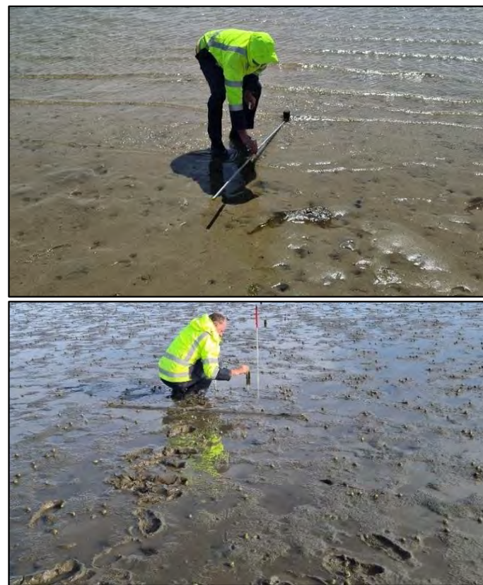
December 2023 site photos: Sand-dominated sediment at Site A1 near the main channel (top), and mud-dominated sediment with surface dwelling macrofauna at Site B (bottom).
