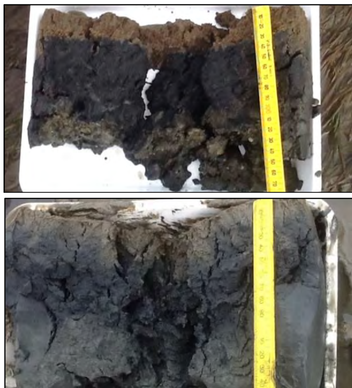
Sediment core profiles from Site B (top, sand) and C (bottom, muddy sand) in 2019. Oxygen-depleted sediment is illustrated by the deeper grey/black colouring.
