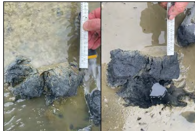
Shallow sediment oxygenation (aRPD transition from brown to dark grey sediment) at Site A (left) and Site B (right) in December 2023.
