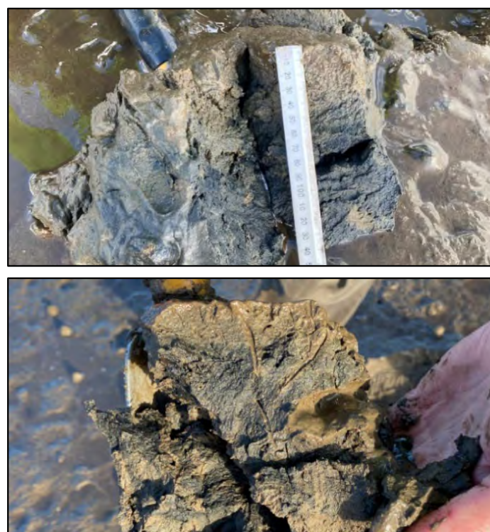
Sediment core profiles from Site A (top, sand) and B (bottom, sandy mud) in December 2022. Oxygen-depleted sediment is illustrated by the deeper grey/black colour.
