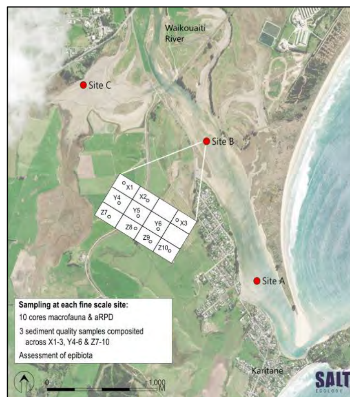
Fig. 1. Location of the three fine-scale monitoring sites in Waikouaiti Estuary. The schematic depicts the sediment sample and macrofauna core collection. Information on site GPS positions and other location information is provided in Robertson et al. (2017).
