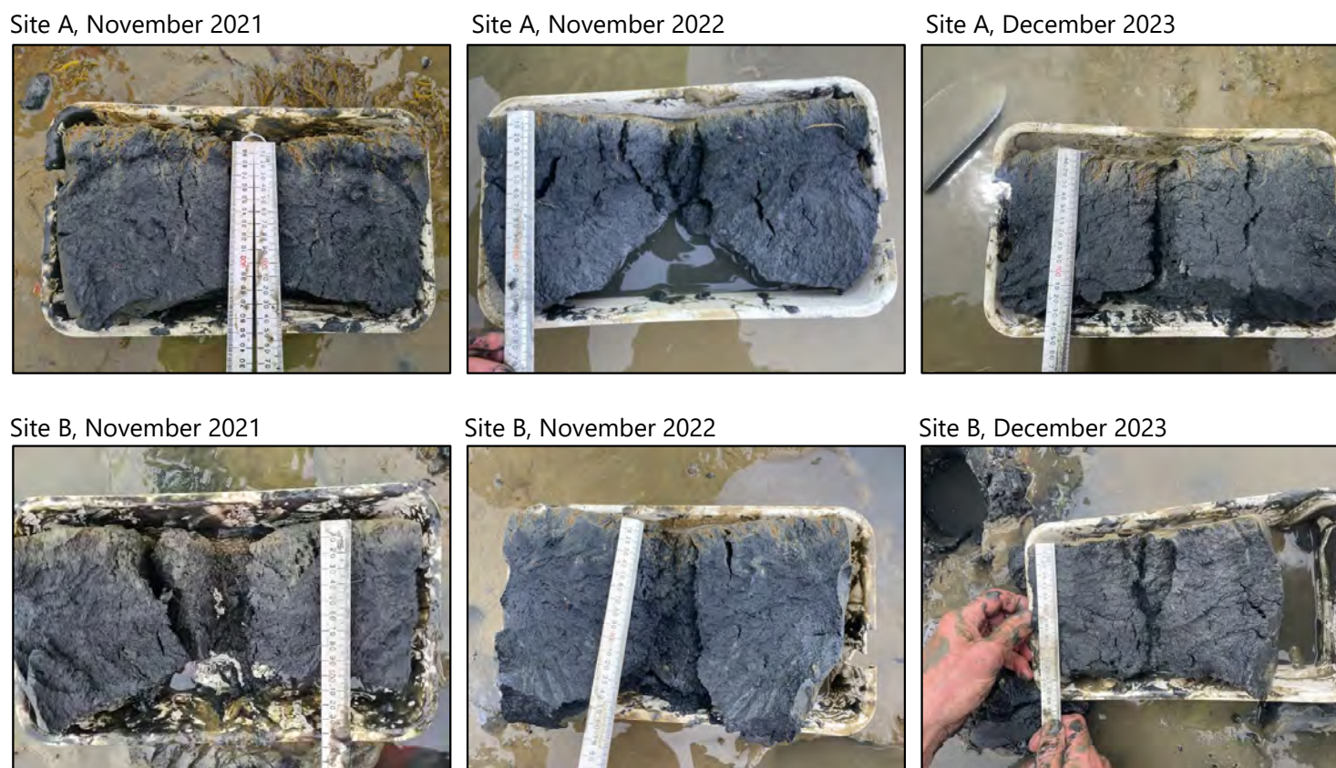
Fig. 4. Sediment core profiles from Site A and B. Oxygen-depleted sediment is illustrated by the deeper grey/black colour.
