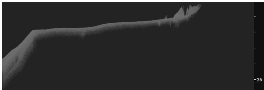
Figure 3-9: Bathymetry of Site 5 – Waipuke park at Lake Karaapiro. Maximum trace distance is 204.2 m. Top right side is the lake shore the steep gradient on the left side is a ridge leading to deeper water across the bathymetry transect.
