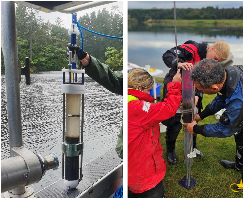
Figure 2-8: Gravity corer deployment (left) and corer substrate sample processing (right).
