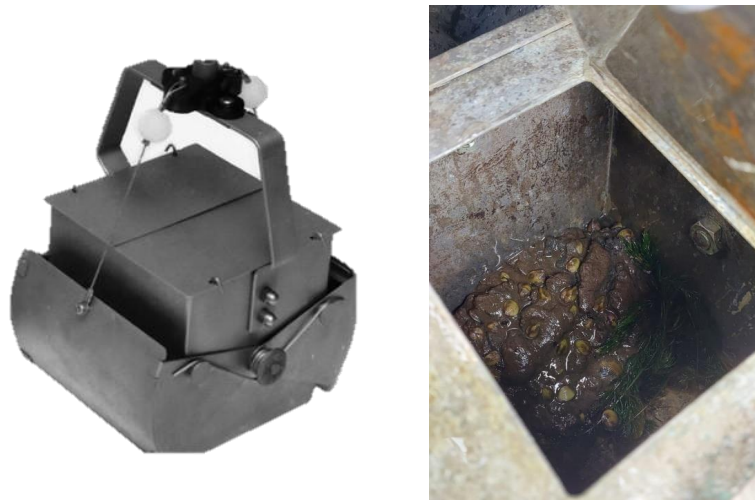
Figure 2-10: Example of Ekman grab device deployed (left). Ekman grab sampler containing sediment recovered from Lake Karaapiro (right).
