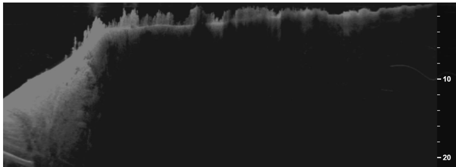
Figure 3-2: Bathymetry of Site 1 - Boat ramp at Lake Maraetai. Maximum trace distance is 122.8 metres. Top right side is the lake shore the steep gradient on the left side is a ridge leading to deeper water across the bathymetry transect.
