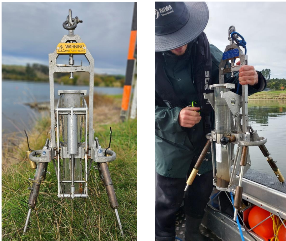
Figure 2-9: Jenkins Surface Mud Corer (left). Preparing it for deployment (right).
