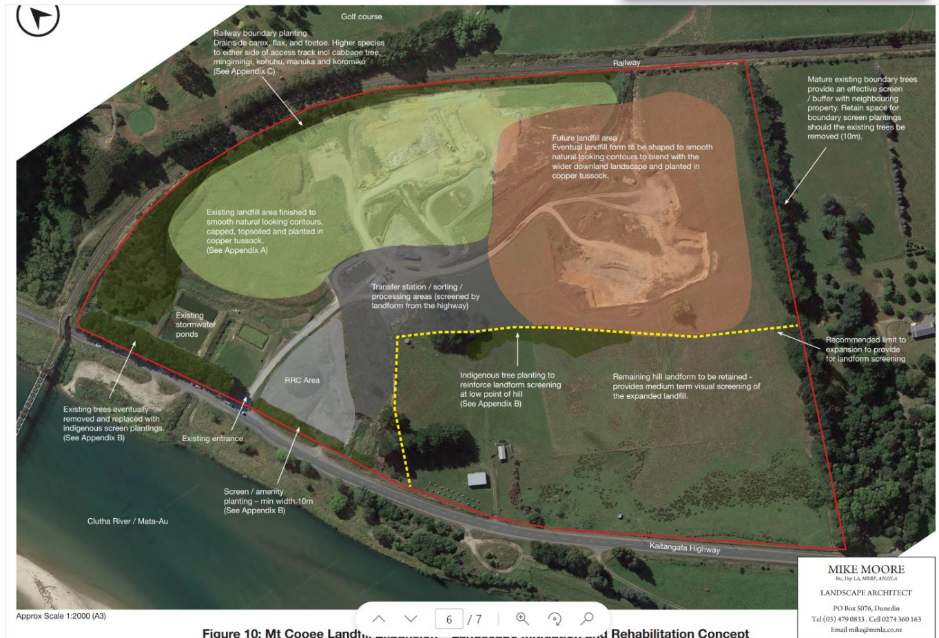
Figure 10: Mt Cooee Landfill Expansion, Landscape Mitigation and Rehabilitation Concept
