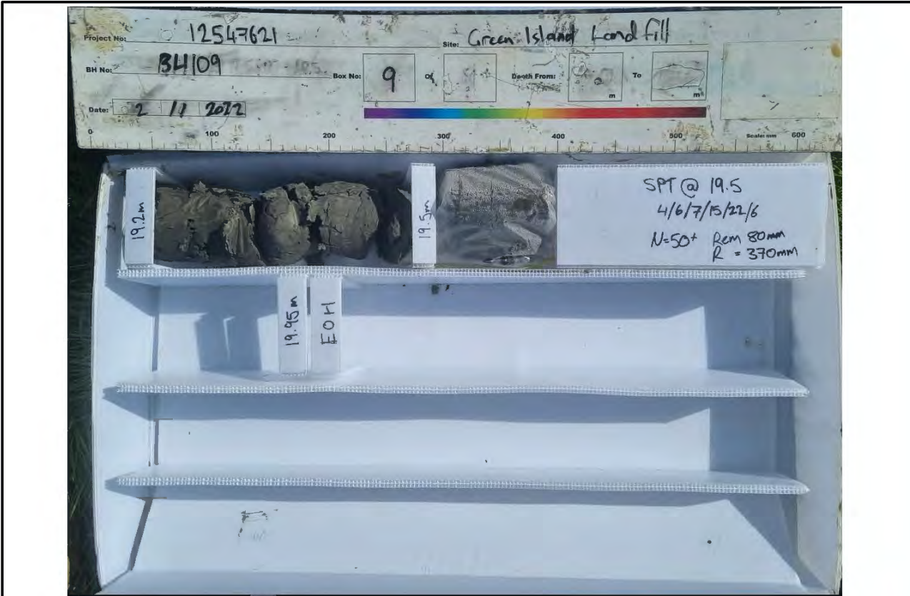
Core Box 9, Depth: 19.2 to 21.6 m
