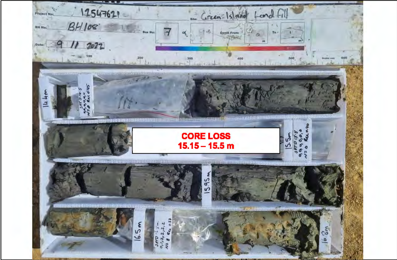
Core Box 7, Depth: 14.4 to 16.8 m
