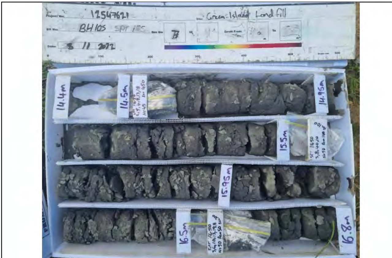
Core Box 7, Depth: 14.4 to 16.8 m
