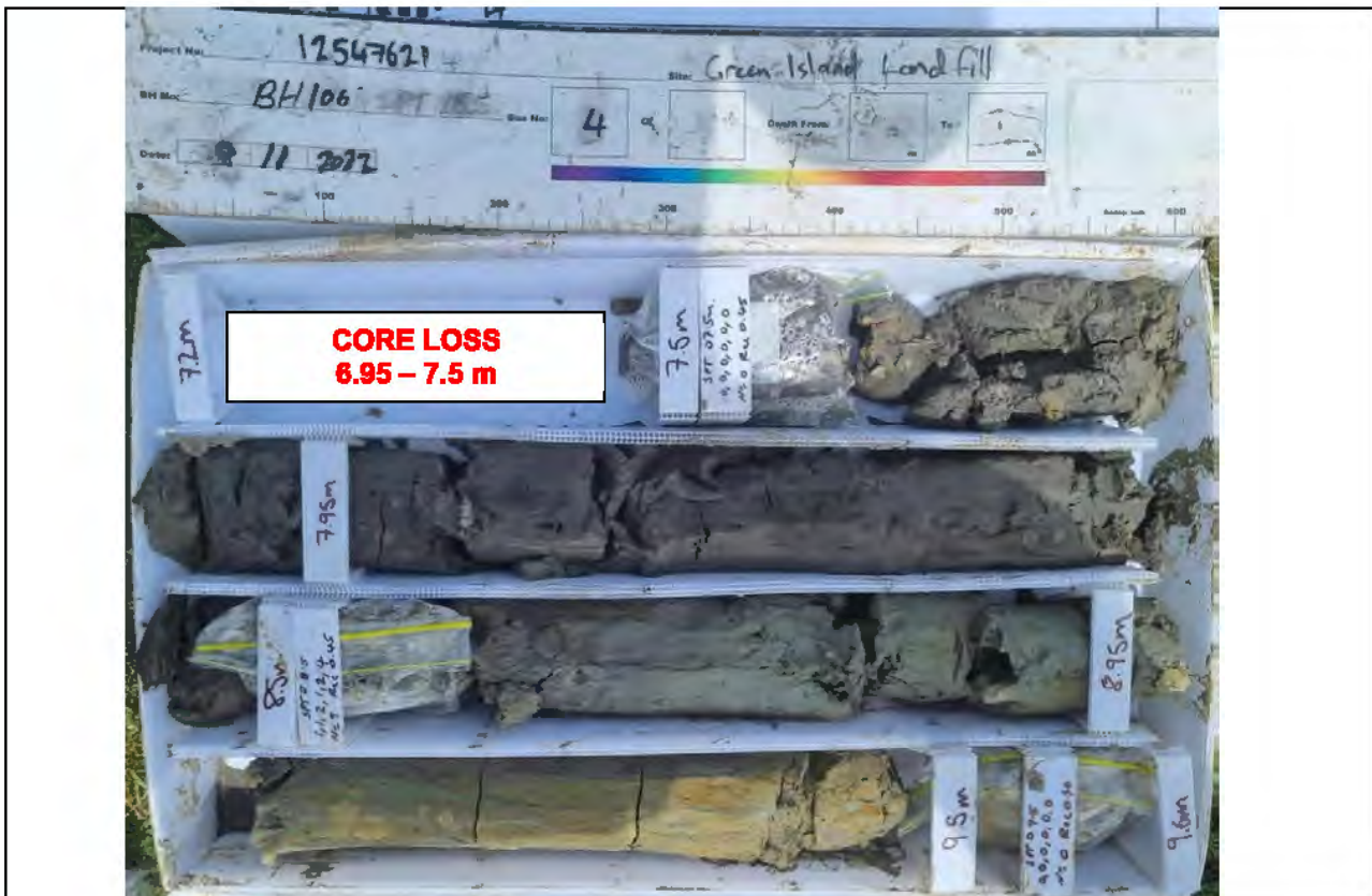
Core Box 4, Depth: 7.2 to 9.6 m
