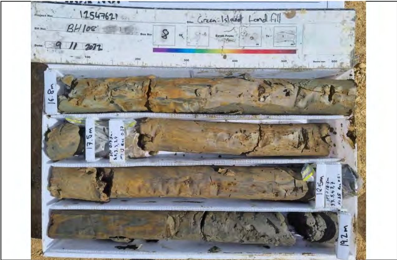
Core Box 8, Depth: 16.8 to 19.2 m
