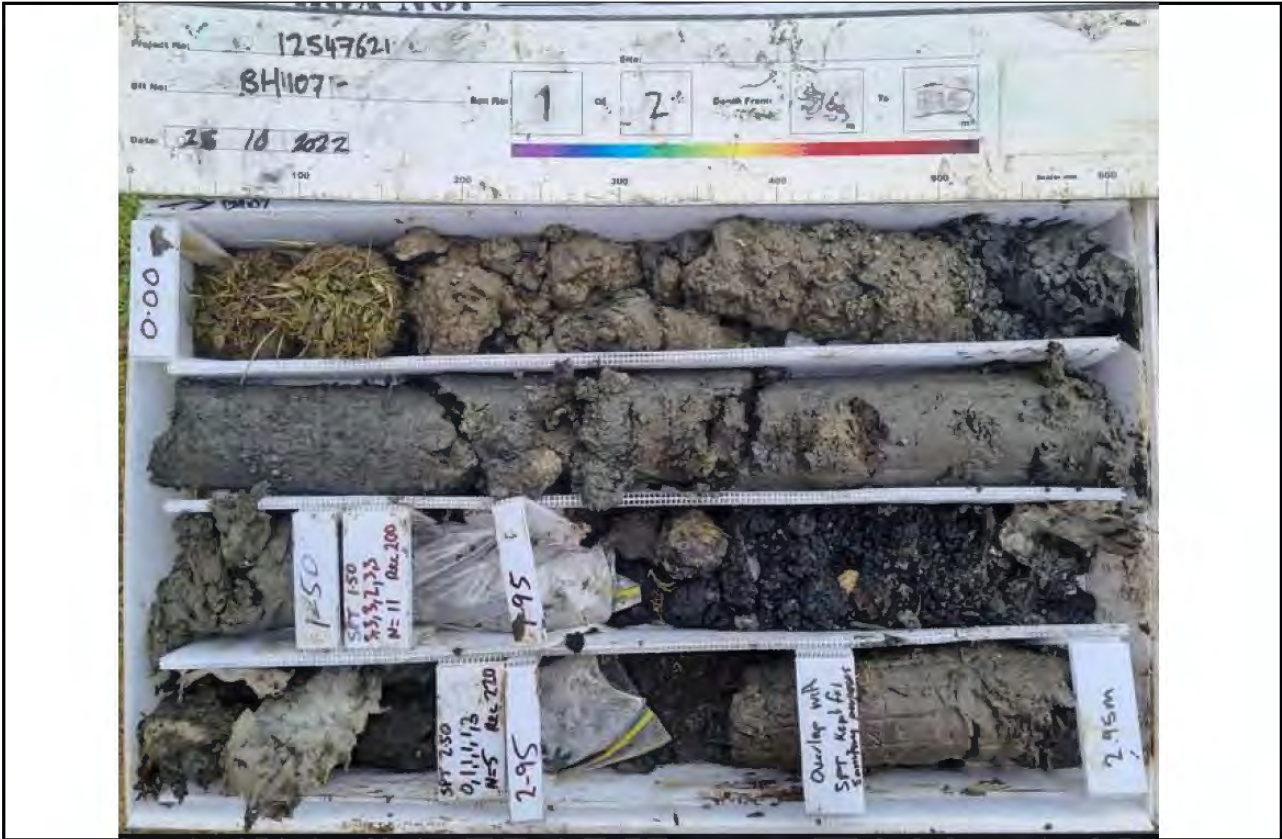
Core Box 1, Depth: 0.0 to 2.95 m
