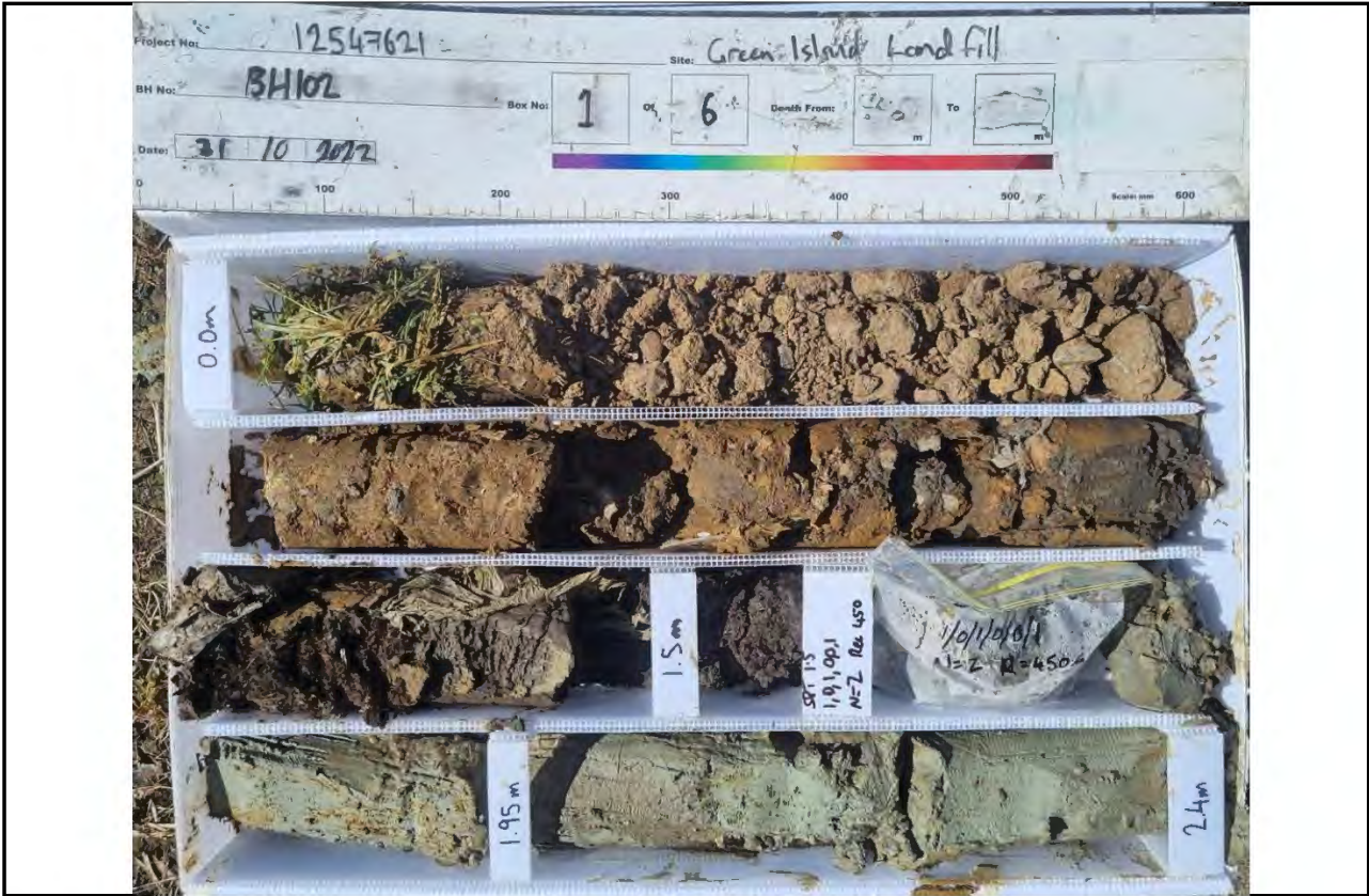
Core Box 1, Depth: 0.0 to 2.4 m
