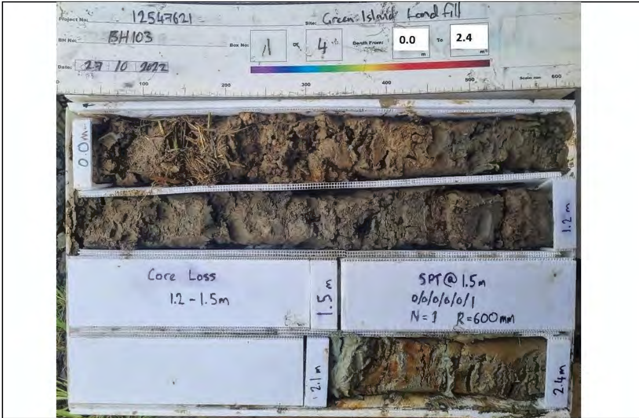
Core Box 1, Depth: 0.0 to 2.4 m
