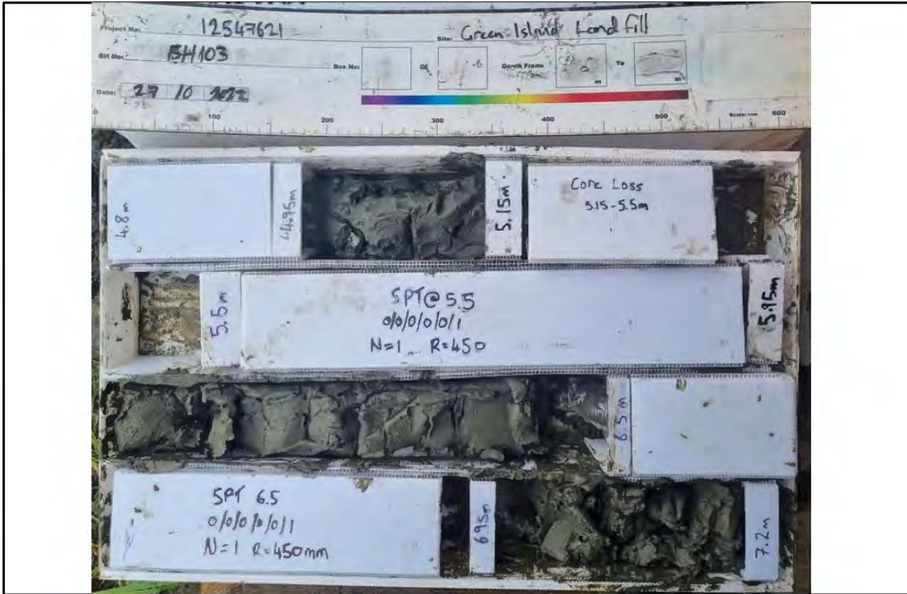
Core Box 3, Depth: 4.8 to 7.2 m
