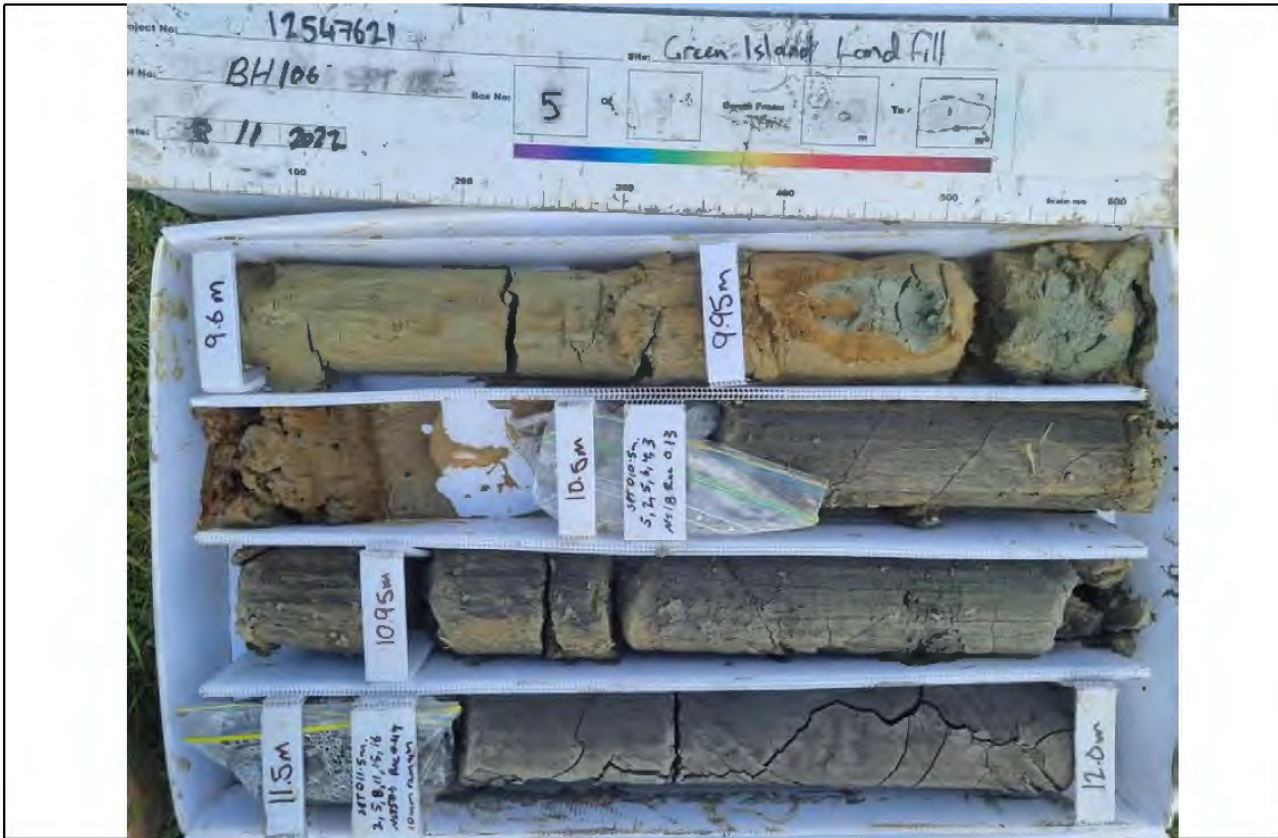
Core Box 5, Depth: 9.6 to 12.0 m
