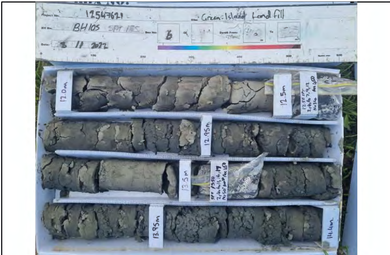
Core Box 6, Depth: 12.0 to 14.4 m
