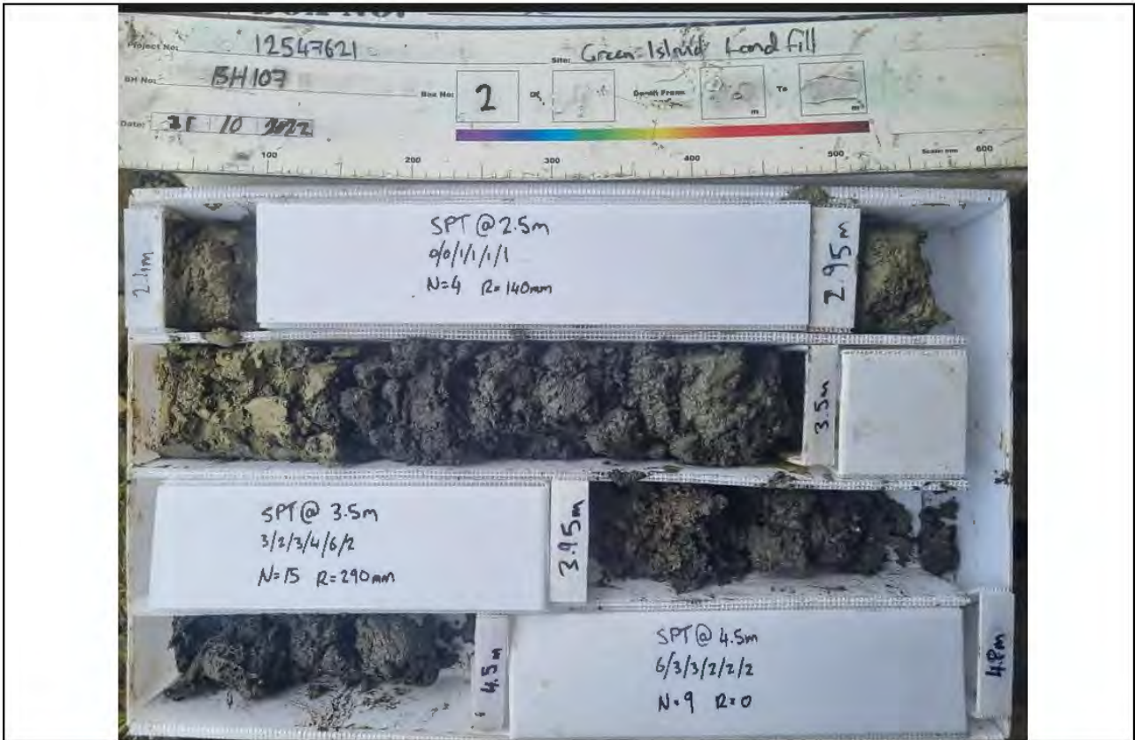
Core Box 2, Depth: 2.4 to 4.8 m
