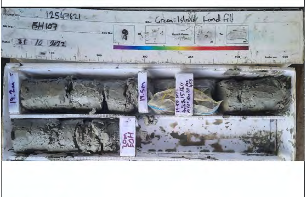
Core Box 9, Depth: 19.2 to 20 m
