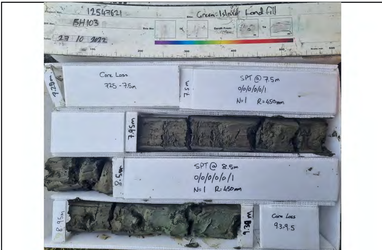
Core Box 4, Depth: 7.2 to 9.6 m
