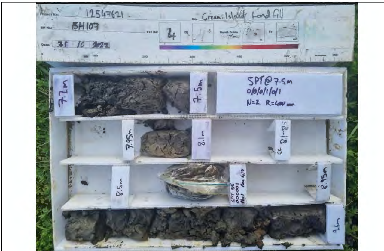
Core Box 4, Depth: 7.2 to 8.8 m
