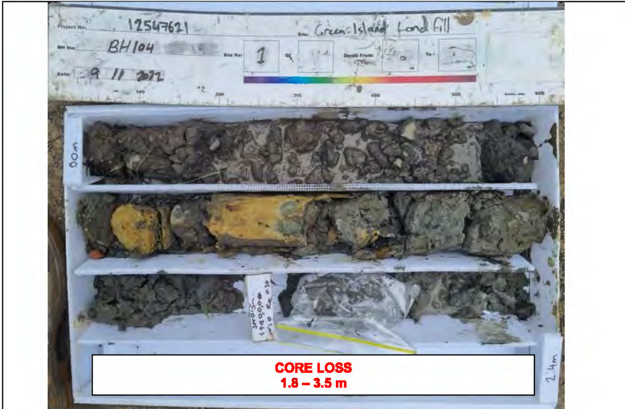
Core Box 1, Depth: 0.0 to 2.4 m
