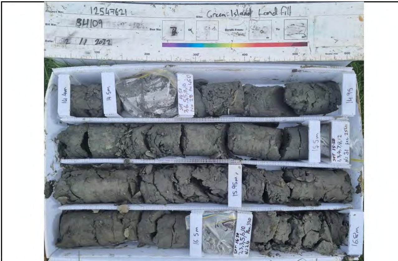
Core Box 7, Depth: 14.4 to 16.8 m
