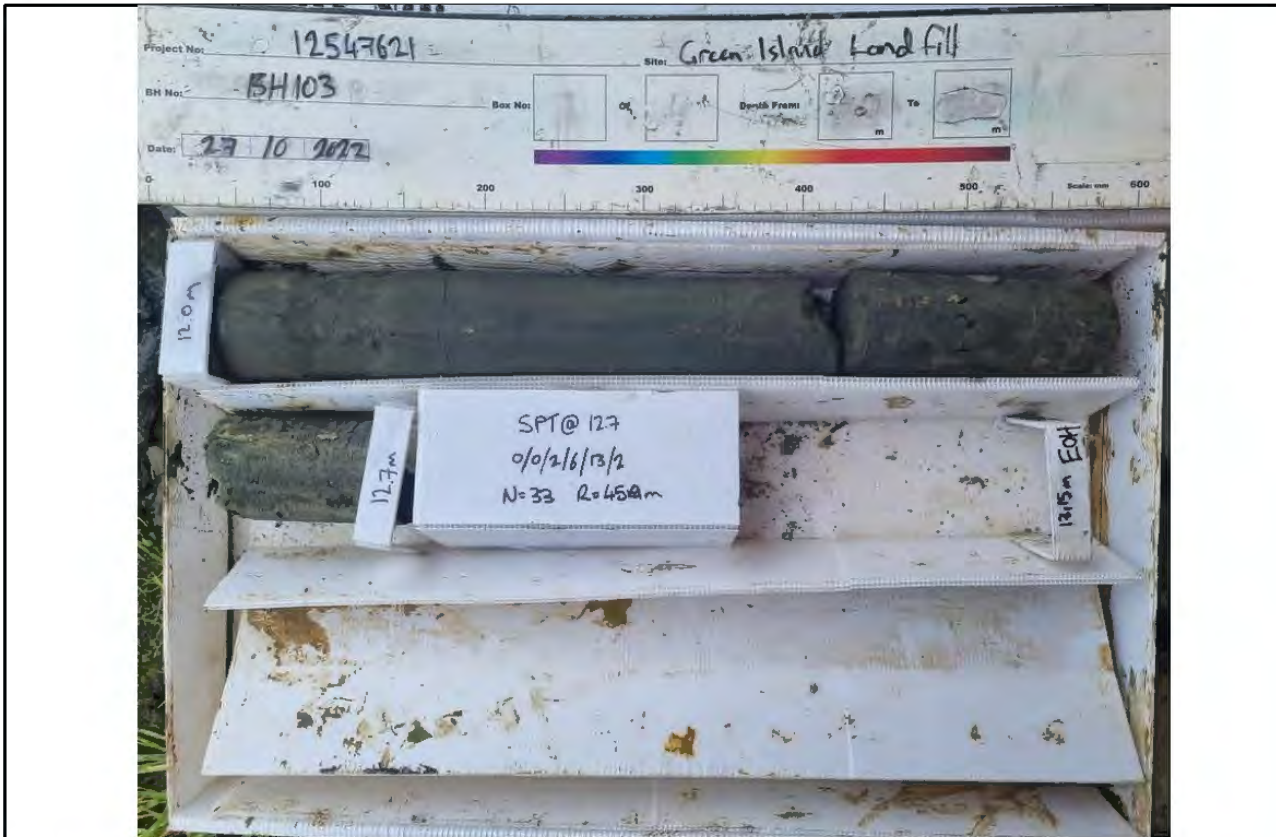
Core Box 6, Depth: 12.0 to 14.4 m
