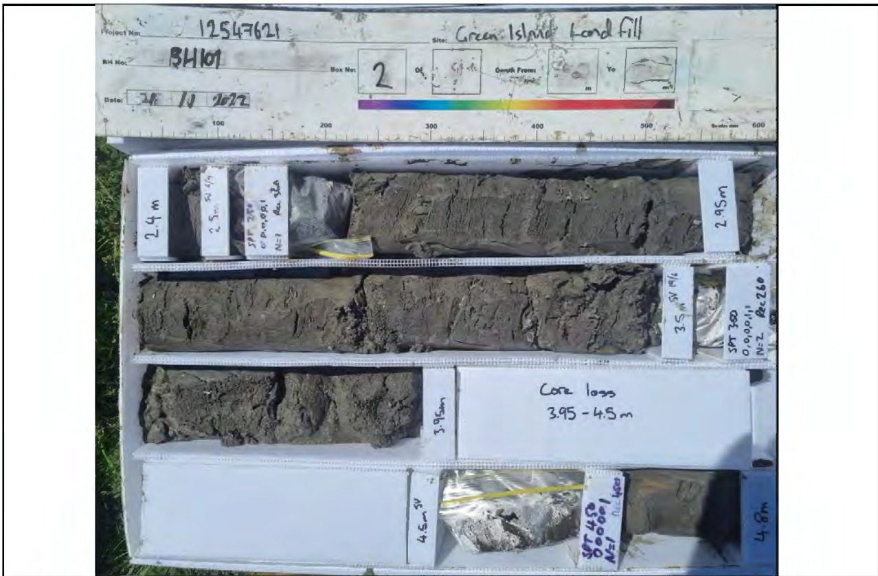
Core Box 2, Depth: 2.4 to 4.8 m
