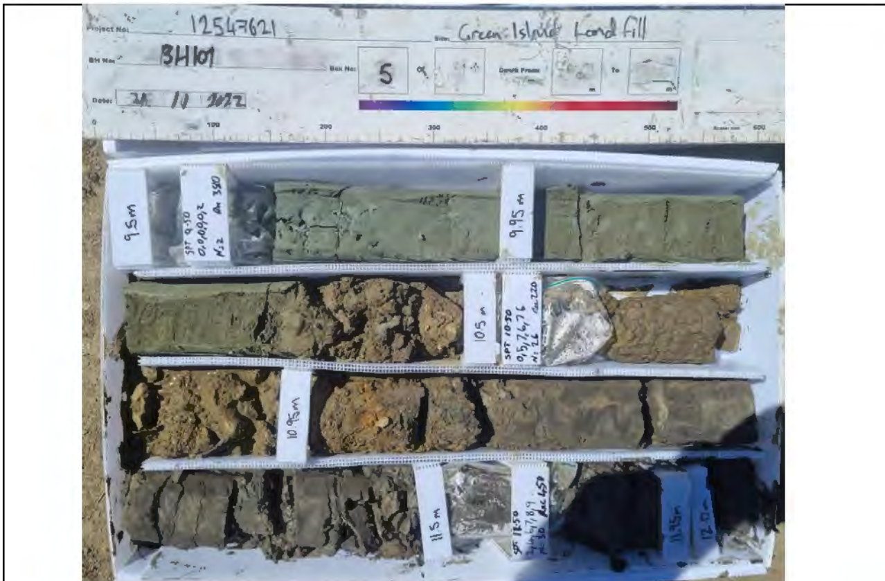
Core Box 5, Depth: 9.6 to 12.0 m
