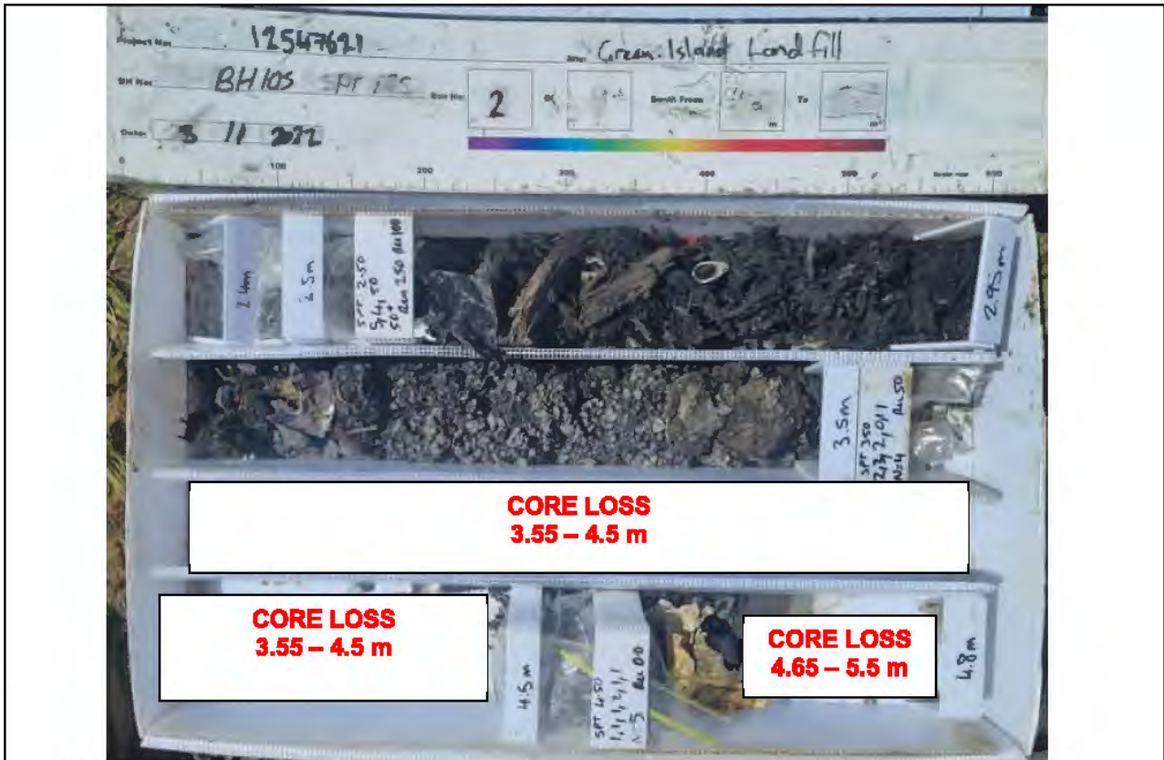
Core Box 2, Depth: 2.4 to 4.8 m
