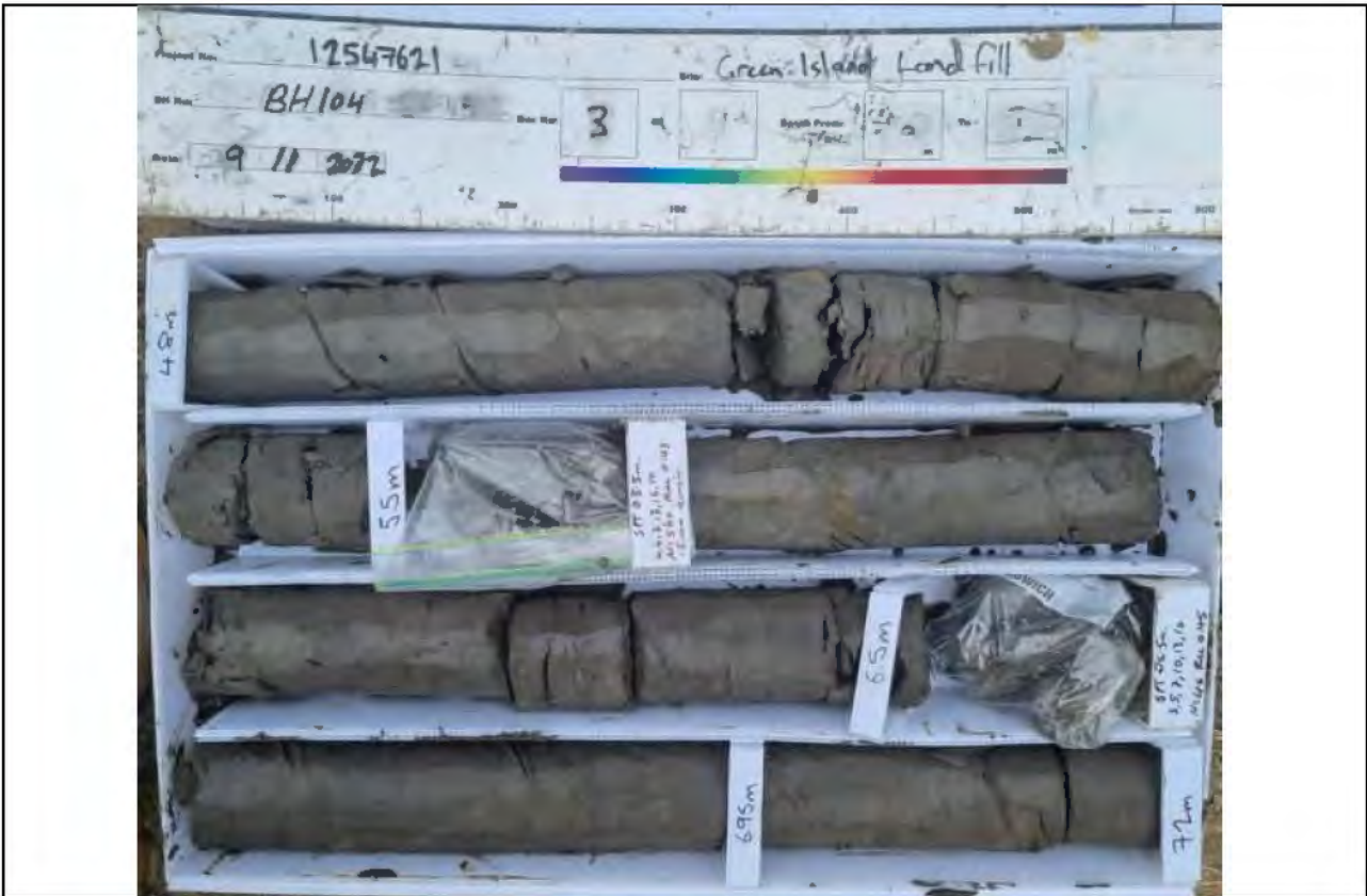
Core Box 3, Depth: 4.8 to 7.2 m
