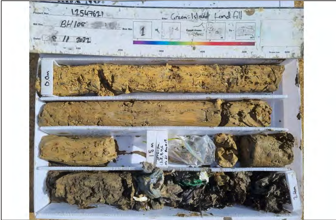
Core Box 1, Depth: 0.0 to 2.4 m
