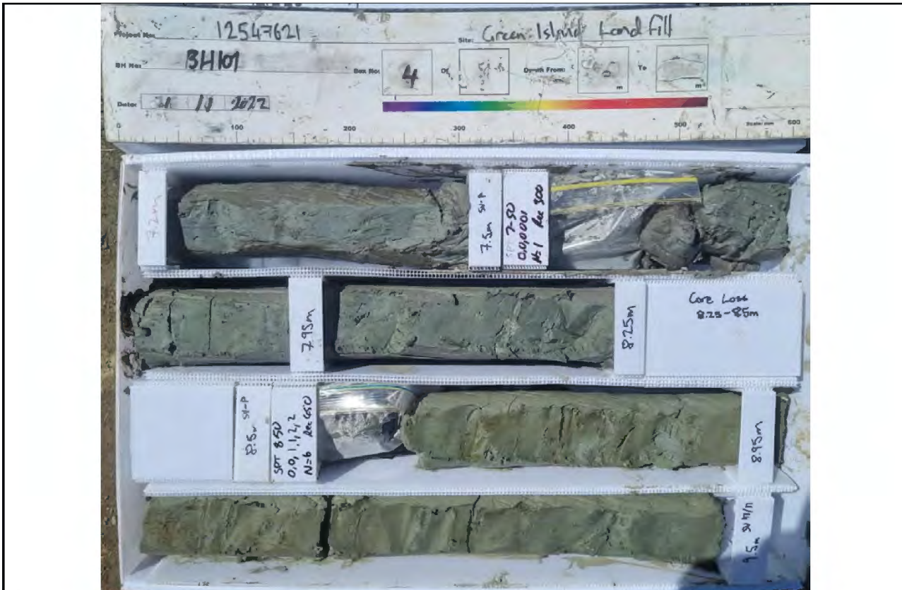
Core Box 4, Depth: 7.2 to 9.6 m
