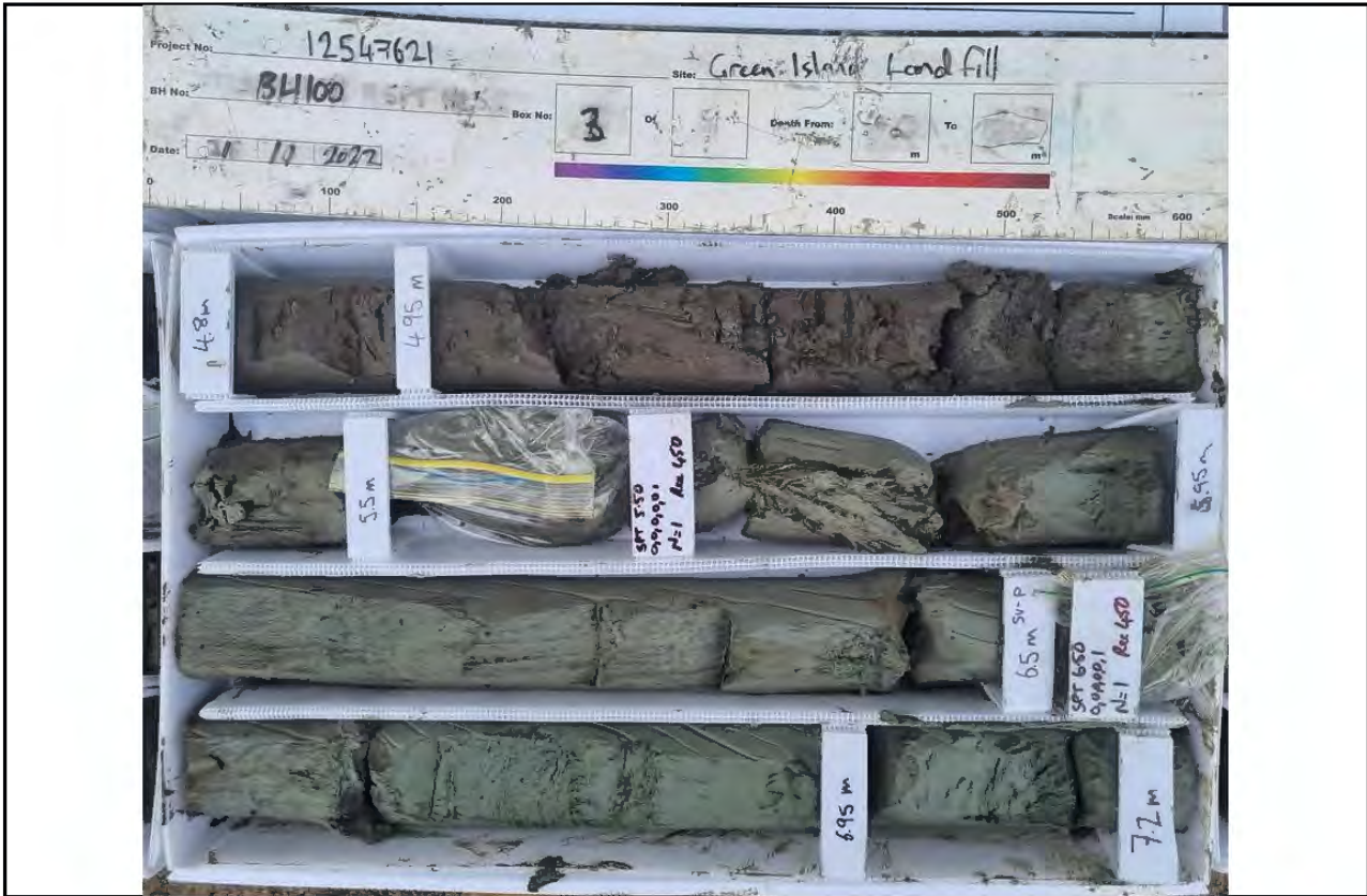
Core Box 3, Depth: 4.8 to 7.2 m
