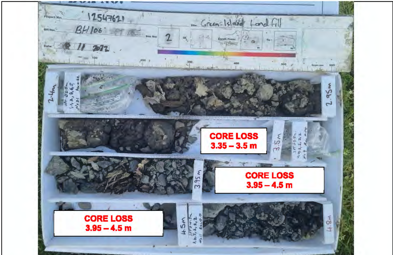
Core Box 2, Depth: 2.4 to 4.8 m
