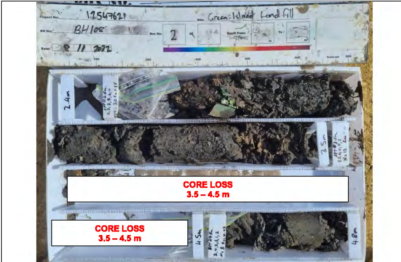
Core Box 2, Depth: 2.4 to 4.8 m
