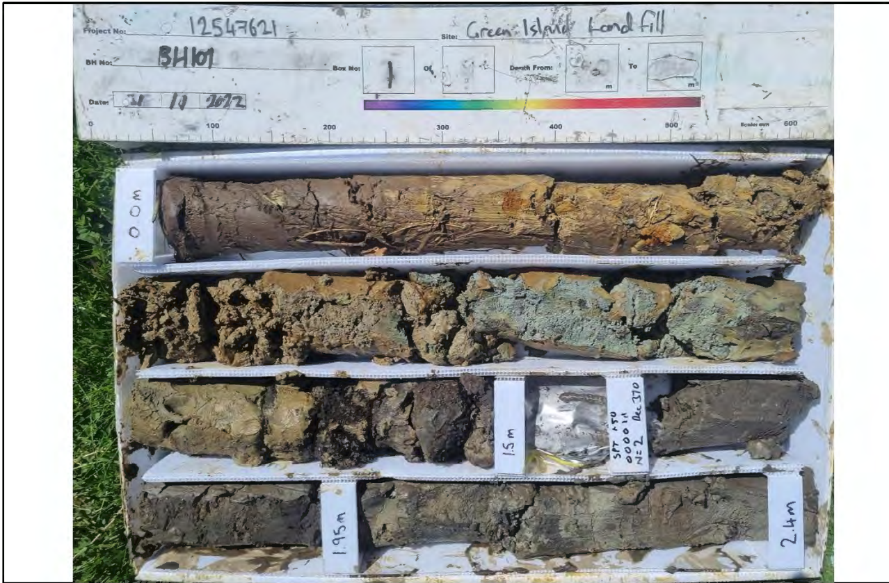
Core Box 1, Depth: 0.0 to 2.4 m
