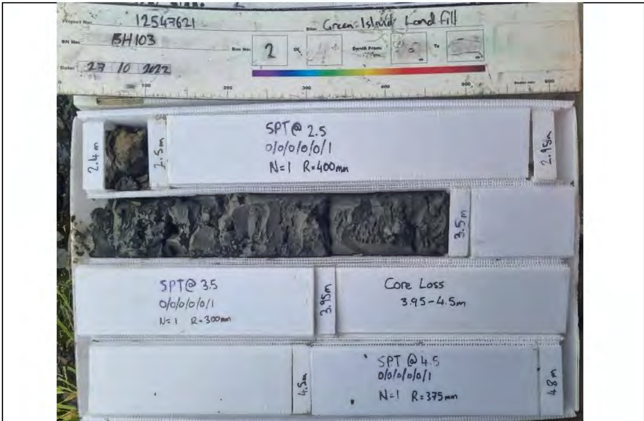
Core Box 2, Depth: 2.4 to 4.8 m
