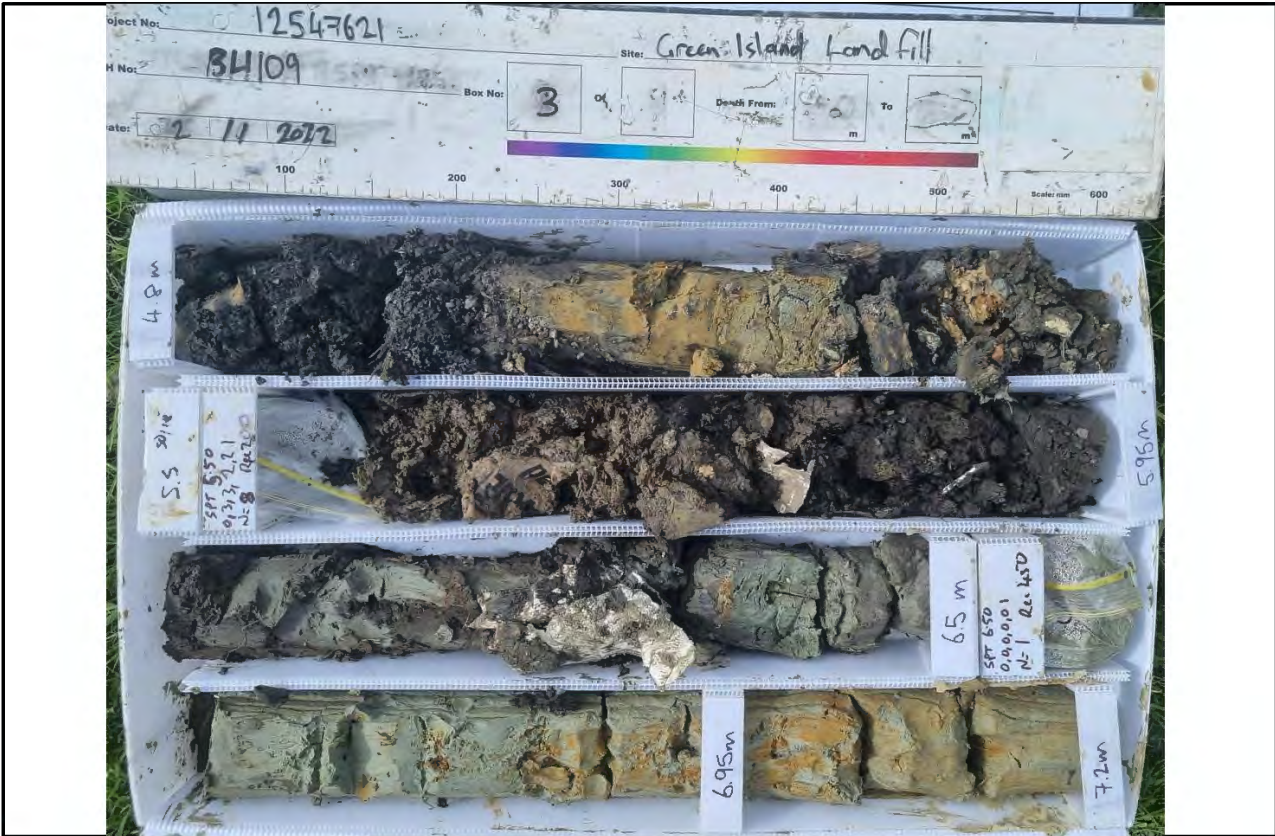
Core Box 3, Depth: 4.8 to 7.2 m
