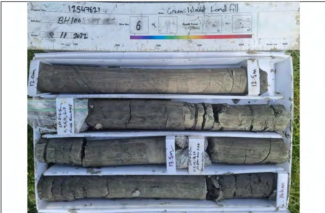
Core Box 6, Depth: 12.0 to 14.4 m
