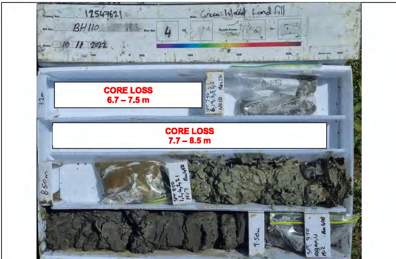
Core Box 4, Depth: 7.2 to 9.6 m
