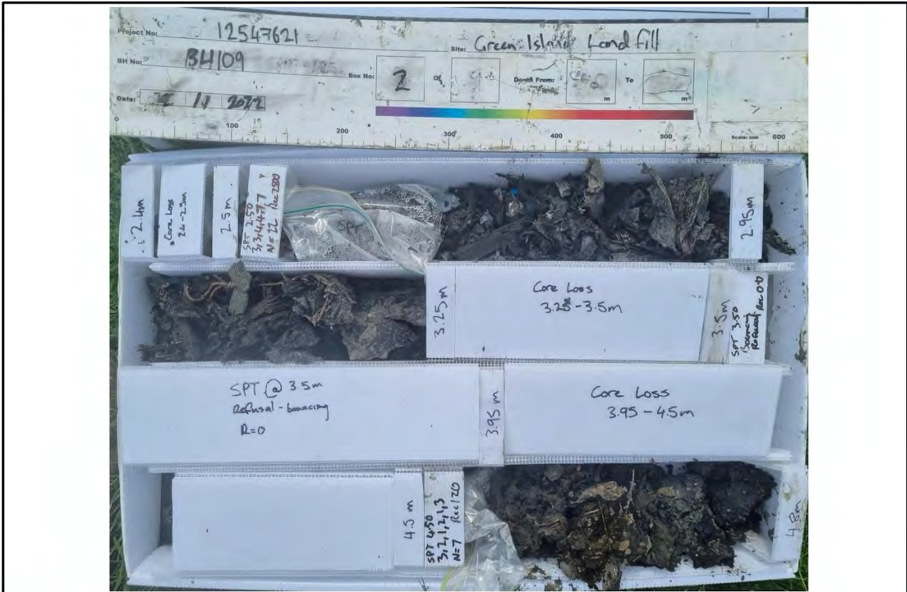
Core Box 2, Depth: 2.4 to 4.8 m
