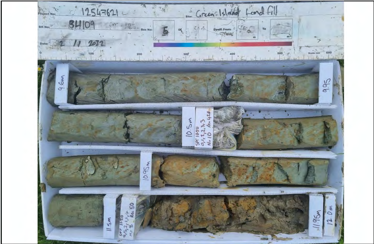
Core Box 5, Depth: 9.6 to 12.0 m
