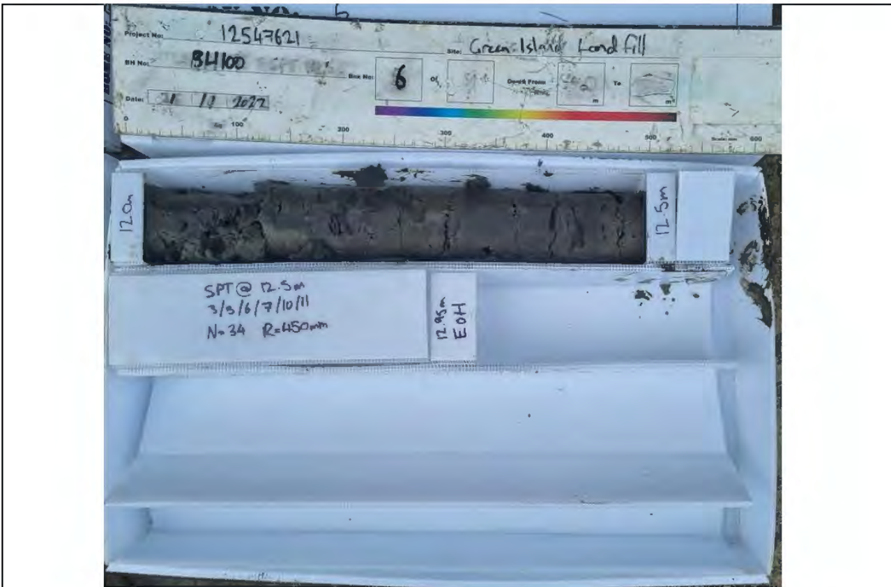
Core Box 6, Depth: 12.0 to 12.95 m
