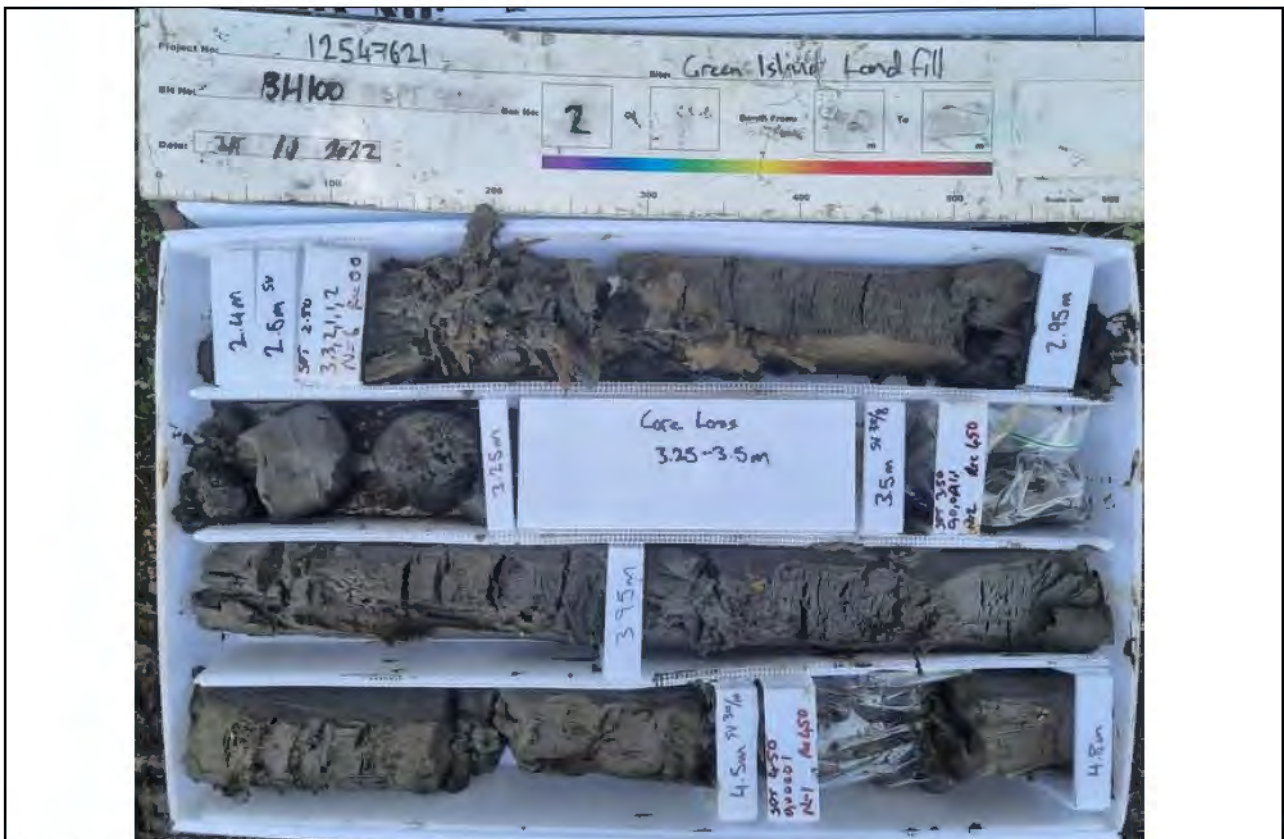
Core Box 2, Depth: 2.4 to 4.8 m
