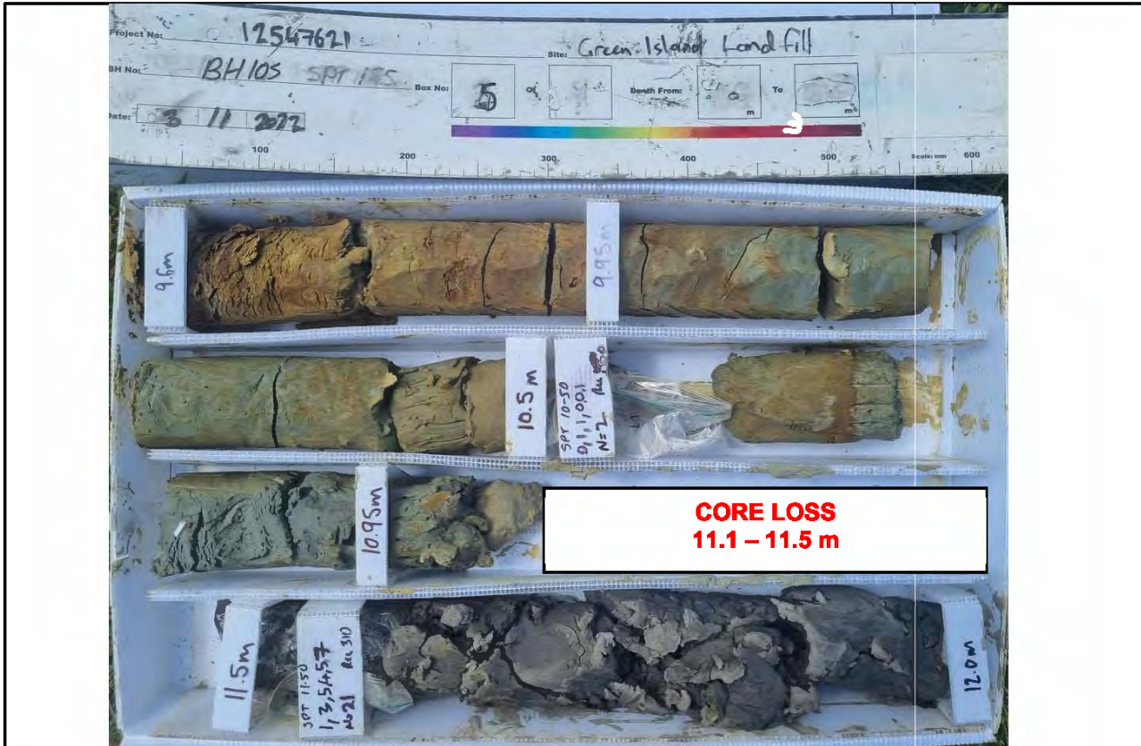
Core Box 5, Depth: 9.6 to 12.0 m
