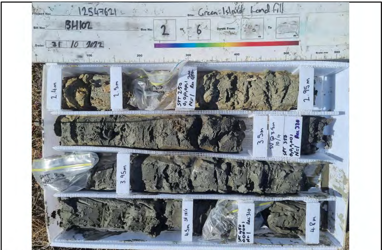
Core Box 2, Depth: 2.4 to 4.8 m
