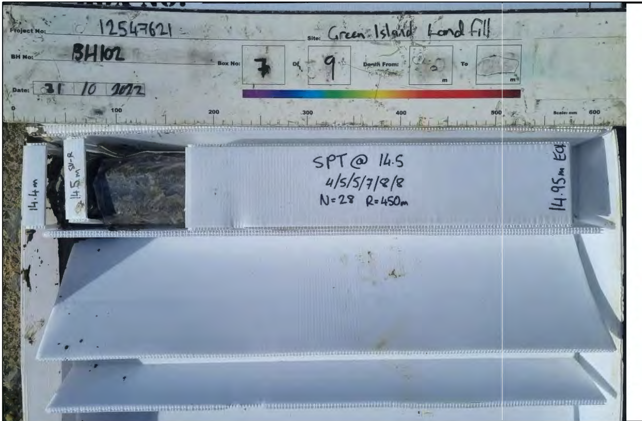
Core Box 7, Depth: 14.4 to 14.95 m
