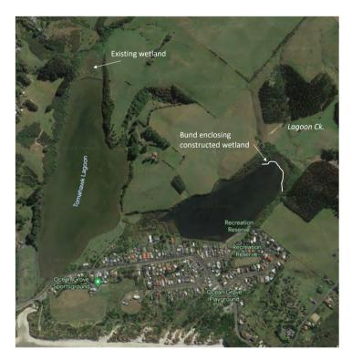
Figure 46. Bund location for potential constructed wetland at the inflow to Upper Tomahawk Lagoon.
