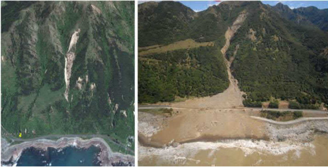
Figure 10.5 Rainfall induced debris flow 2018 post Kaikoura Earthquake 2016 (GNS Science) Note The earthquake-triggered landslide debris in 2016 (on the left) becomes a rainfall-triggered debris flow 15 months later in 2018 (on the right).
