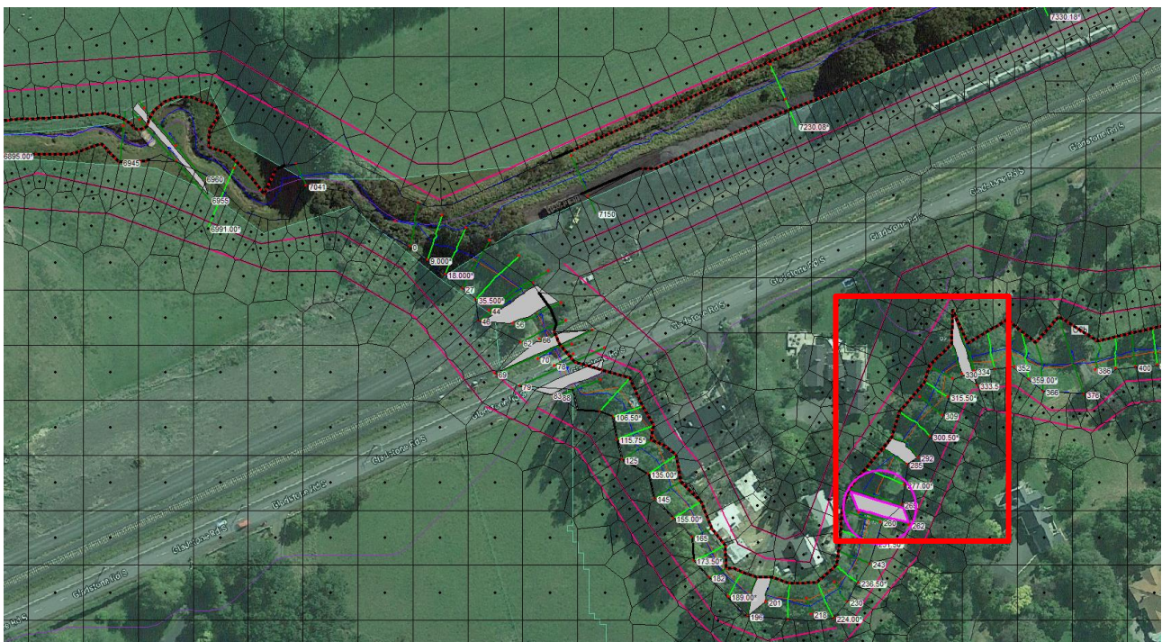
Figure 33 - Culvert "RS265" with flow shown in previous figure is circled in pink. The three culverts contained in the red outline are constriction points for Quarry Creek
