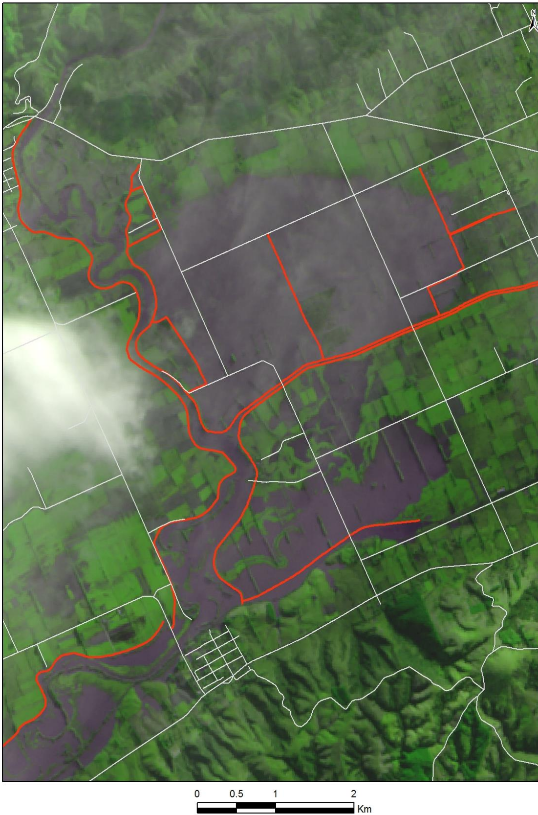
Figure 13 - Satellite imagery of July 2017 event (image taken midmorning 24 July 2017, after peak of event), provided by ORC. Red lines are stopbanks and white lines are key roads.
