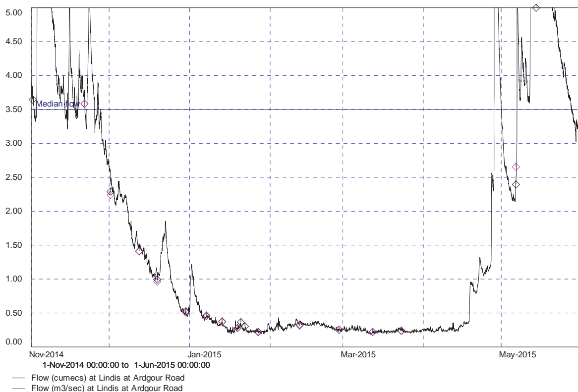
Figure 14 Instantaneous flow in the Lindis at Ardgour Road, with gauged flows overplotted (pink diamonds) for the period 1 November 2014 to 31 May 2015
