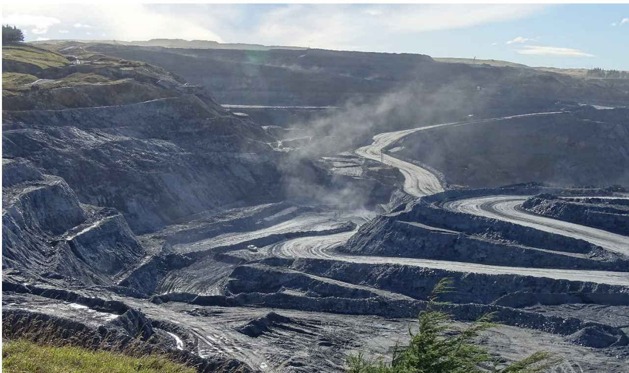
Figure 4-4. Example of dust generated from exposed surfaces by winds (Frasers West Pit)
