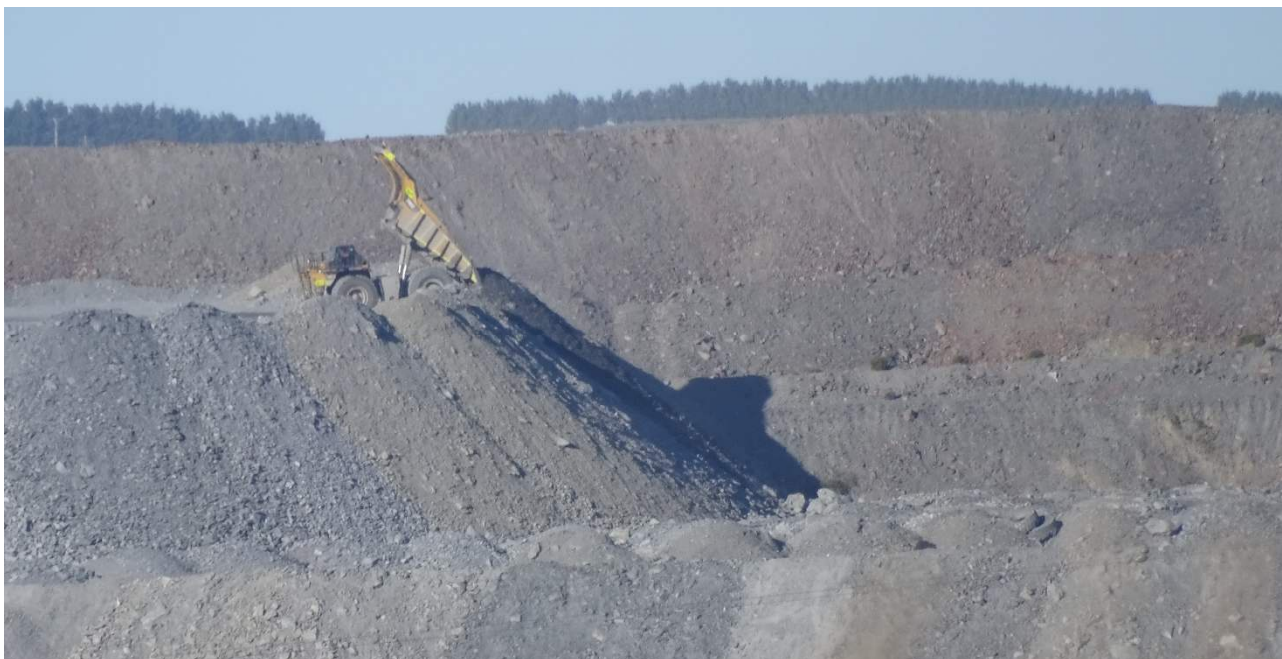
Figure 4-2. Unloading of waste rock by end tipping at Frasers West WRS
