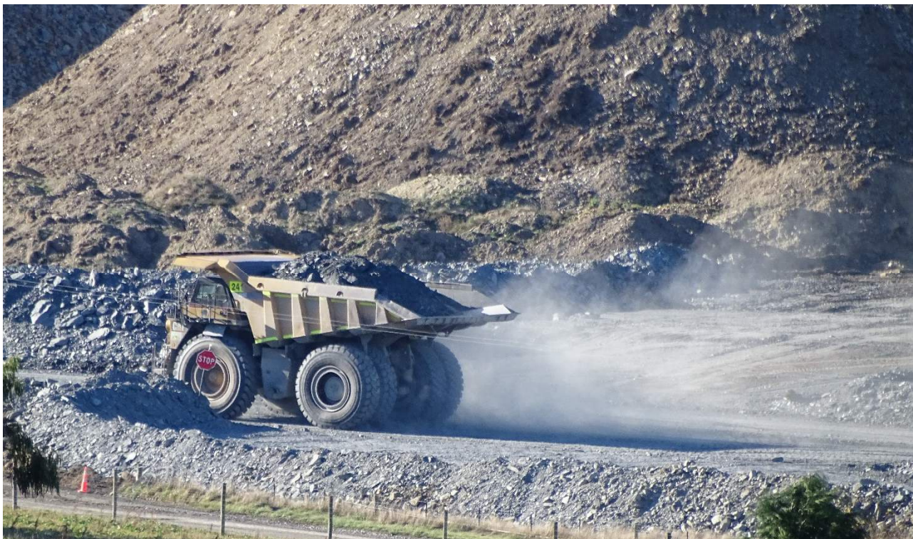
Figure 4-3. Example of dust generated by vehicle movements (note the hauled material being damp is not generating dust)
