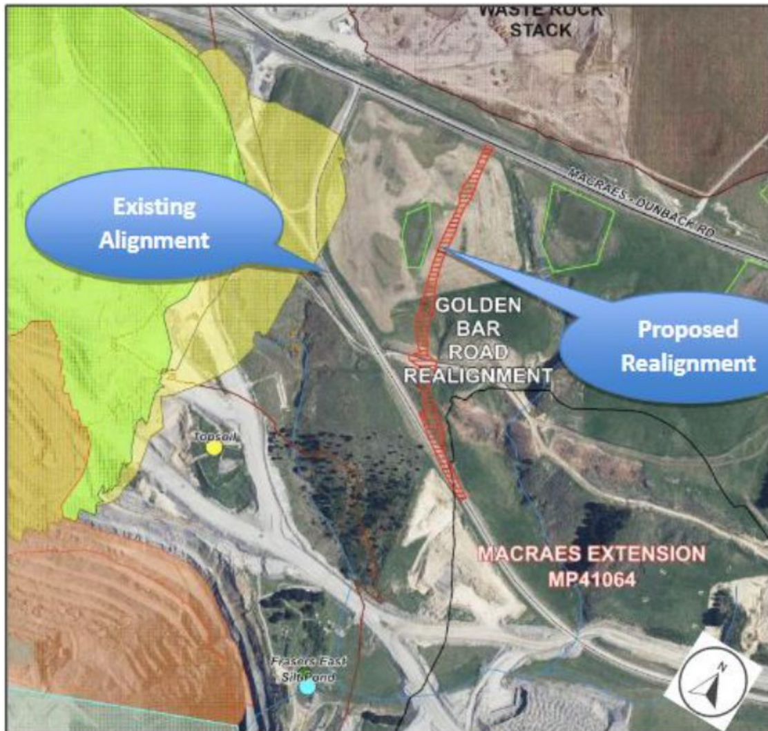
Figure 17 Proposed Golden Bar Road realignment. Wetlands are shown as green polygons. Source: RM24.184 application.
