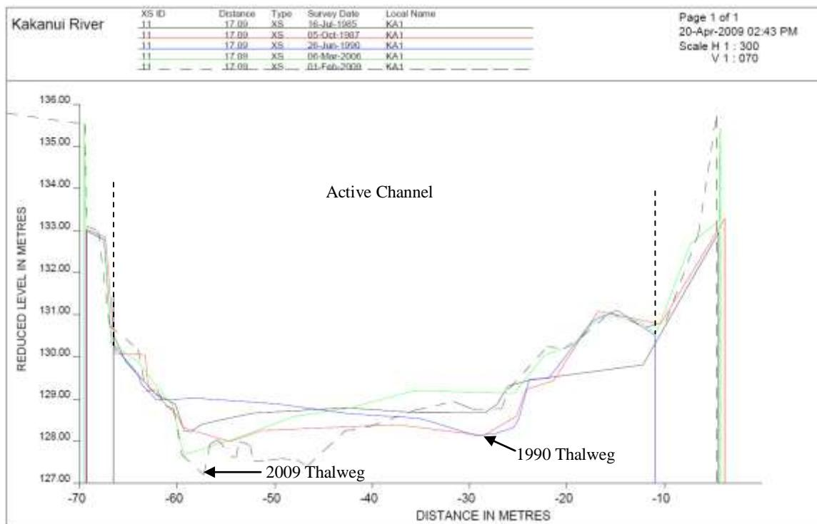
**Figure 8.11** Cross-section KA1, looking downstream.
