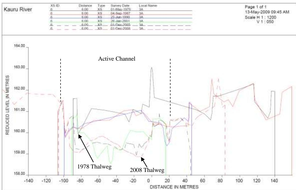
**Figure 8.30** Cross-section K3A, looking downstream.
