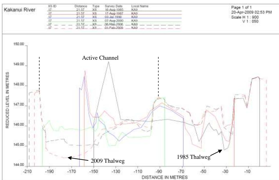
Figure 8.17 Cross-section KA9, looking downstream.
