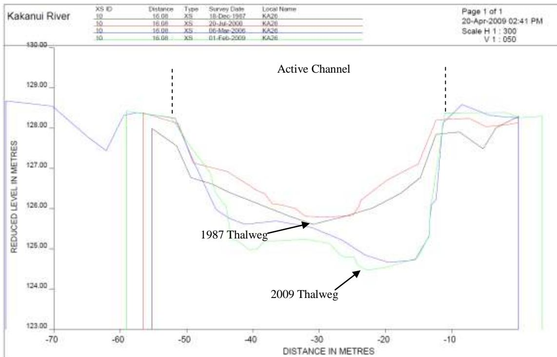
Figure 8.10 Cross-section KA26, looking downstream.
