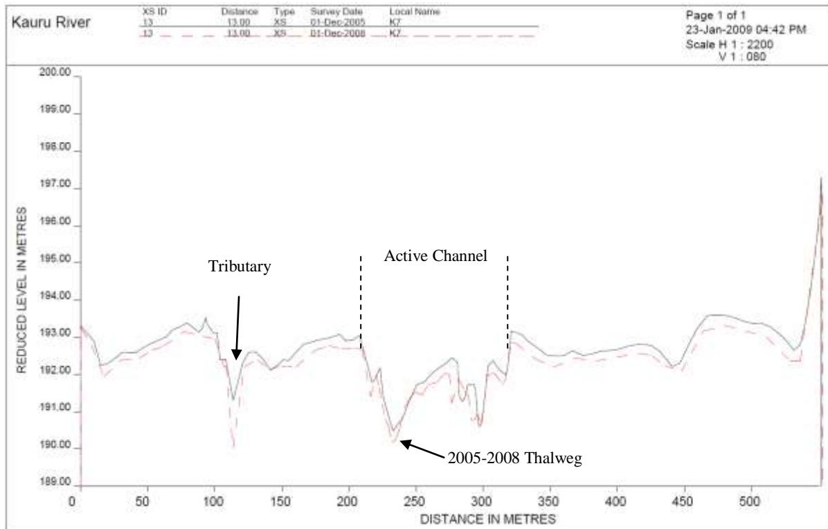
**Figure 8.36** Cross-section K7, looking downstream.
