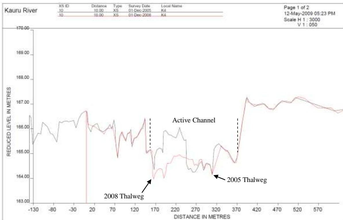
**Figure 8.32** Cross-section K4, looking downstream.
