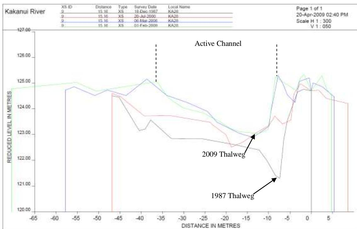
**Figure 8.9** Cross-section KA28, looking downstream.
