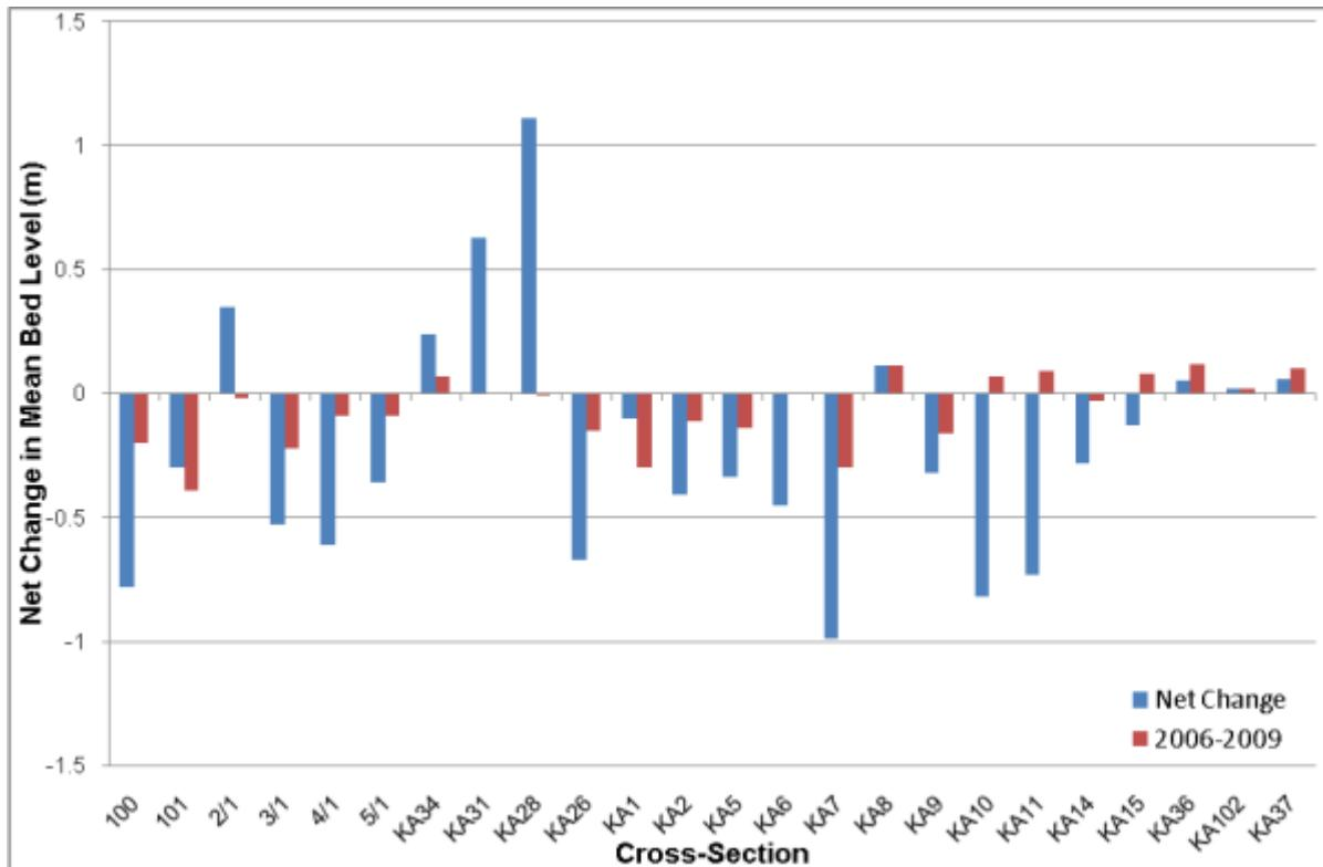
Figure 3.2 Graph showing net change in mean bed level across all survey periods and between the last two surveys (2006 and 2009) for each cross-section.
