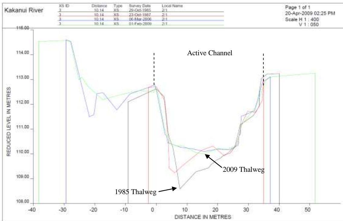
**Figure 8.3 Cross-section 2/1, looking downstream.**
