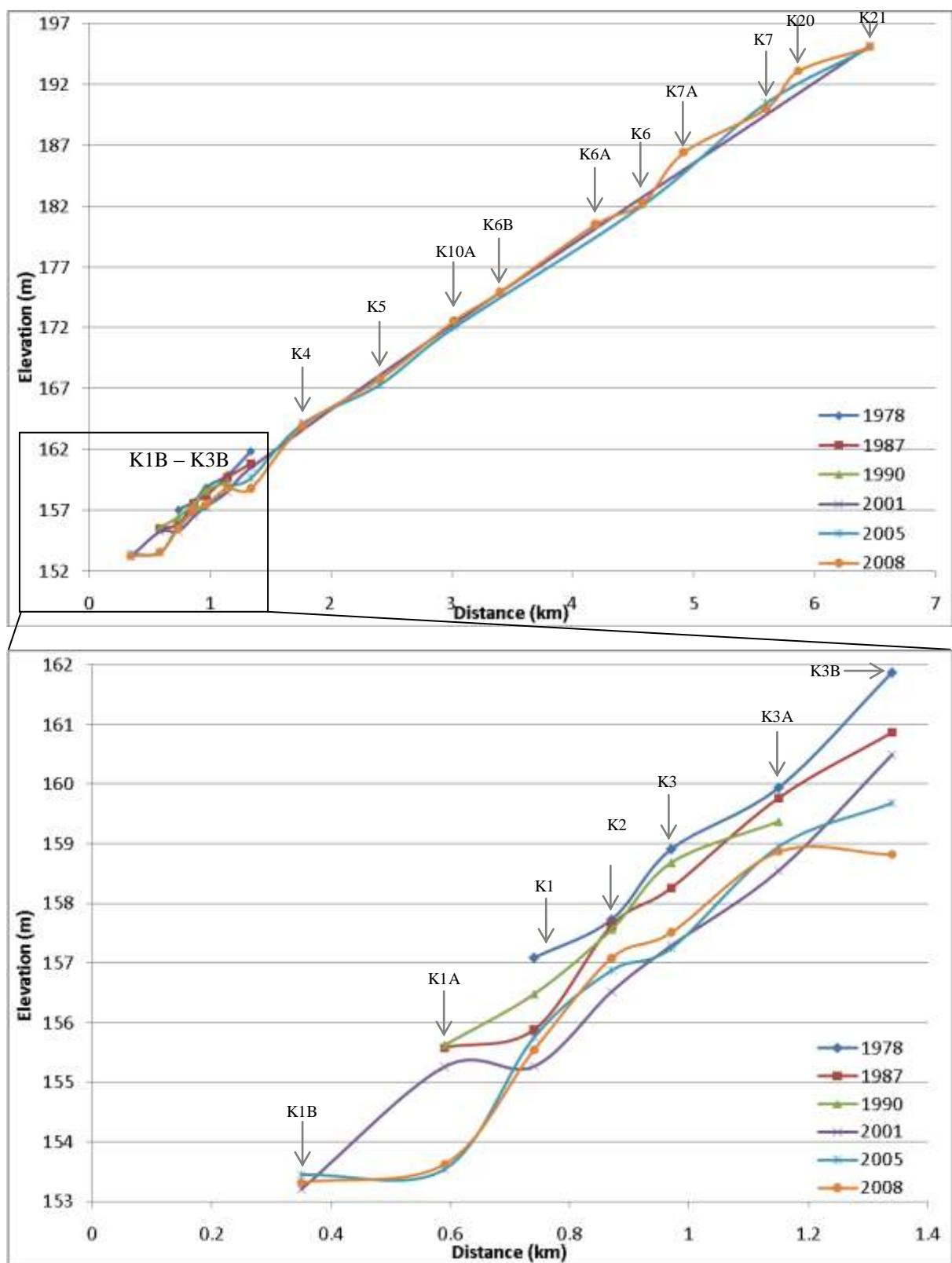
Figure 4.2 Longitudinal profile of the Kauru River, using minimum bed level. The river mouth is at 0km distance.
