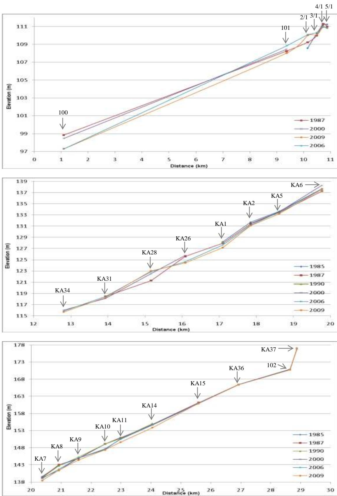
Figure 4.1 Longitudinal profile of the Kakanui River using minimum bed level. The river mouth is at 0km distance.
