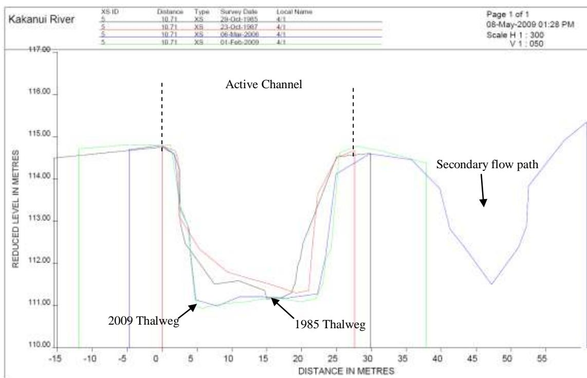
**Figure 8.5** Cross-section 4/1, looking downstream.
