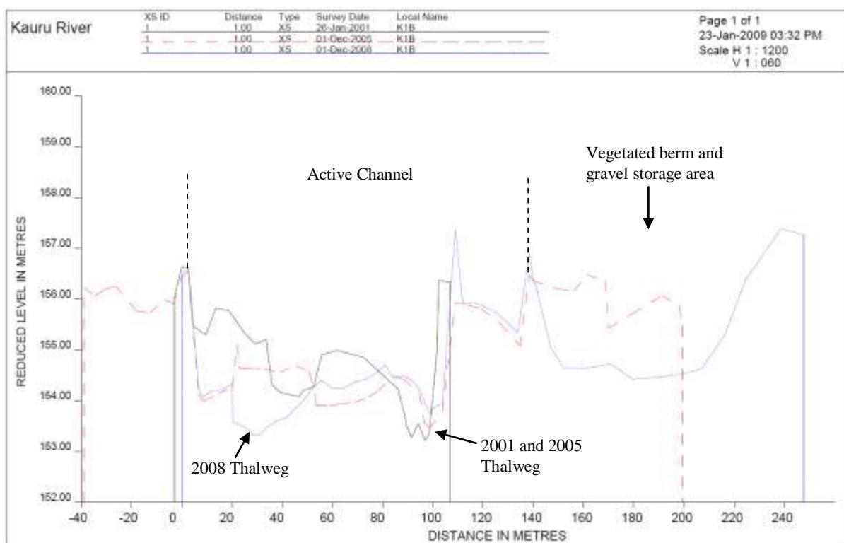
**Figure 8.25** Cross-section K1B, looking downstream.
