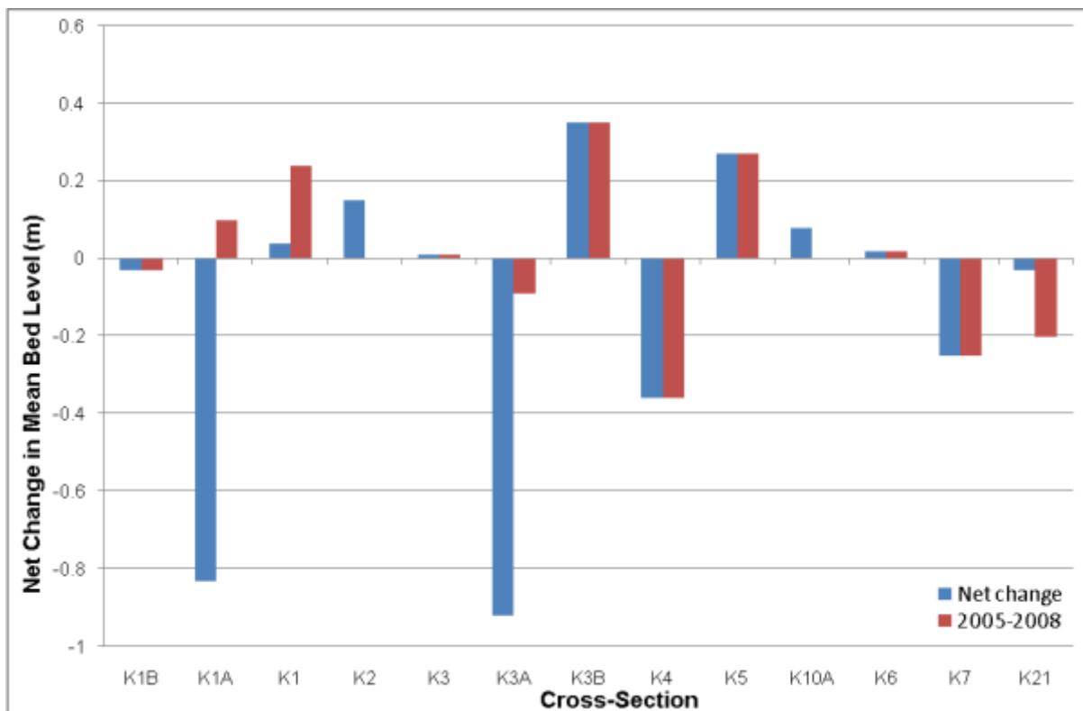
Figure 3.4 Graph showing net change in mean bed level across all survey periods and between the last two surveys (2005 and 2008) for each cross-section.
