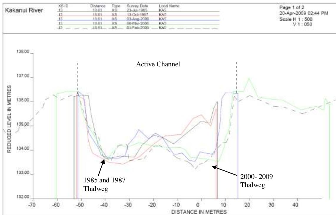
Figure 8.13 Cross-section KA5, looking downstream.
