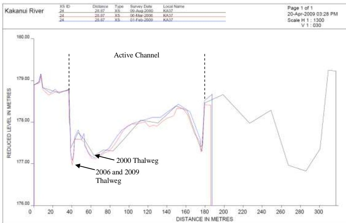
**Figure 8.24** Cross-section KA37, looking downstream.
