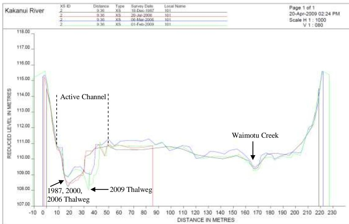
**Figure 8.2** Cross-section 101, looking downstream.
