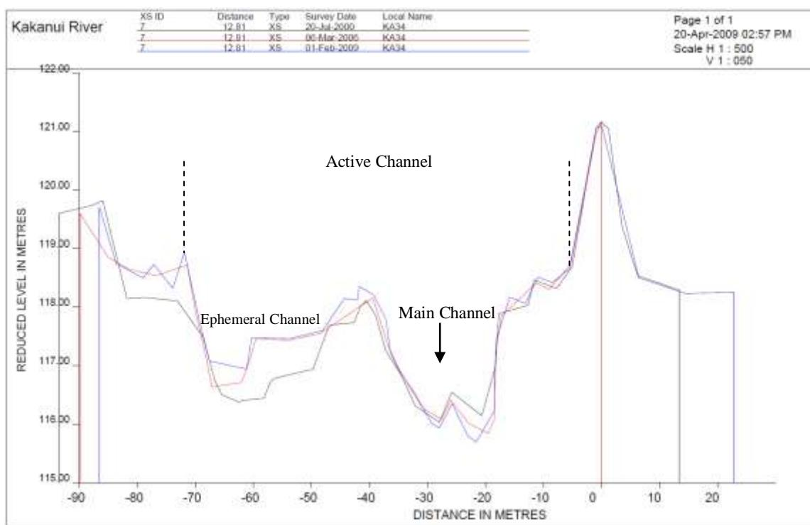
**Figure 8.7** Cross-section KA34, looking downstream.
