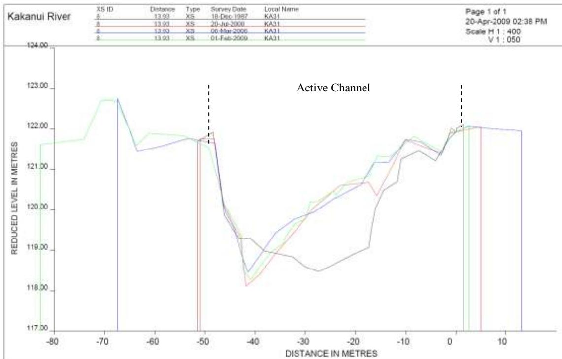
**Figure 8.8** Cross-section KA31, looking downstream.
