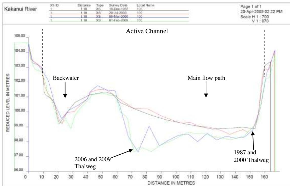
**Figure 8.1** Cross-section 100, looking downstream.
