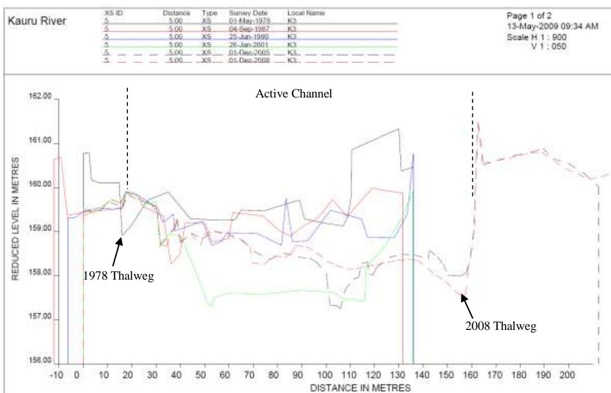
Figure 8.29 Cross-section K3, looking downstream.
