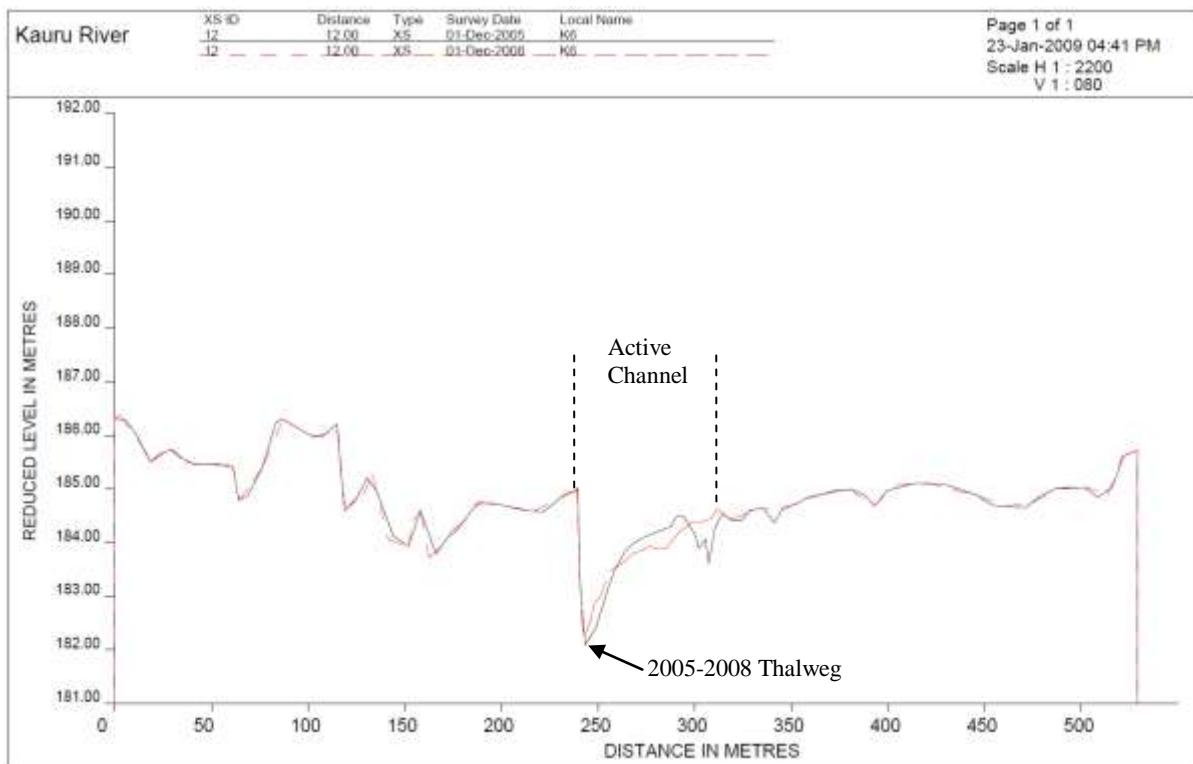
**Figure 8.35** Cross-section K6, looking downstream.
