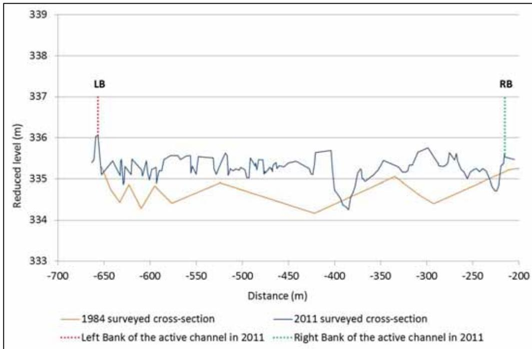
Figure 23 The earliest and most recent cross-section surveys at RR12, upstream of the Rees River Bridge
