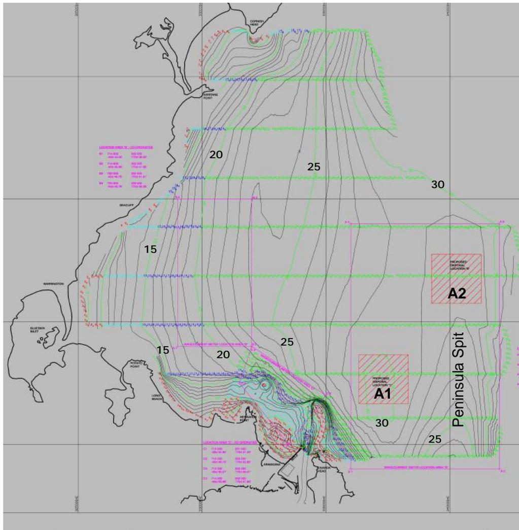
**Figure 2.5** POL seabed sounding lines (2 km spacing offshore) and contours at 1 m increments and annotated every 5 m increments (m; Chart Datum), illustrating the bathymetry coverage within Blueskin Bay and the inner shelf. The hatched squares (A1, A2) indicate initial site options considered for placement of dredged sediment (Source: Figure 3.1 Bell *et al.* 2009).
