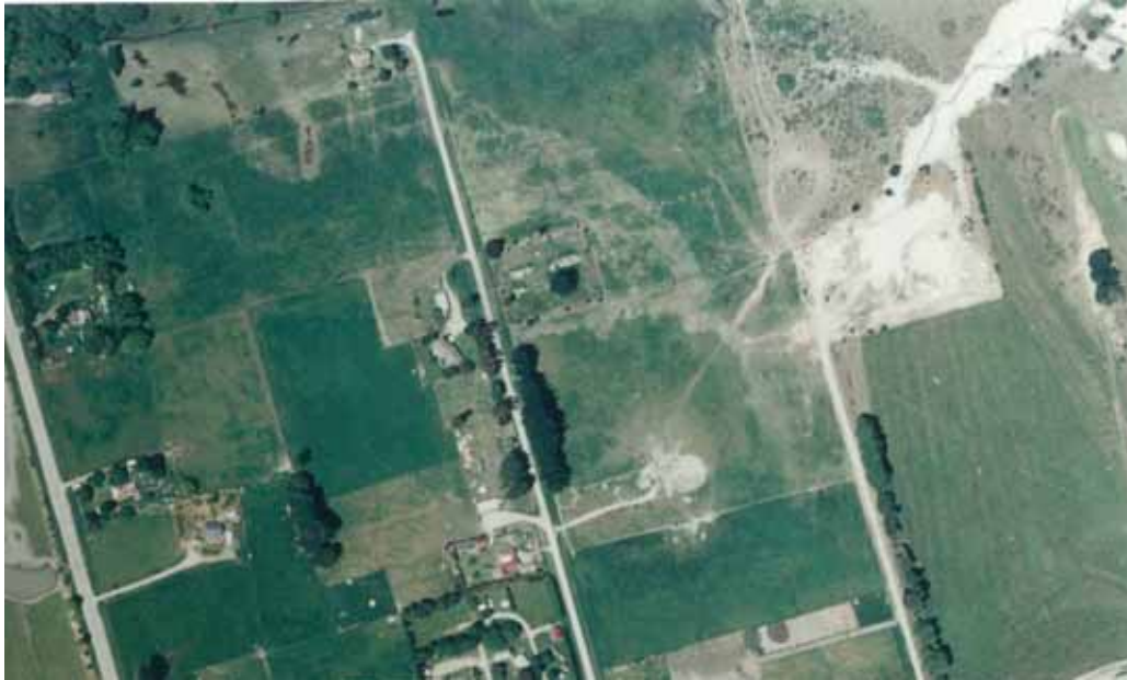
Figure 3.17 Sedimentation resulting from the November 1999 flood event across the Bible Stream alluvial fan
