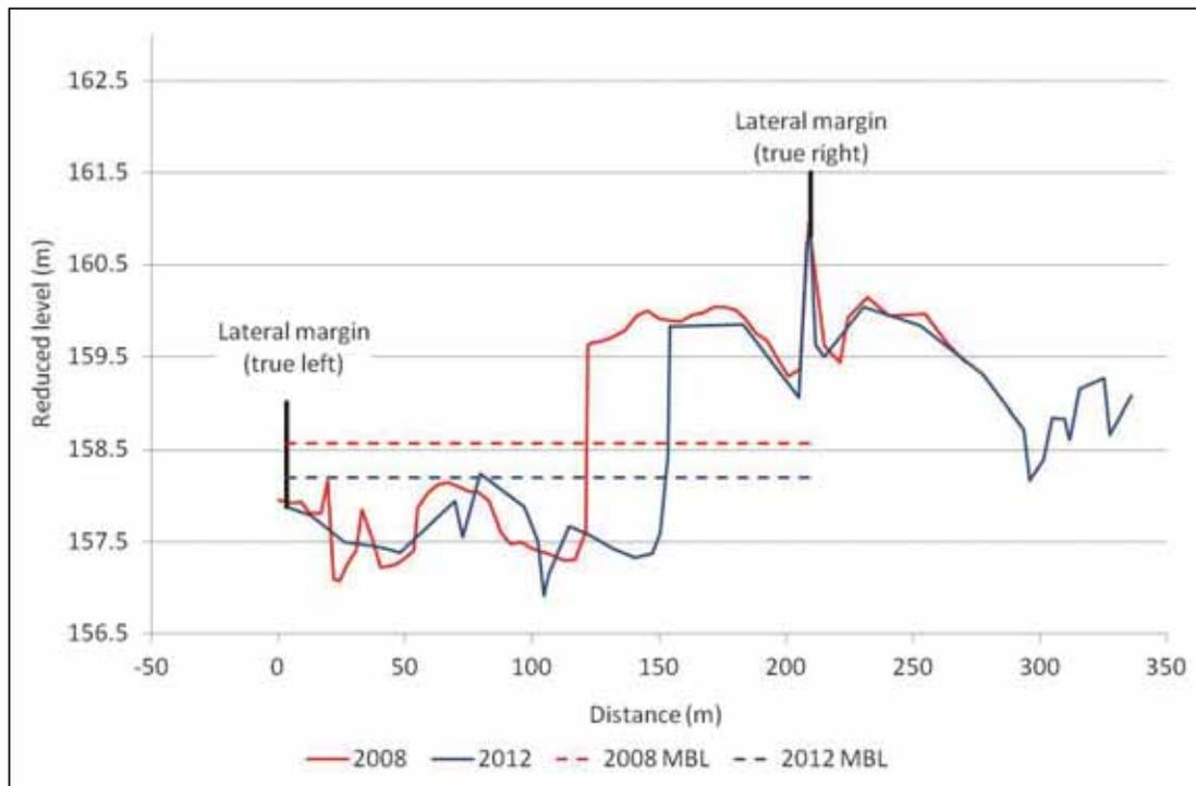
**Figure 39.** Change in the MBL at a cross-section. The MBL was calculated for that part of the channel within the true-left and true-right lateral margins.
