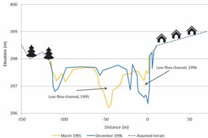
**Figure 8. Cross-section 3 showing migration of the main channel towards the true right between March 1995 and December 1996**
