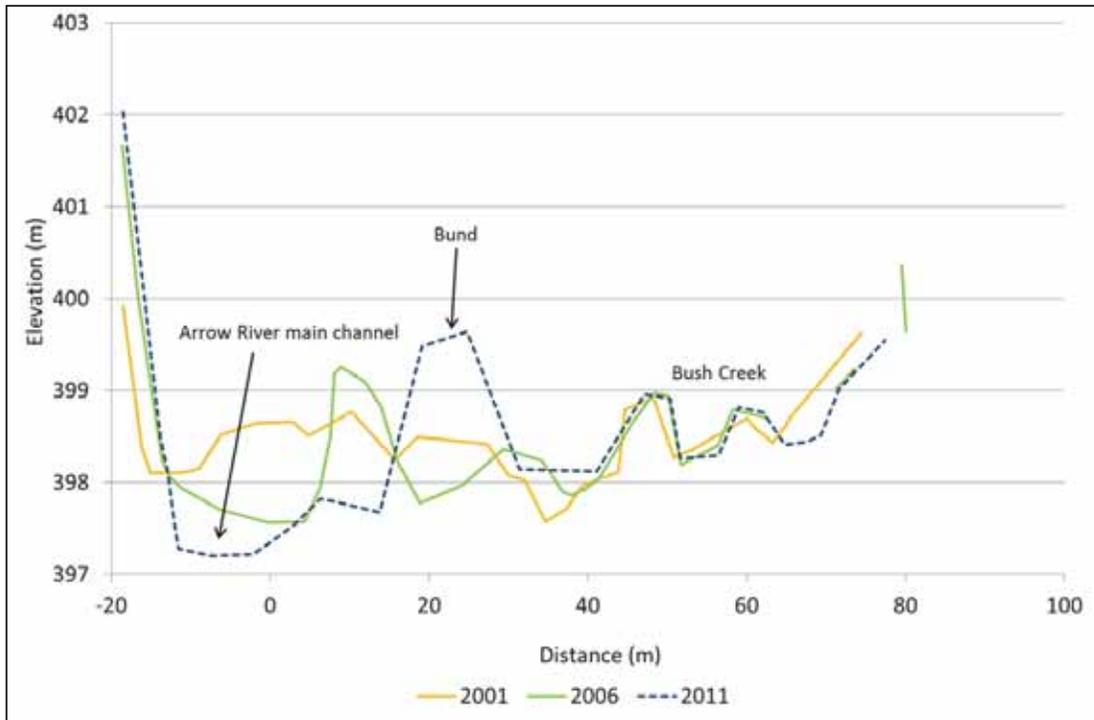
**Figure 26.** Cross-section 3/1, looking downstream, showing data from the three most recent surveys
