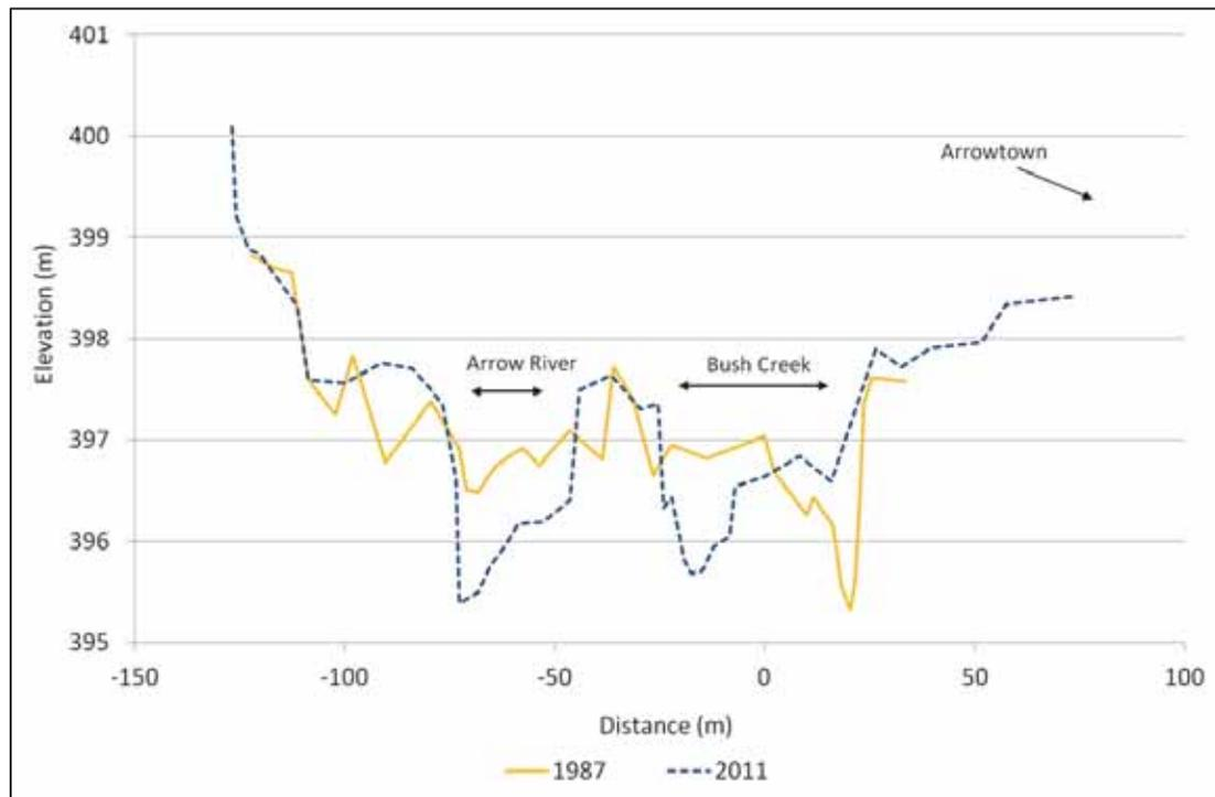
Figure 32. Cross-section 2/3, looking downstream, showing first (1987) and last (2011) survey data
