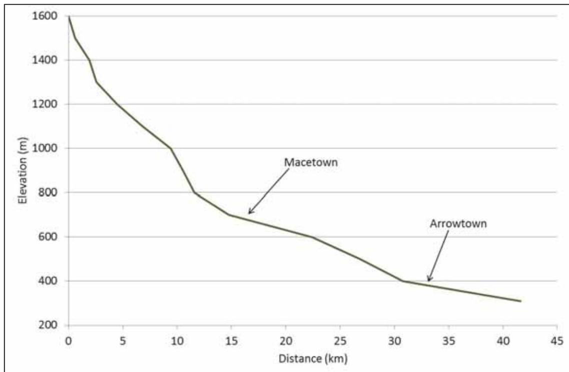
**Figure 5. Longitudinal profile of the Arrow River (estimated from LINZ 1:50,000 topographical maps, F40, F41)**
