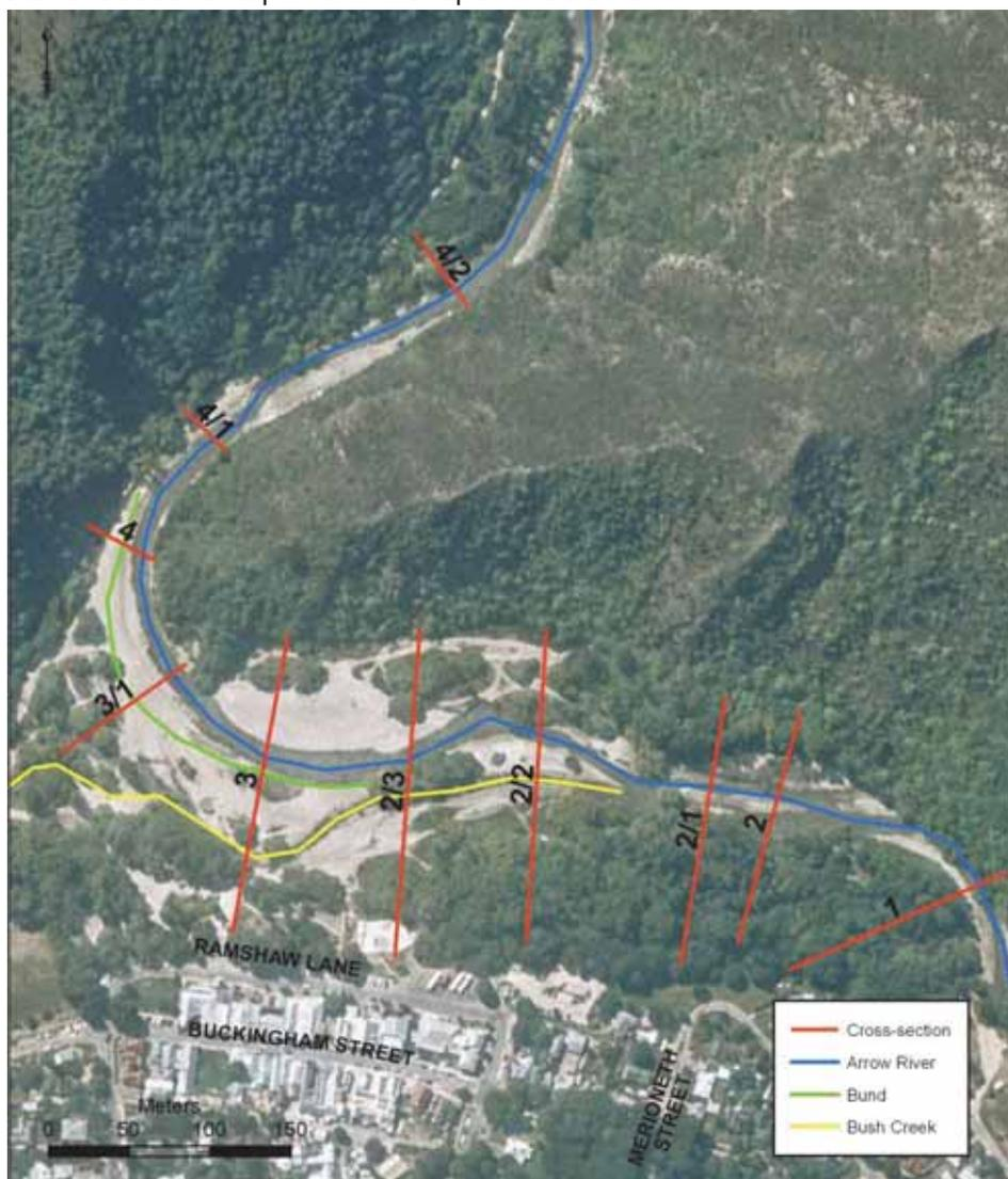
**Figure 1.** Location of Arrow River cross-sections. These were established in 1987 and sections 4 to 2/2 were most recently surveyed in 2011 (Appendix 2).
