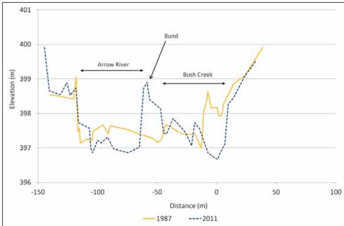
Figure 28. Cross-section 3, looking downstream, showing first (1987) and last (2011) survey data
