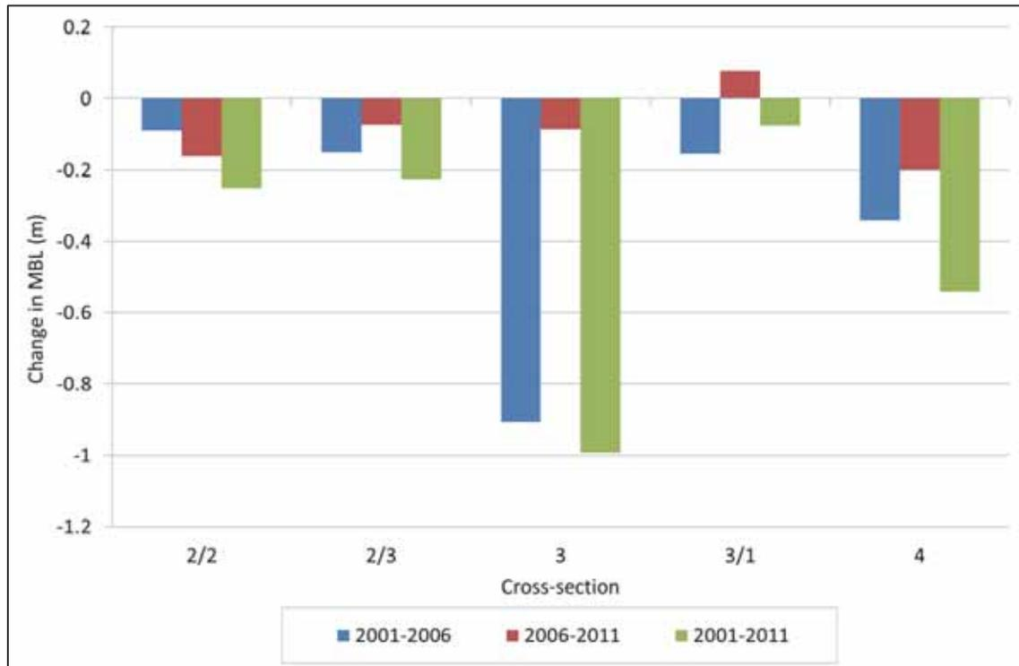
Figure 19. Change in MBL between Jan. 2001 and Nov. 2006 and Nov. 2006 and Nov. 2011. The net change in MBL over the entire period is also shown.
