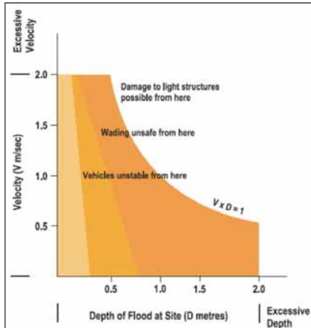
Figure 18. Example of flood-hazard classification, based on the product of the velocity and depth (NSW Government, 2005)
