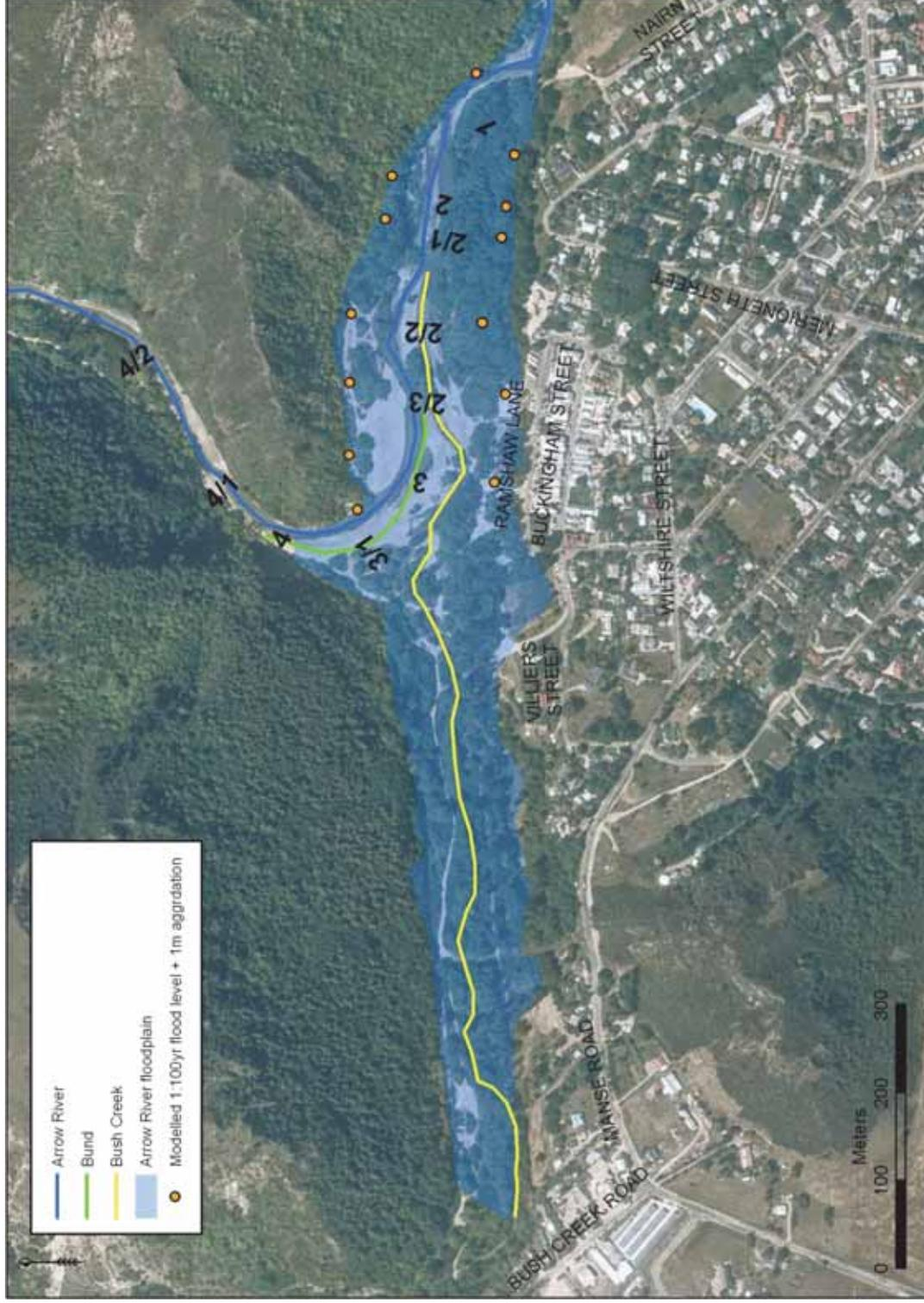
Figure 12. Arrow River/Bush Creek floodplain area, and the extent of the modelled 1:100-year flood level at each cross-section location
