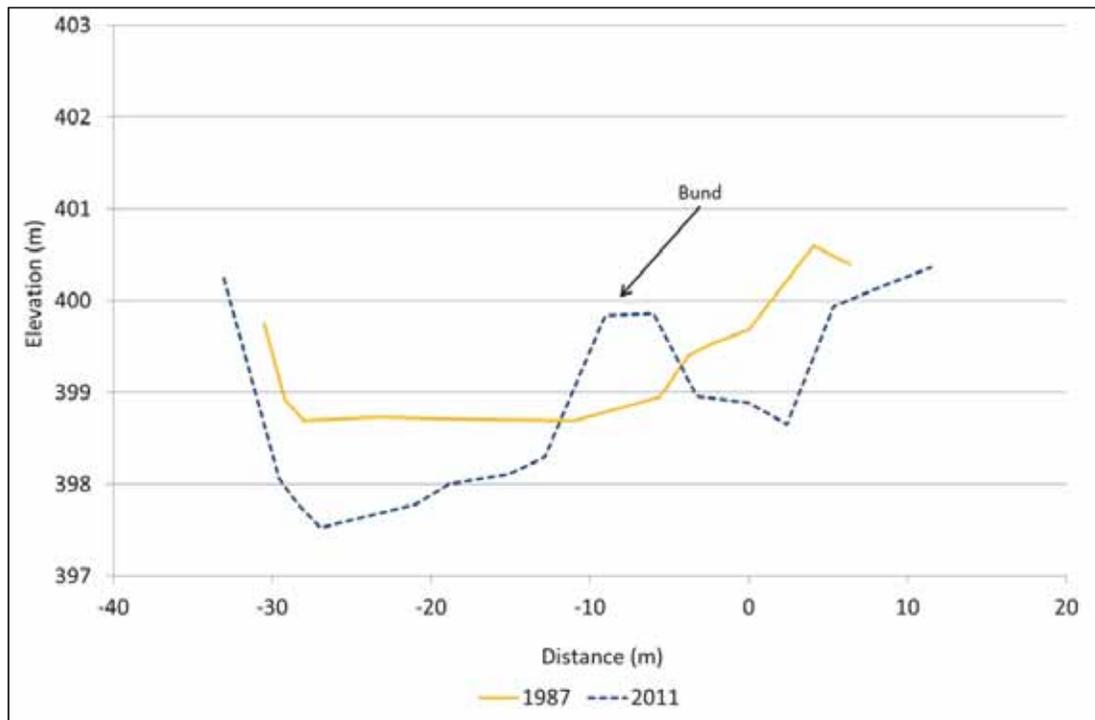
Figure 20. Cross-section 4, looking downstream, showing first (1987) and last (2011) survey data
