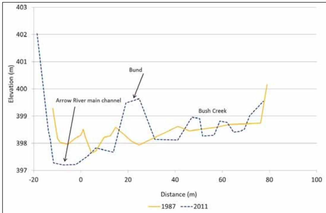
Figure 24. Cross-section 3/1, looking downstream, showing first (1987) and last (2011) survey data
