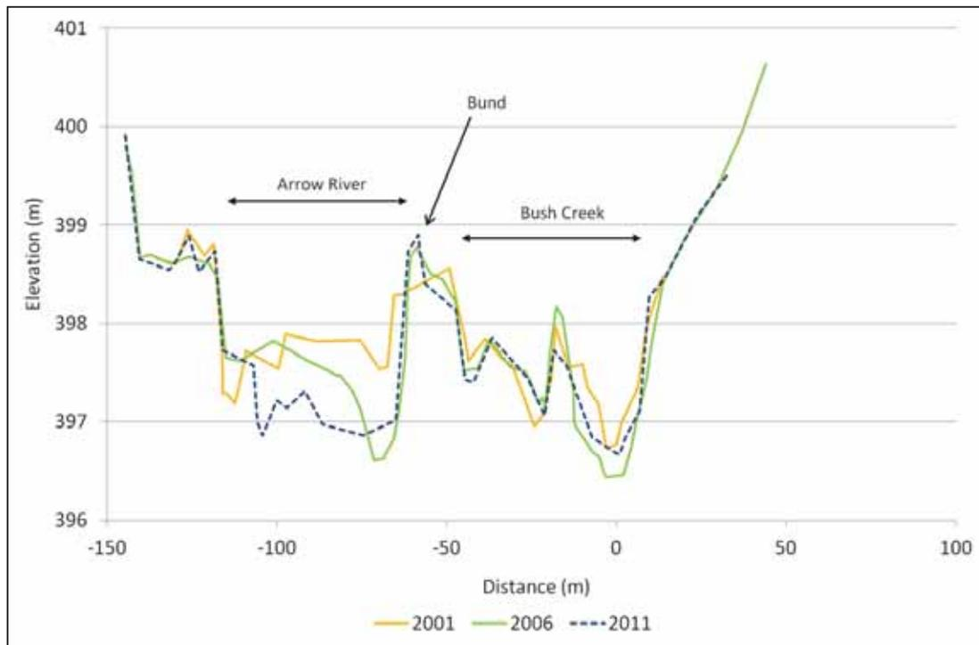
Figure 30. Cross-section 3, looking downstream, showing data from the three most recent surveys
