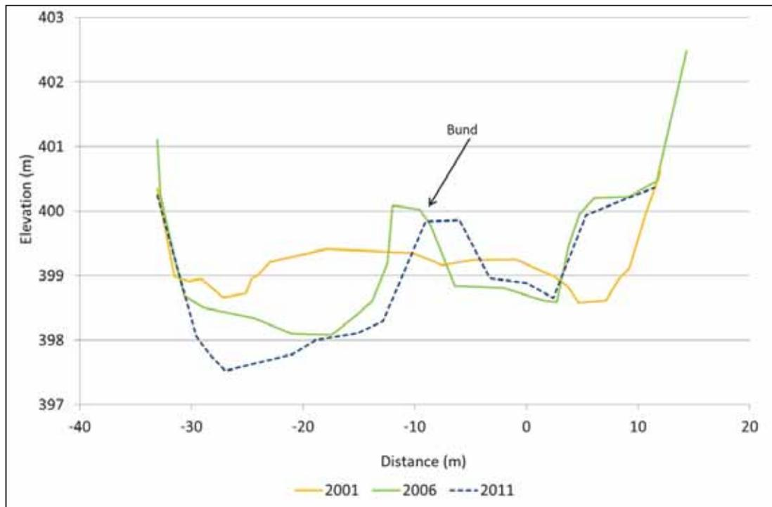
Figure 22. Cross-section 4, looking downstream, showing data from the three most recent surveys
