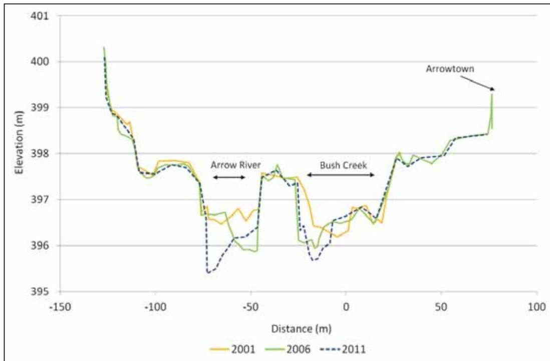
**Figure 34. Cross-section 2/3, looking downstream, showing data from the three most recent surveys**
