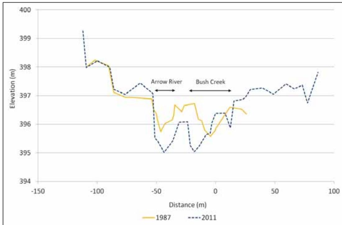
Figure 35. Cross-section 2/2, looking downstream, showing first (1987) and last (2011) survey data
