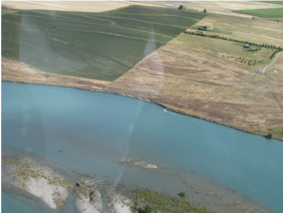
Figure 21. View of the Clutha River/Mata-Au, looking downstream and showing erosion of the true left bank, downstream of the Lindis confluence (point 3 on Figure 15). Photo taken 15 January 2013.
