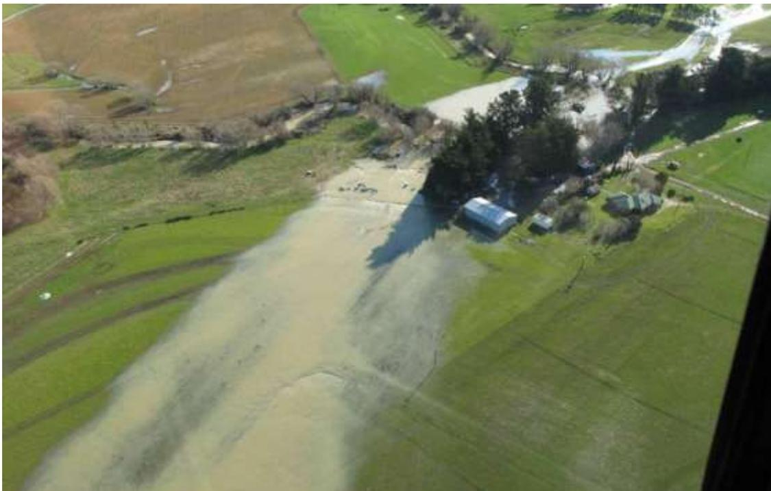
**Figure 4. Avulsion of the Hororata River following fault movement during the September 2010 Darfield earthquake (photo courtesy D. Barrell, GNS Science)**
