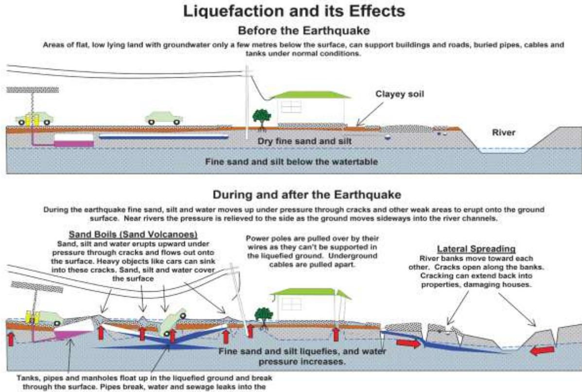
Figure 5. Effects of liquefaction (from IPENZ factsheet)
