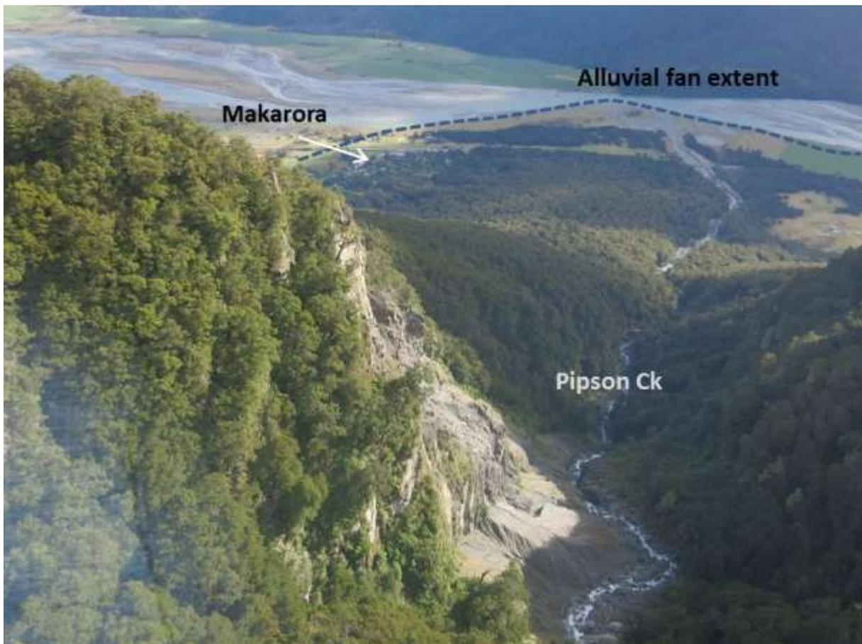
**Figure 30. View down Pipson Creek, near Makarora (May 2015). The eroding cliffs in the foreground (and other cliffs upstream) contribute rock and sediment to the channel, which can mobilise into debris flows during high rainfall. Earthquake shaking is liable to cause extensive rockfall and landsliding into the creek.**
