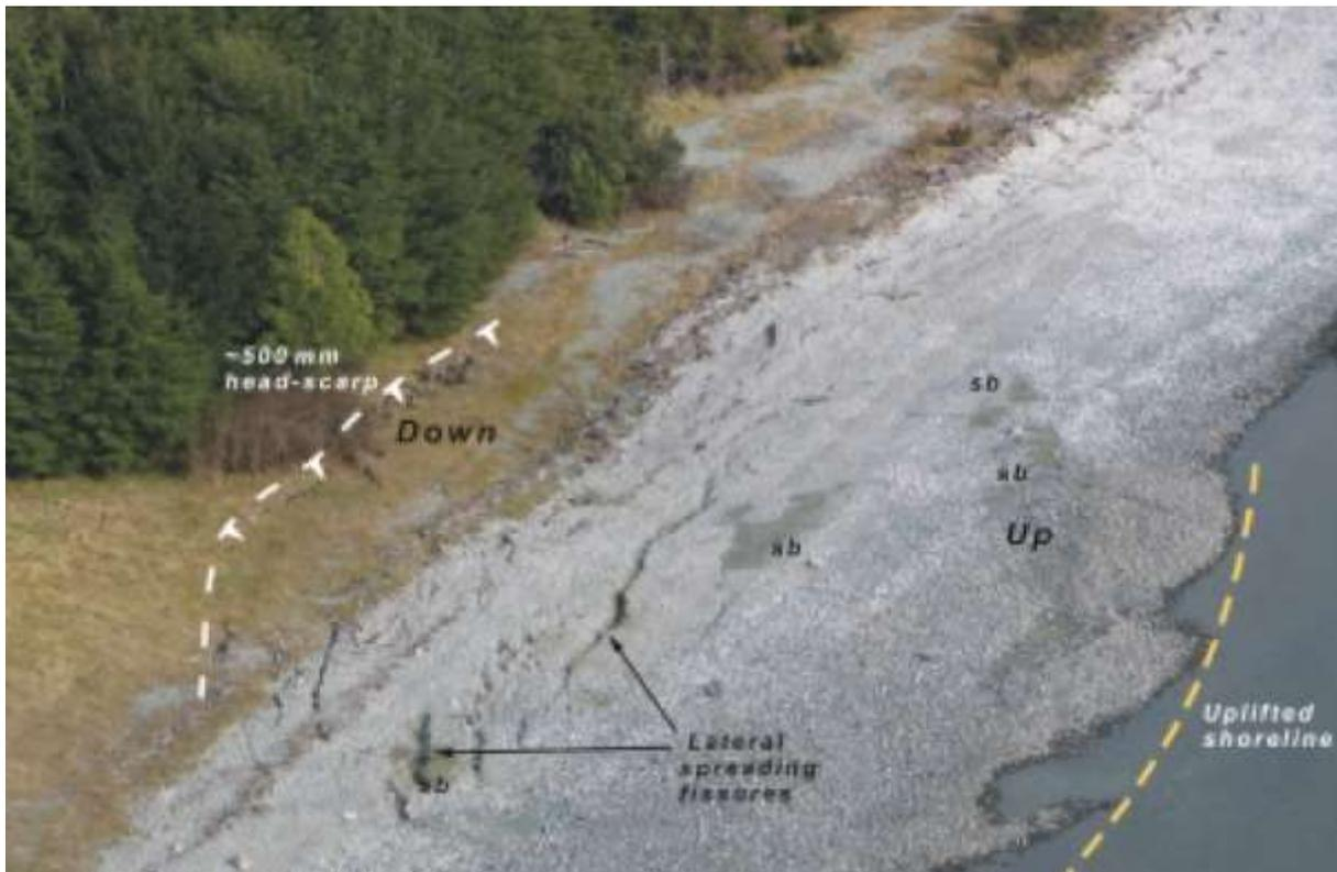
**Figure 7. Lake-edge failure along Lake Te Anau during the 2003 Fiordland earthquake (Hancox *et al.*, 2003). This failure incorporated liquefaction and lateral spreading of the lake-beach area.**
