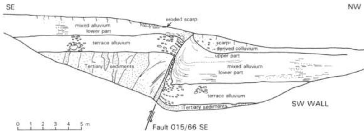
**Figure 21. Diagram of a trench wall cut through active section of a splay of the northern Cardrona Fault, just south of MacDonaldis Creek (6 km north of Cardrona village). The ~18,000 year old alluvial terrace deposit (terrace alluvium layer) has been offset by 4 m vertically, by at least three recognised earthquakes (from Beanland and Barrow-Hurlbert, 1988).**
