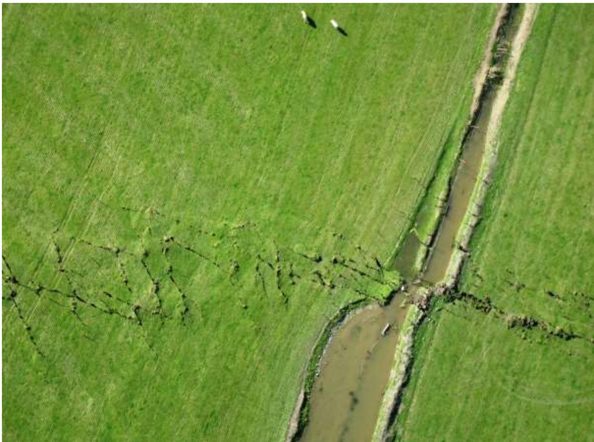
**Figure 1.** The surface trace of the Greendale Fault rupture cut across paddocks in the Canterbury Plains in September 2010 (photo courtesy M. Quigley). The ground moved up to 5.3 m laterally, but was expressed at the surface as a zone of distributed deformation up to 300 m wide, as seen in the network of shear structures (Quigley *et al.*, 2012).
