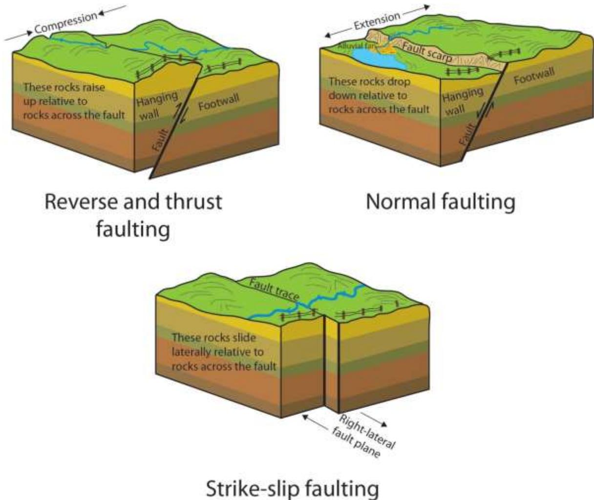
**Figure 2. The main styles of faulting. Faults in western Otago are primarily reverse faults, reflecting the regional compression, whereas the Alpine Fault is a predominantly a strike-slip fault (from USDA National Park Service).**
