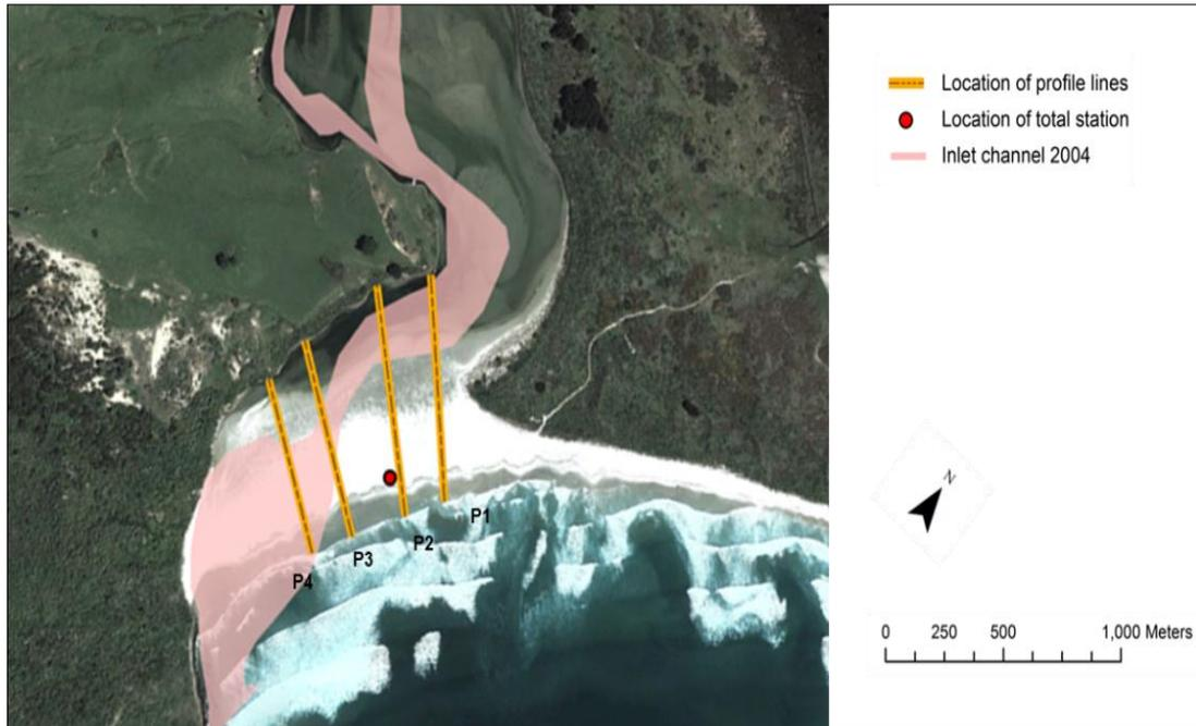
Figure 4. Location of the surveyed shore normal profiles surveyed in March relative to the existing spit and the tidal inlet in 2004.
