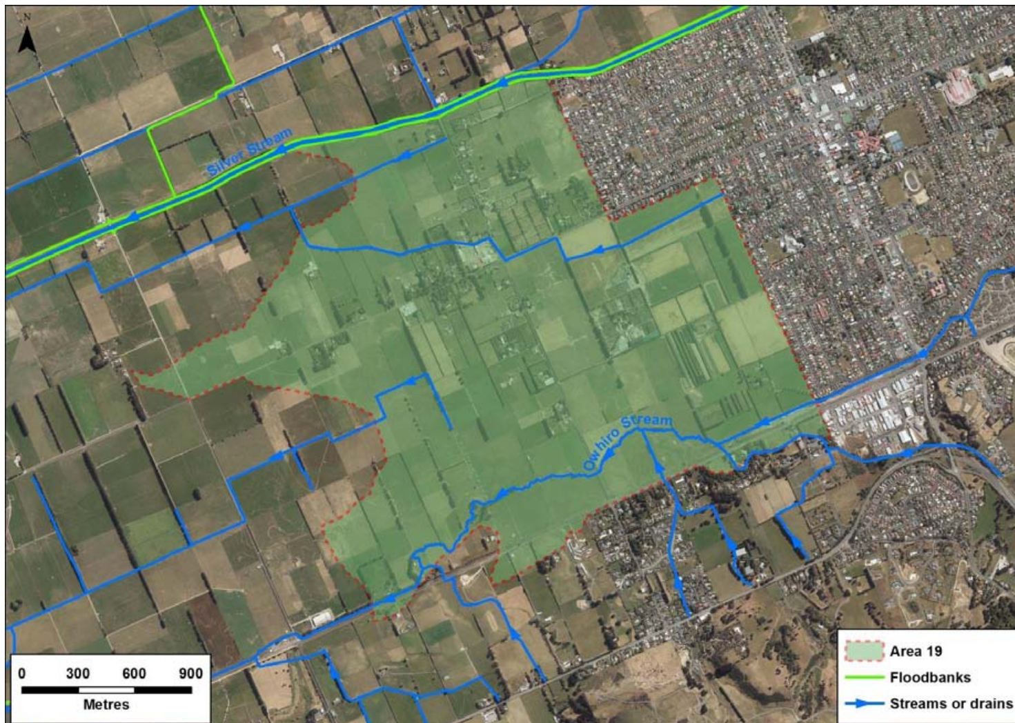
Figure 27 Area 19 – Streams and drains and general direction of flows in Area 19
