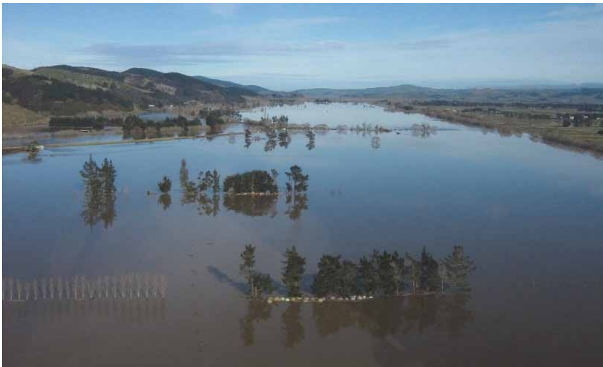
Figure 25. Lower Taieri floodway, looking downstream to Henley, 31 July 2007. Several rows of trees and balage lie perpendicular to the direction of flow.
