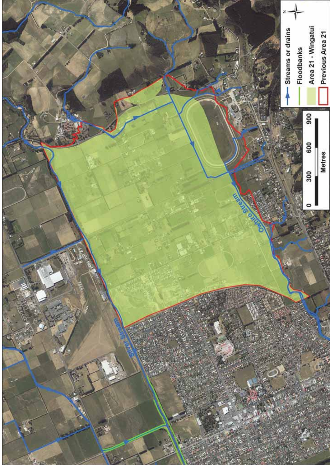
Figure 55. Area 21 Streams and drains and general direction of flows in Area 21. The previous extent of this area is also shown.
