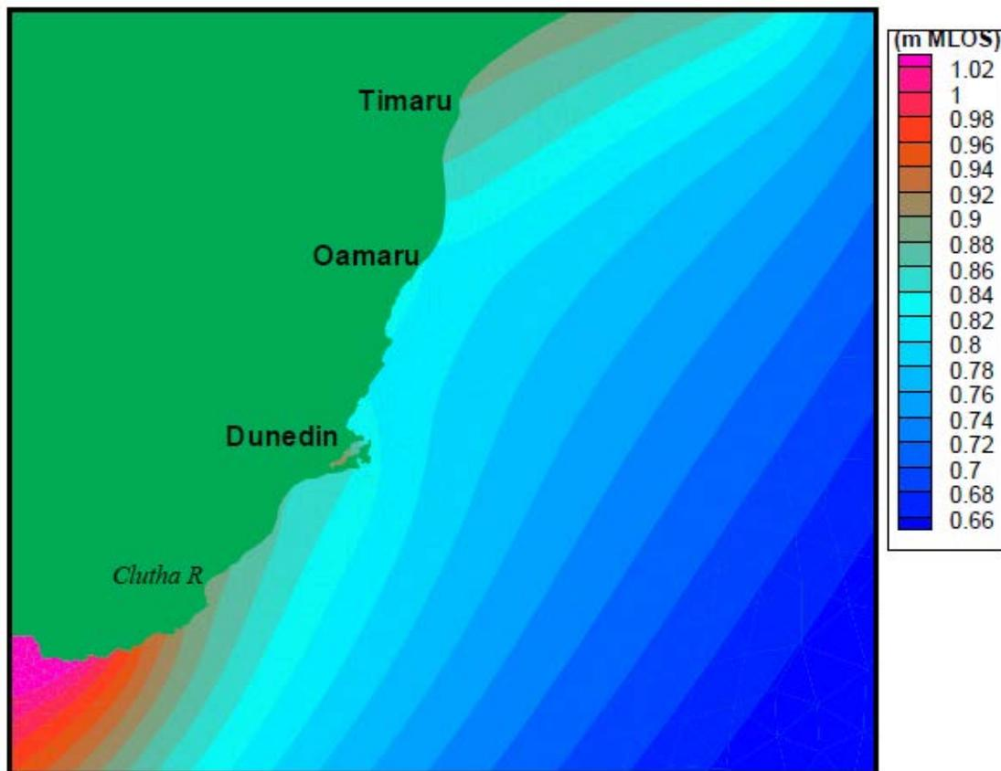
Figure 3. Distribution of MHWS level in Otago waters. Levels are shown in metres above mean level of the sea (MLOS), based on a tidal model of New Zealand. (Image from NIWA, 2008)
