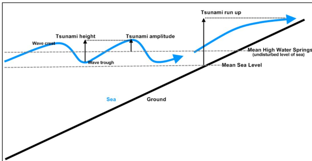
Figure 4. Diagram showing tsunami-wave amplitude and run-up. Amplitude is measured relative to the undisturbed level of the sea (which is MHWS, for the purpose of this report), while wave run-up is measured relative to MSL
