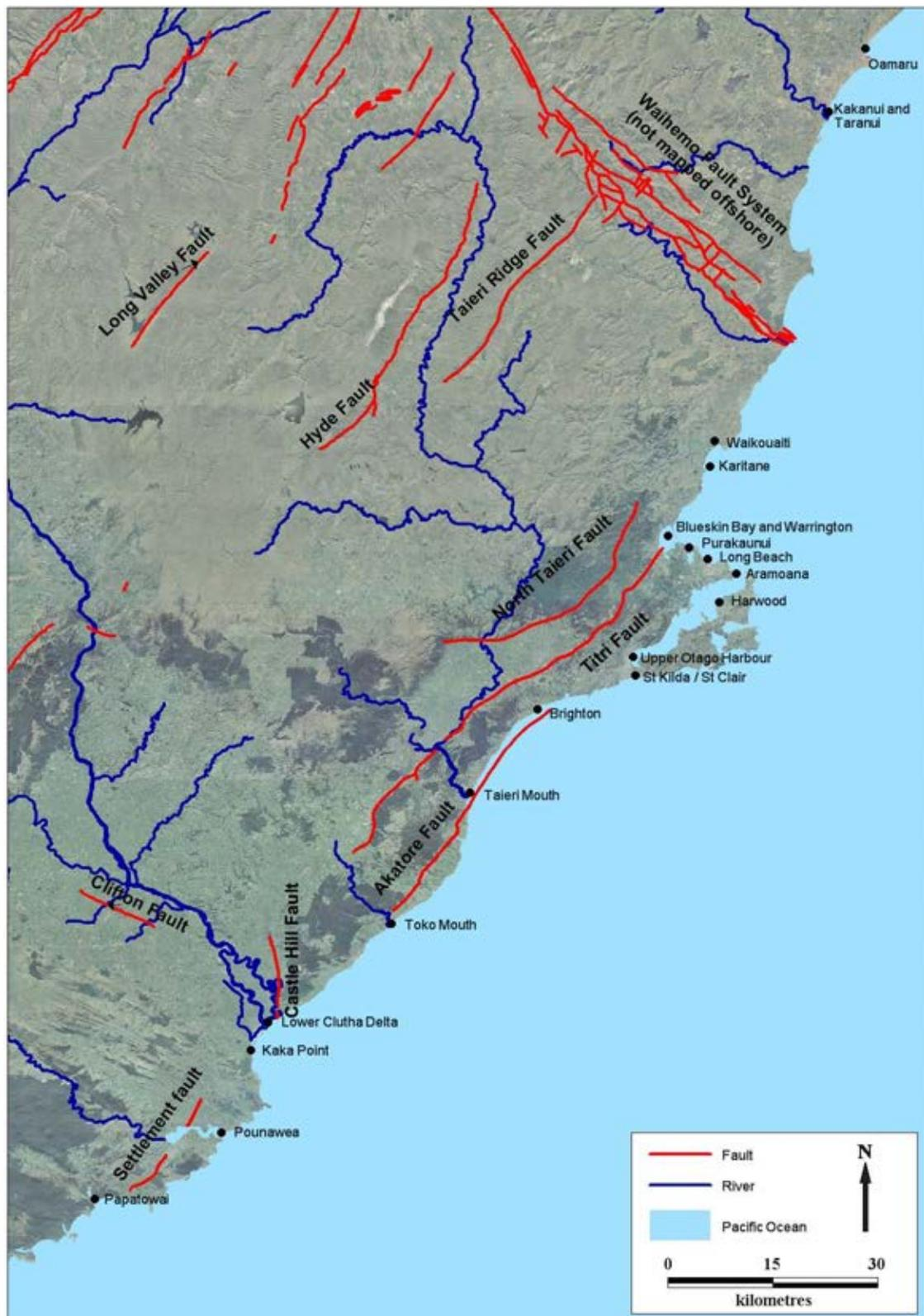
Figure 6. Location of mapped active faults in eastern Otago<sup>26</sup> and the location of coastal communities included in this report
