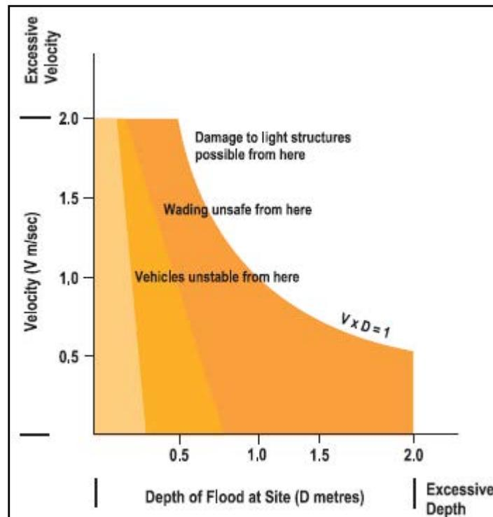
**Figure 2.** Hazard standard for water velocity and depth relationship (NSW Floodplain Development Manual, 2005). Note that this relationship has been derived from laboratory testing and observations of flood conditions that caused damage
