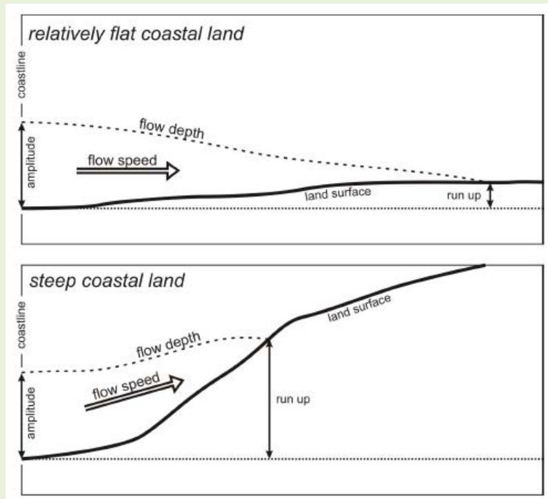
The topography of land next to the coast will affect the distance a tsunami event will travel inland and the maximum run-up height. The diagram above shows that, for gently sloping topography, the run-up may be minimal, even though the tsunami impacts (resulting from other characteristics such as wave velocity, debris accumulation and subsequent backwash) can be huge. For steep slopes, the run-up will be greater (Figure from Saunders *et al.*, 2011).
