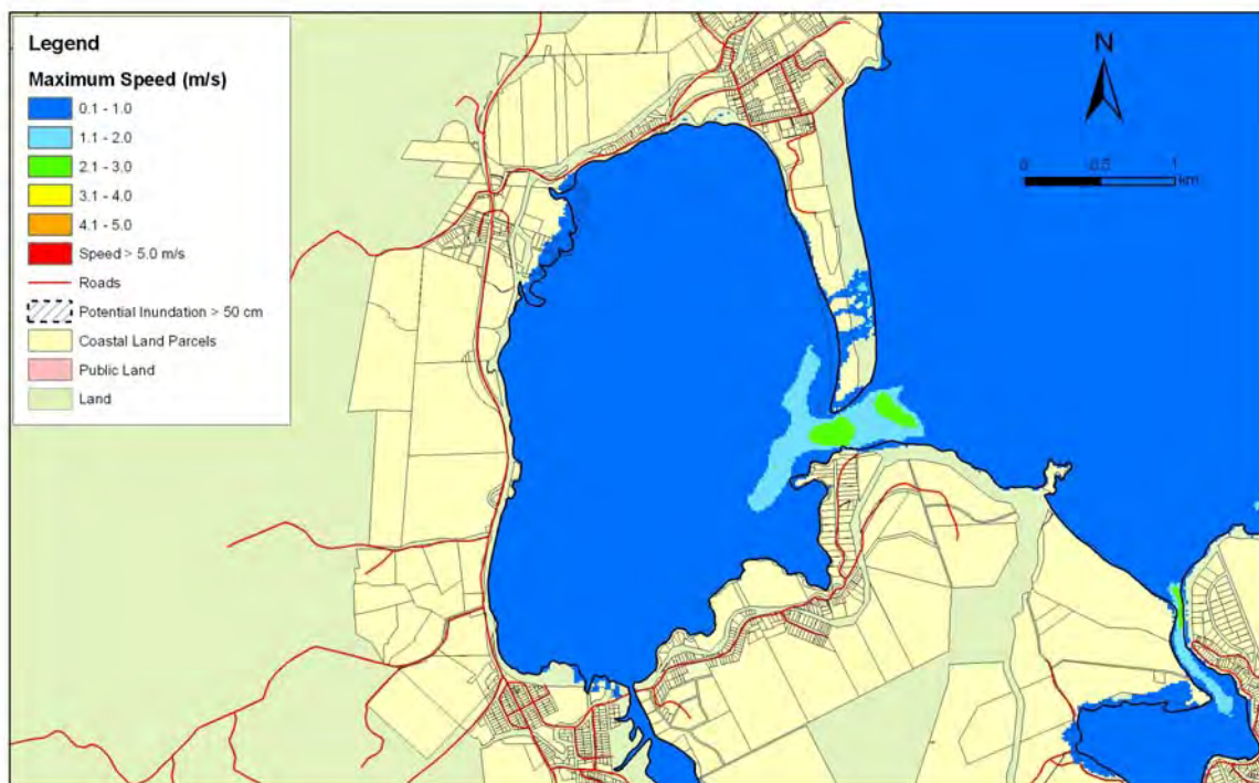
Figure 5.112: Warrington and Blueskin Bay – 1:100 year remote tsunami: Maximum water depth for inundated land (top) and maximum speed (bottom) for MHWS.
