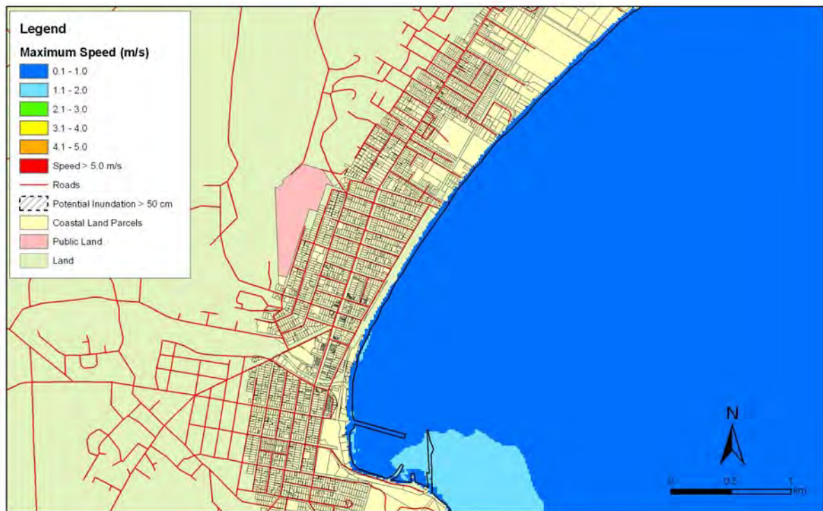
Figure 5.155: Oamaru – Puysegur tsunami: Maximum water depth for inundated land (top) and maximum speed (bottom) for MHWS with a sea level rise of 30 cm.
