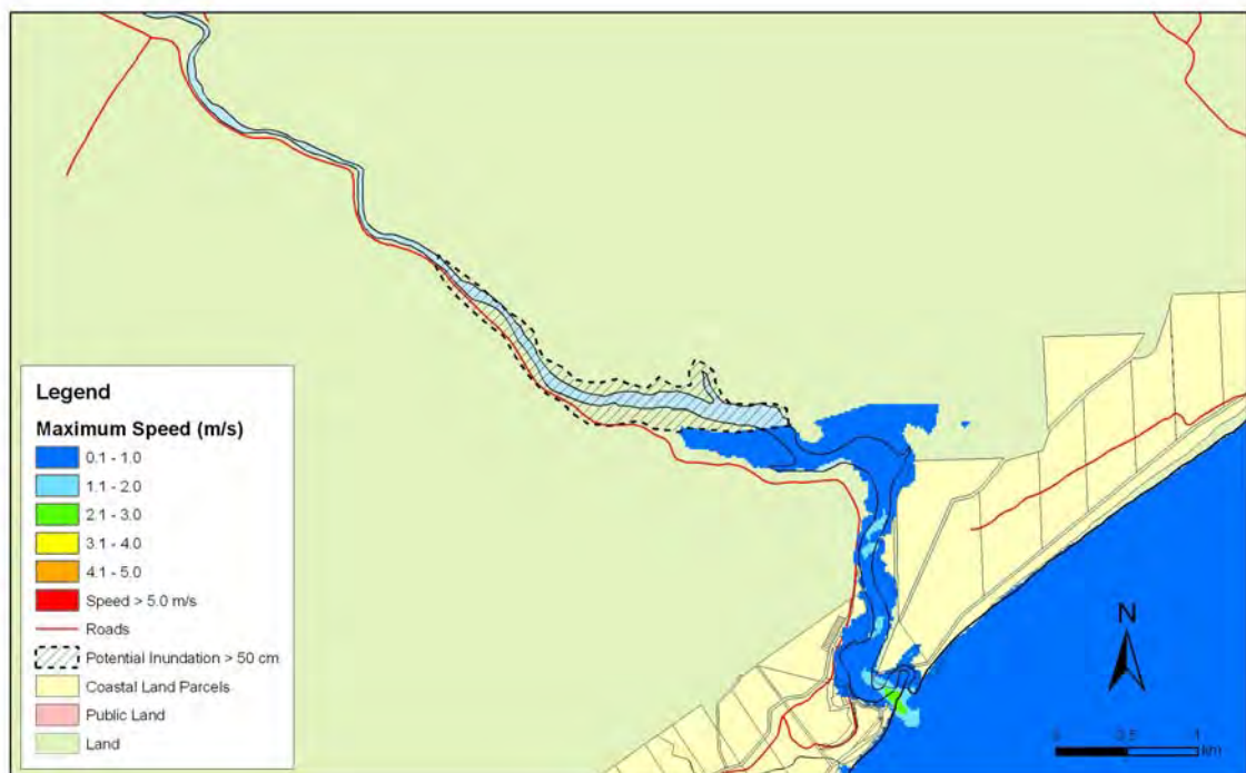
Figure 5.49: Toko Mouth – 1:100 year remote tsunami: Maximum water depth for inundated land (top) and maximum speed (bottom) for MHWS
