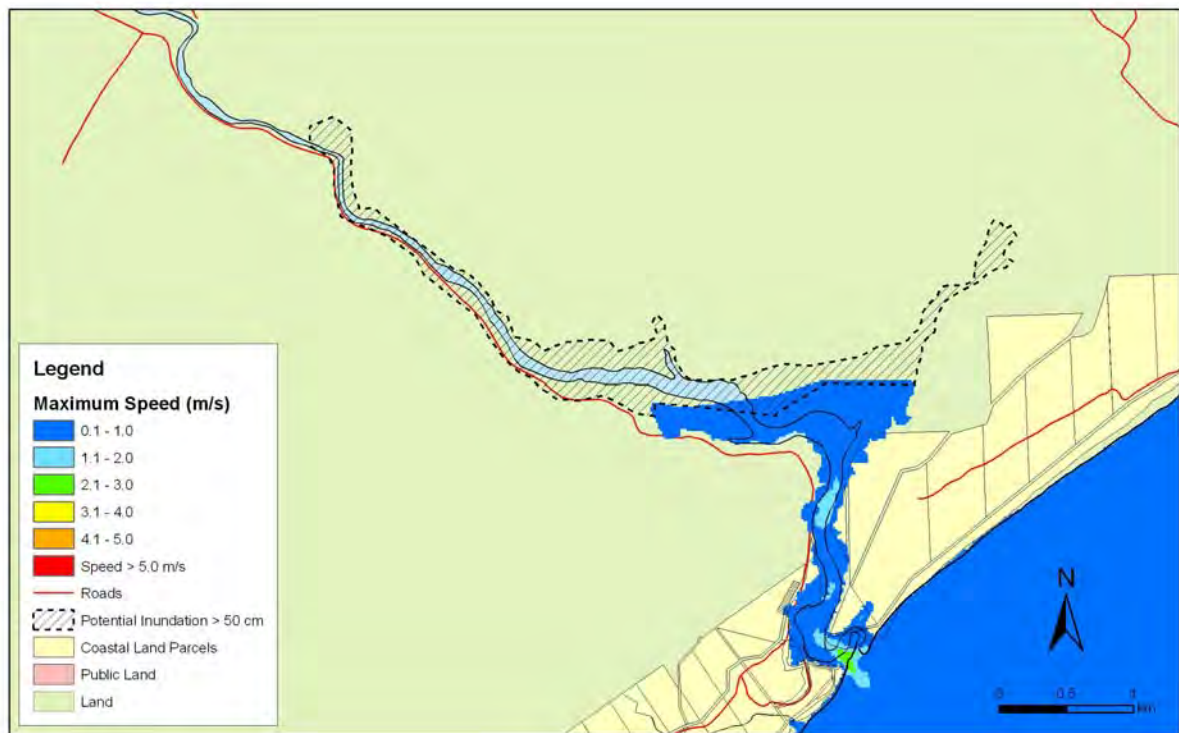
Figure 5.50: Toko Mouth– 1:100 year remote tsunami: Maximum water depth for inundated land (top) and maximum speed (bottom) for MHWS with a sea level rise of 30 cm.
