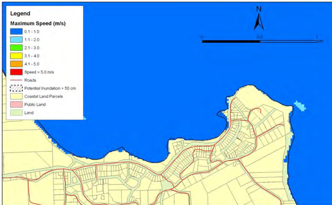
Figure 5.130: Moeraki – 1:100 year remote tsunami: Maximum water depth for inundated land (top) and maximum speed (bottom) for MHWS.
