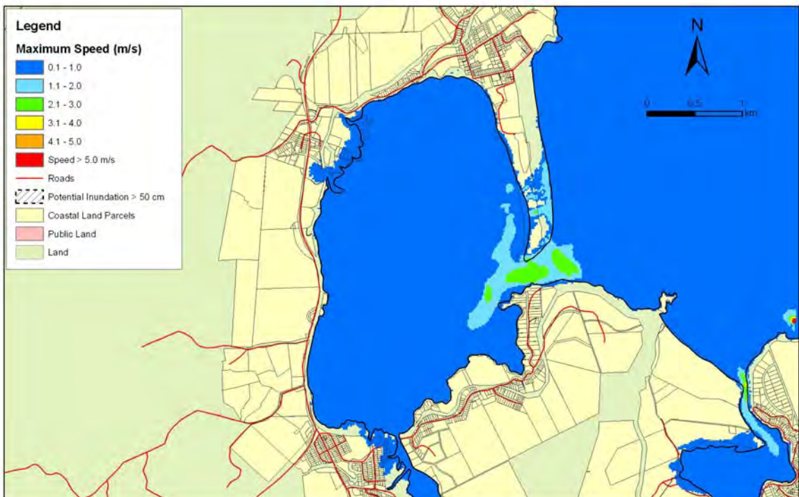
Figure 5.113: Warrington and Blueskin Bay – 1:100 year remote tsunami: Maximum water depth for inundated land (top) and maximum speed (bottom) for MHWS with a sea level rise of 30 cm.
