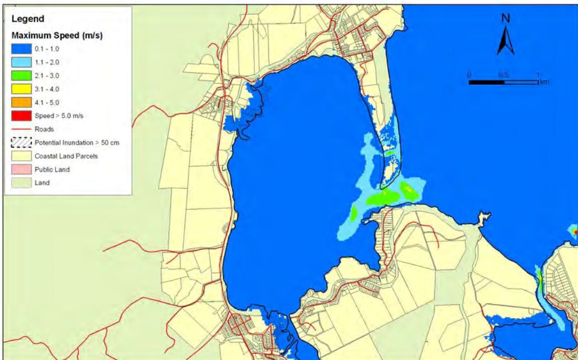
Figure 5.114: Warrington and Blueskin Bay – 1:100 year remote tsunami: Maximum water depth for inundated land (top) and maximum speed (bottom) for MHWS with a sea level rise of 50 cm..
