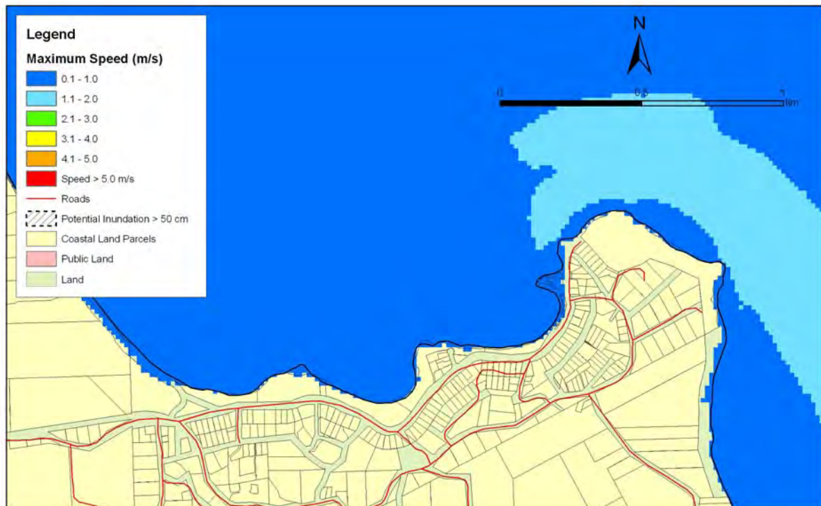
Figure 5.135: Moeraki – 1:500 year remote tsunami: Maximum water depth for inundated land (top) and maximum speed (bottom) for MHWS with a sea level rise of 50 cm.
