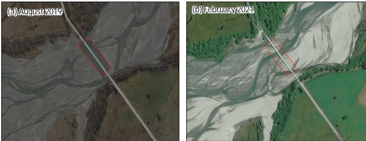
Figure 2.6: Aerial photos of riverbed in the vicinity of the Rees River Bridge showing (a) gravel extraction zone upstream and downstream of bridge in August 2019 (indicated by dashed, red box) and (b) same area in February 2021
