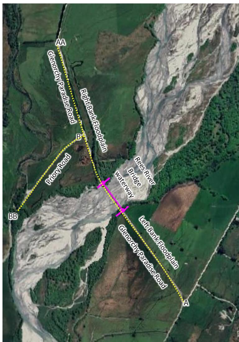
Figure B.4: Aerial photograph showing right bank floodplain, Rees River Bridge waterway and left bank floodplain locations and where flows listed in Table B.1 were extracted. Also shown are locations of long-section profiles A-AA shown on Figure B.5 and B-BB shown on Figure B.6.
