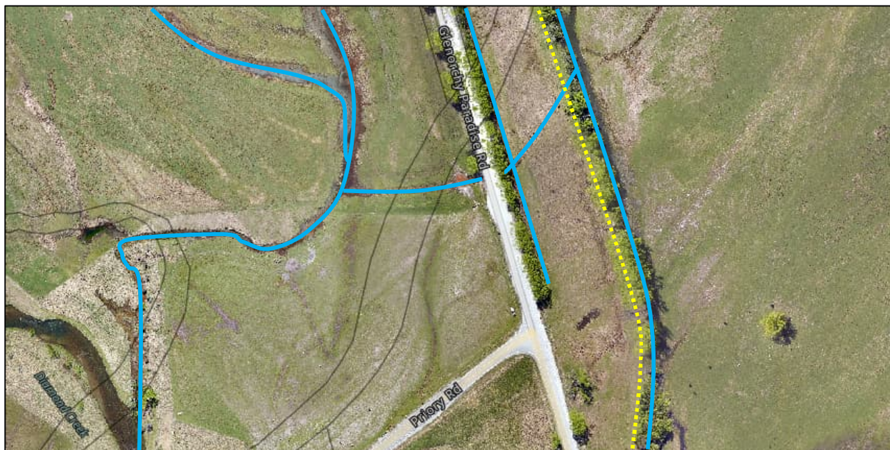
Figure 5.1: Example of existing drainage channels (marked with blue lines) running parallel with Glenorchy-Paradise and Priory Roads. Existing secondary floodbank marked with dashed, yellow line.
