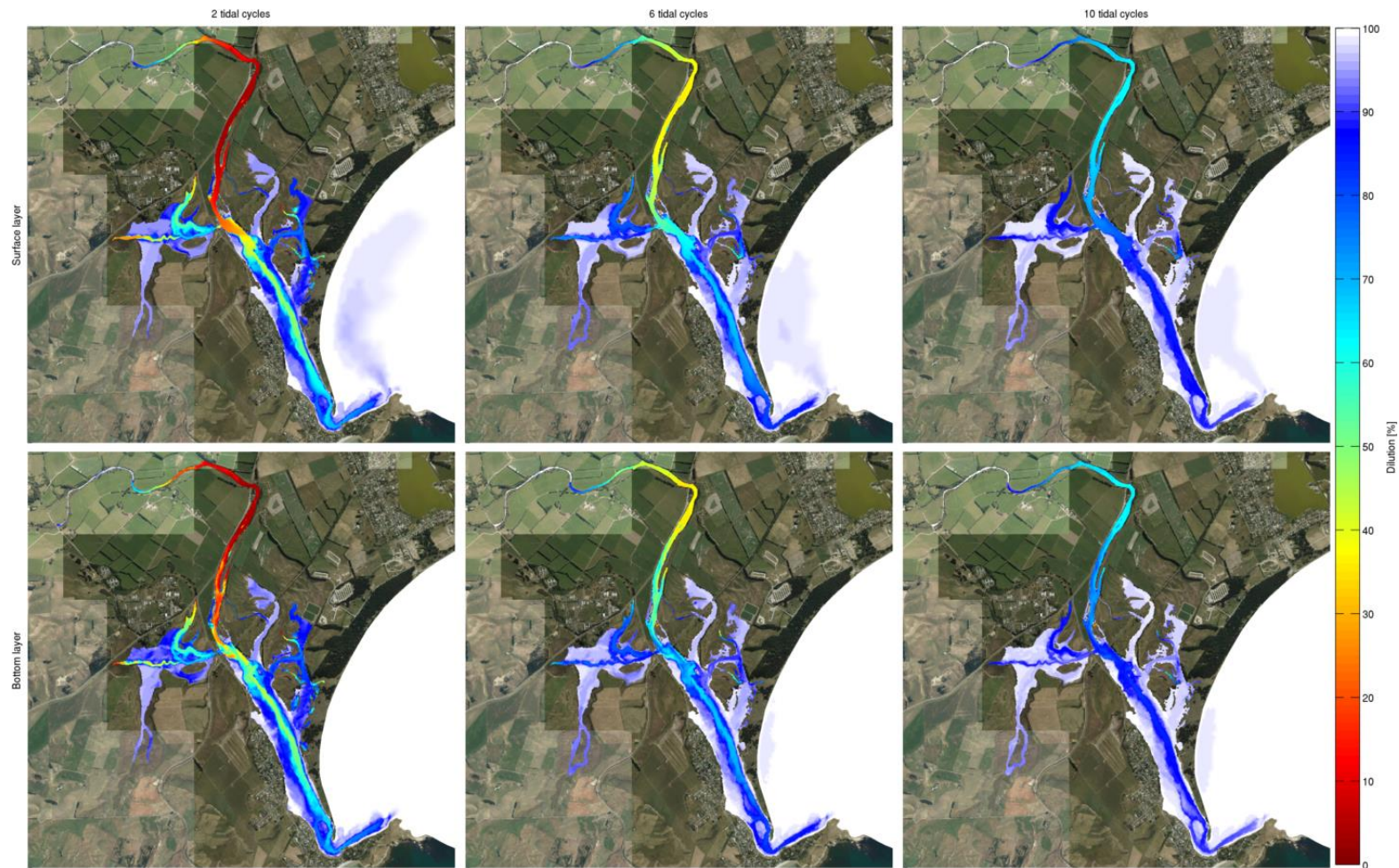
Figure 4.19 Dilution occurring at the surface (top) and bottom (bottom) of the estuary after 2 (left), 6 (middle) and 10 tidal cycles during a spring tide range. The scenario modelled here is a discrete release of pollutant from the river into the estuary.
