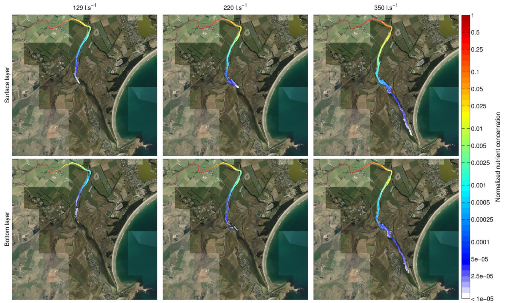
Figure 4.15 Relative (normalised) concentration of river nutrient after 24H of continuous release from Orbell's Crossing under the three flow states during spring tide. The release was started at the peak ebb tide.
