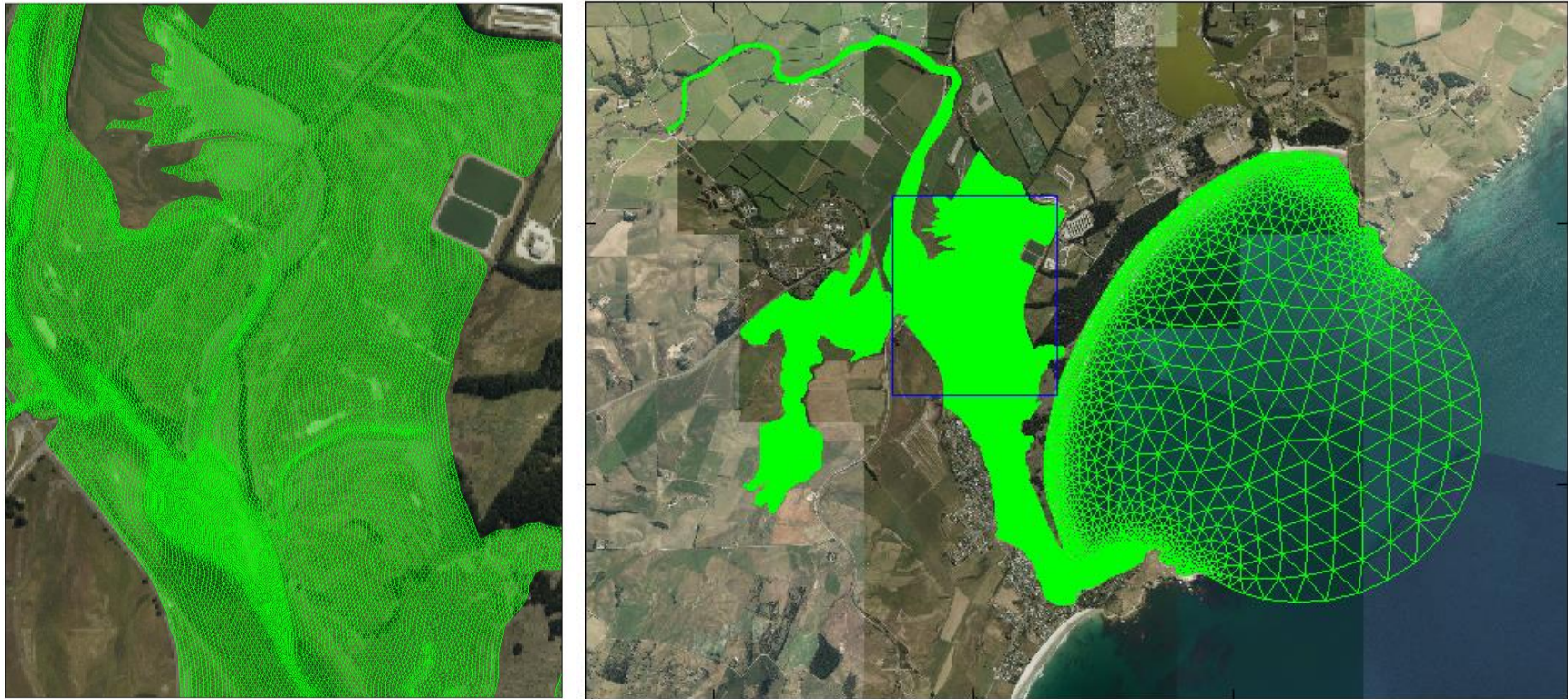
Figure 3.2 Triangular model mesh defined for the Waikouaiti Estuary. Right is the extent of the domain, and left is a zoom on the central part of the estuary.
