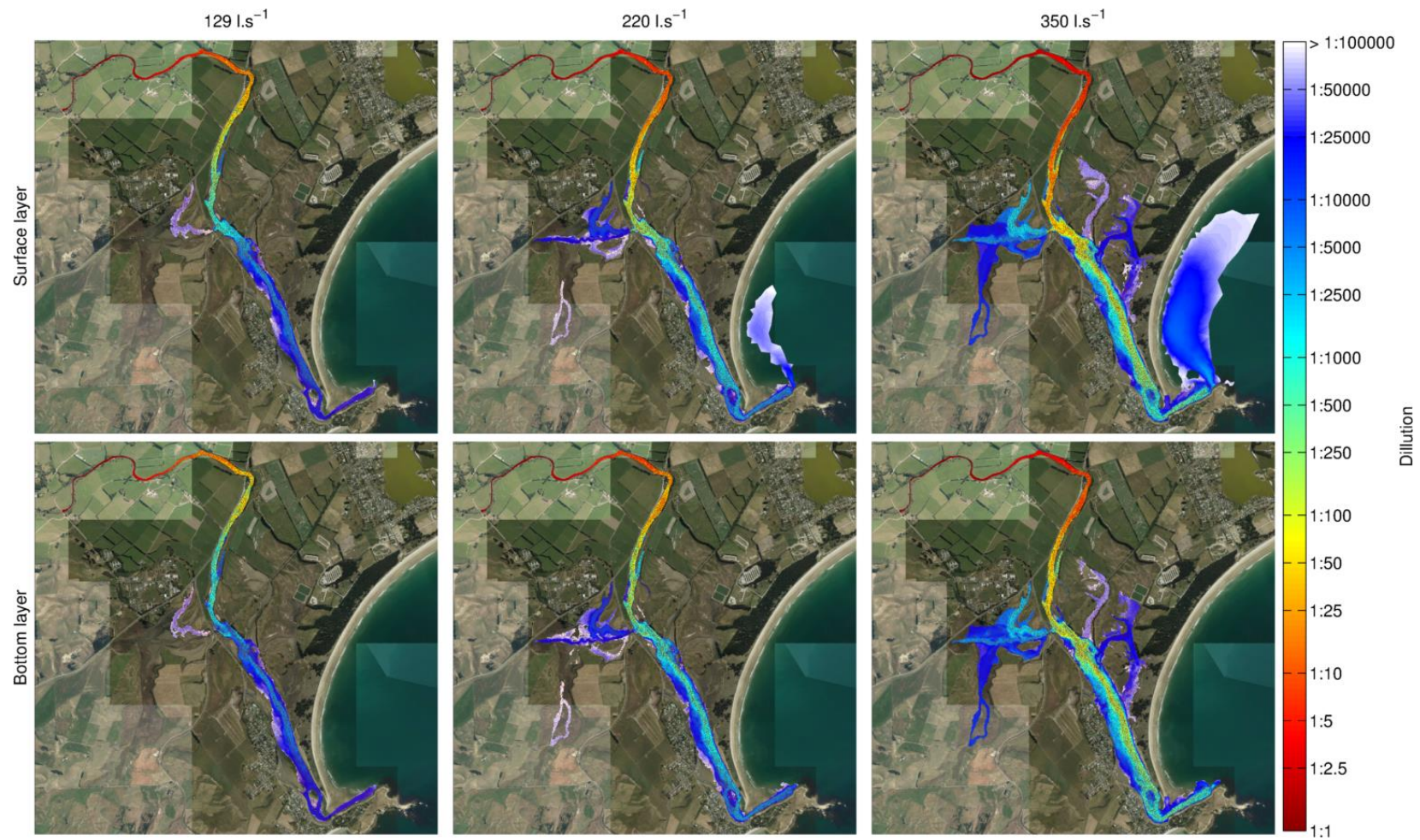
Figure 4.18 Dilution of river nutrient after 48H of continuous release Orbell's Crossing under the three flow states during spring tide. The release was started at the peak ebb tide.
