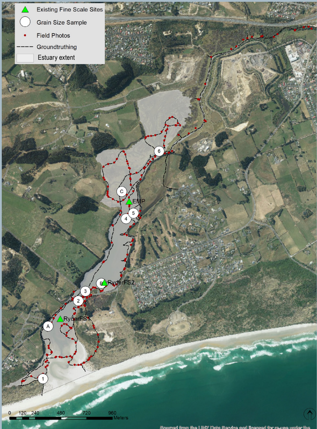
Figure 3. Kaikorai Estuary - mapped estuary extent showing ground-truthing coverage, field photos and location of fine scale sites and grain size samples used to validate substrate classifications.
