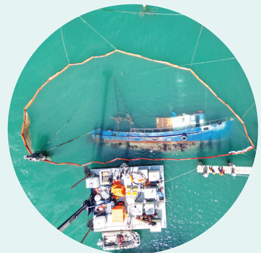
Above: ORC staff use containment booms and mechanical skimmers to clean up the oily water
