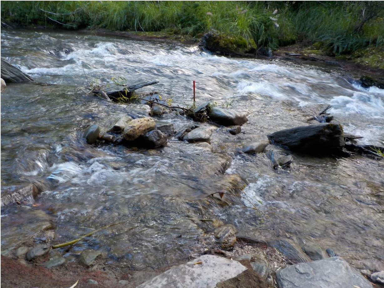
Figure 2: A temporary staff gauge with orange top to aid relocating the peg.
